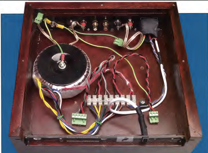
The new transformer mounted inside the same plinth as held the original two transformers. Again, ensure that any exposed mains wiring (for example, the IEC mains input socket) is properly covered, as shown here.
