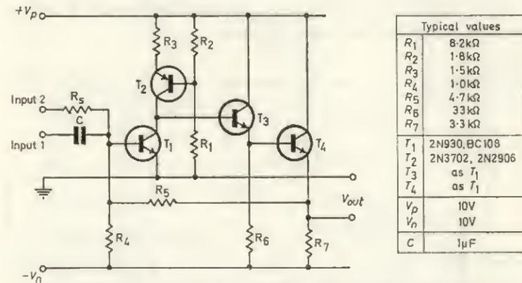
FIG. 12.2 Practical circuit for ultra-high gain amplifier
