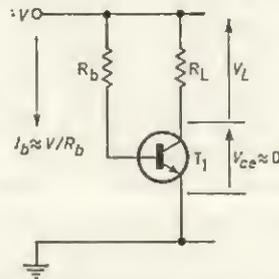
FIG. 3.1 Saturated transistor
