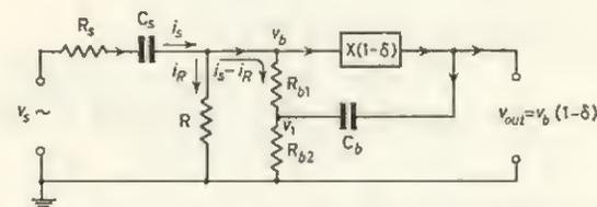
FIG. A6.1 Amplifier with bootstrap feedback
