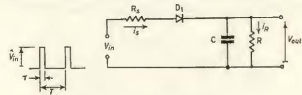
FIG. 1.4 Rectifier circuit
