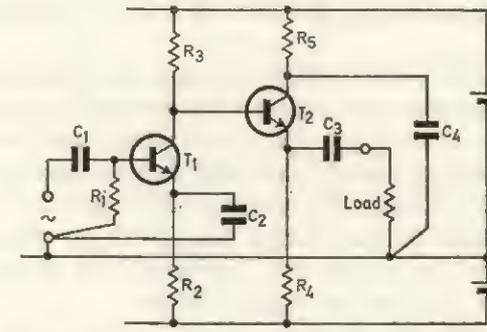
FIG. 16.9 Improved layout for simple amplifier circuit (Fig. 16.8)
