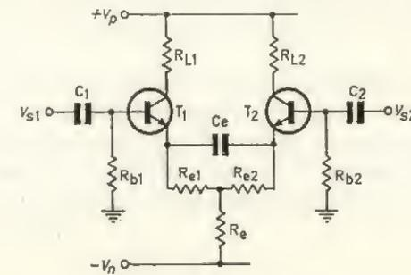
FIG. 4.12 Alternative bias circuit for emitter-coupled pair
