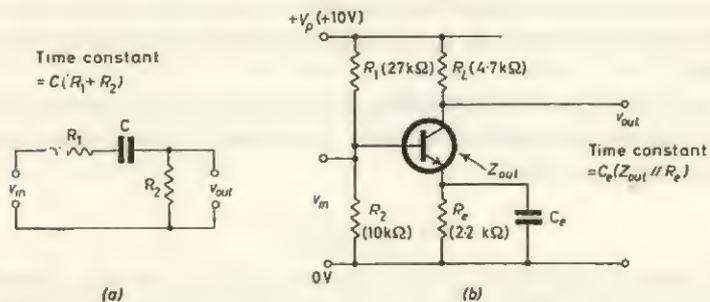
FIG. 8.2 Low-frequency time constants: (a) coupling, (b) decoupling
