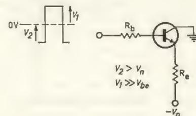
FIG. 3.6 Drive for saturation (circuit of Fig. 3.2)
