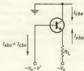
FIG. 3.4 Cut-off for circuit of Fig. 3.2
