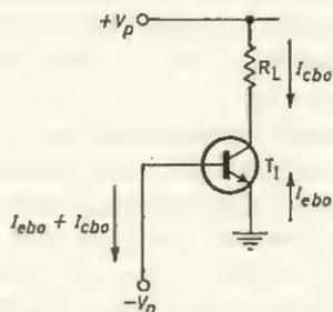
FIG. 3.3 Cut-off for circuit of Fig. 3.1
