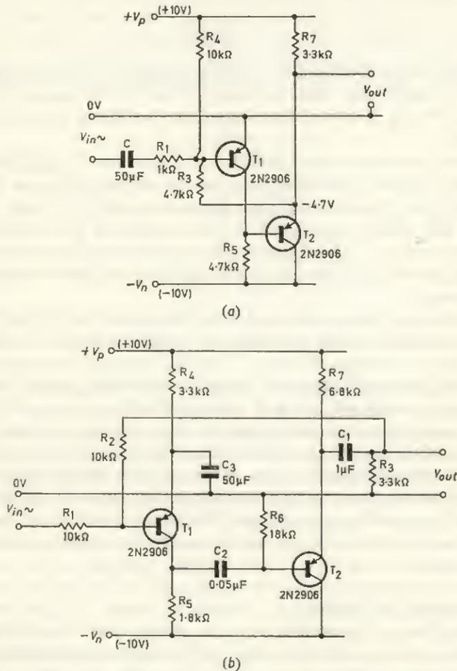
FIG. 8.3 Feedback amplifiers: (a) stable, (b) unstable
