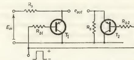
FIG. 9.18 Balancing  $V_{ce(sat.)}$
