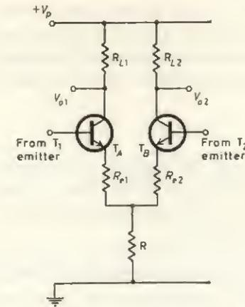
FIG. 11.9 Reduction of gain by extra emitter resistance, leading to poor rejection ratio
