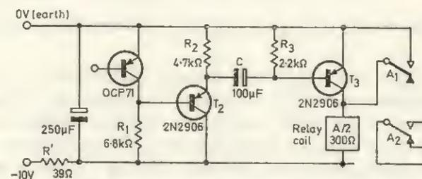
FIG. 16.3 Alternative method to improve light relay
