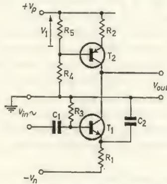
FIG. 12.1 Basic idea for ultra-high gain amplifier
