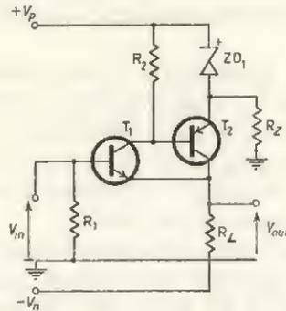
FIG. 10.7 Modified form of Fig. 10.6 for high-temperature operation
