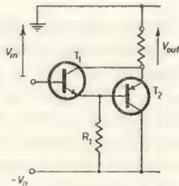
FIG. 10.8 Power-drive circuit
