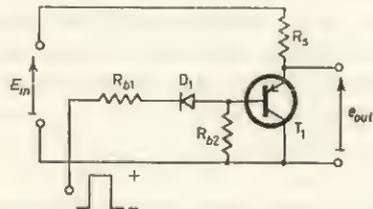
FIG. 9.17 Circuit to reduce effect of  $I_{ebo}$
