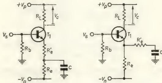
FIG. 4.8 Addition of  $R_e'$  to stabilize gain
