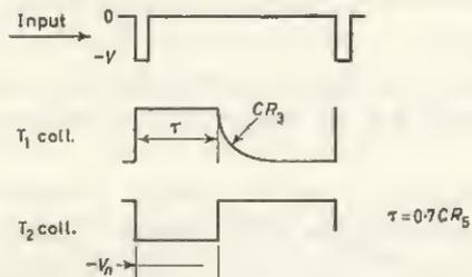
FIG. 3.14 Waveforms for one-shot multivibrator (Fig. 3.13)
