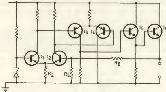
FIG. 9.11 Extra stages for higher loop gain
