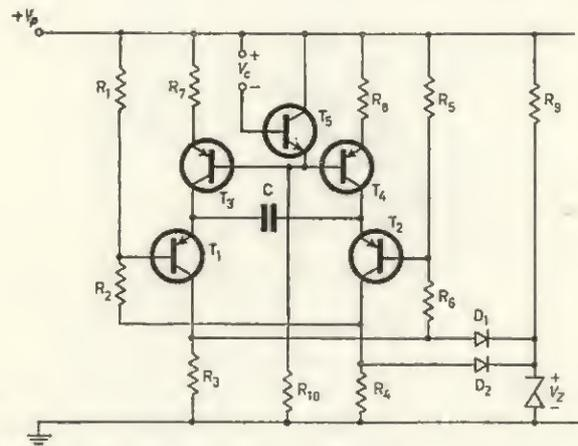
FIG. 11.5 Use of extra transistor for  $V_{EB}$  compensation
