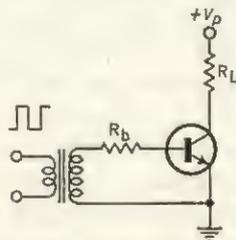
FIG. 3.9 Transformer-coupled drive
