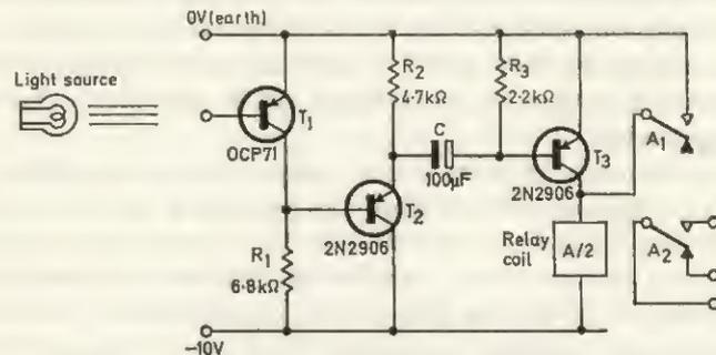
FIG. 16.1 Pulse-operated light relay
