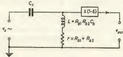
FIG. A6.3 Equivalent circuit of amplifier with bootstrap feedback (Fig. A6.1) for approximate analysis near response peak
