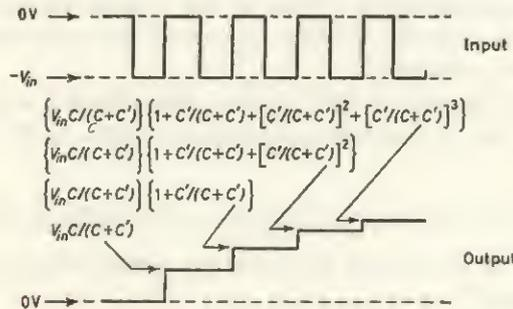
FIG. 13.2 Waveforms for diode pump staircase generator (Fig. 13.1)
