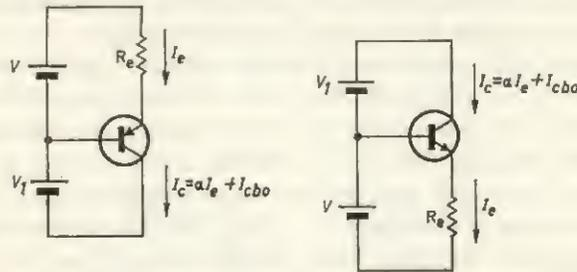
FIG. 2.4 Transistor currents
