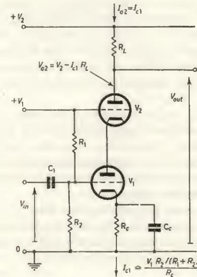
FIG. 14.1 Valve cascode
