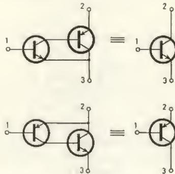
FIG. 10.10 Equivalence of complementary circuits to single transistors
