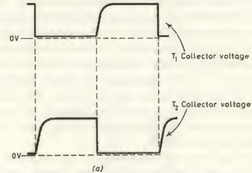
FIG. 10.3 (a) Waveforms for conventional two-state circuit (Fig. 10.1)
