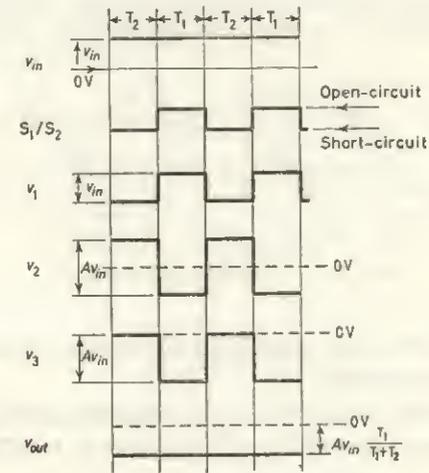
FIG. 9.14 Waveforms for chopper amplifier block diagram (Fig. 9.13)
