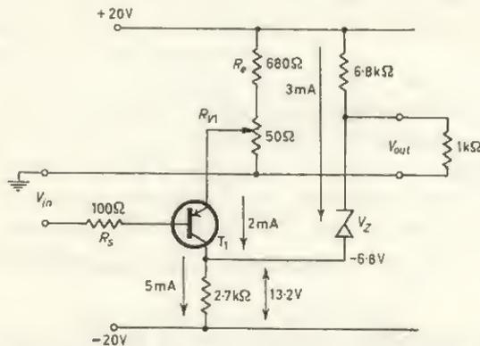
FIG. 9.2 Practical form of simple direct-coupled amplifier (Fig. 9.1)
