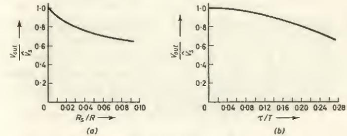
FIG. 1.9  $V_{out}$  for sine-wave input in terms of (a)  $R_s/R$  and (b)  $\tau/T$
