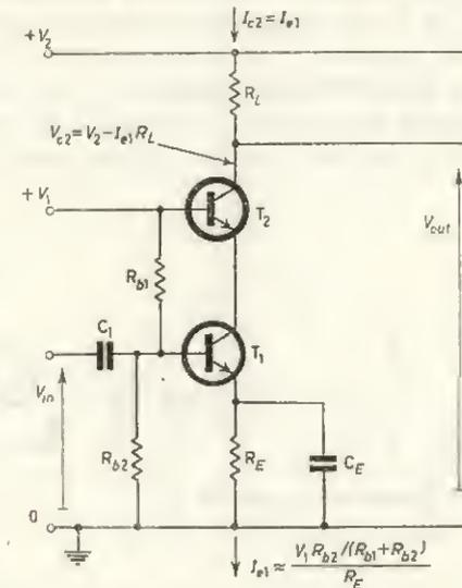
FIG. 14.2 Transistor cascode
