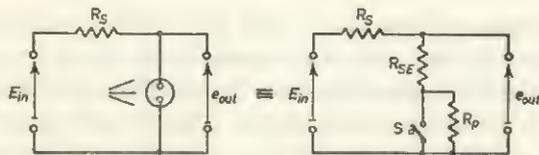
FIG. 9.20 Photoconductive cell used as a chopper
