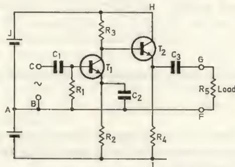
FIG. 16.8 Simple amplifier circuit
