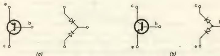
FIG. 2.1 (a)  $p-n-p$  transistor, (b)  $n-p-n$  transistor
