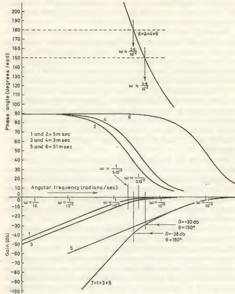
FIG. 8.6 (a) Stabilized version of Fig. 8.5 (second method)
