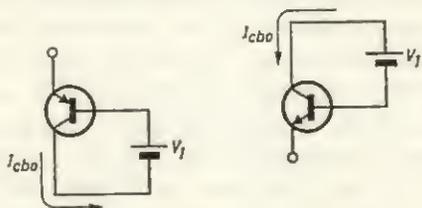
FIG. 2.3 Collector leakage
