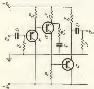
FIG. 7.7 Amplifier with input and output buffer stages
