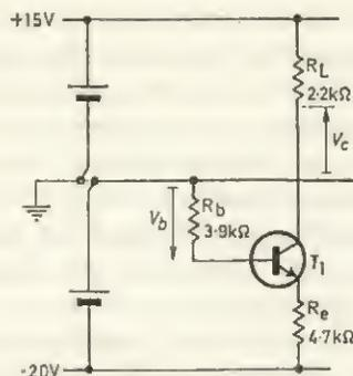
FIG. 2.6 Practical example of bias circuit
