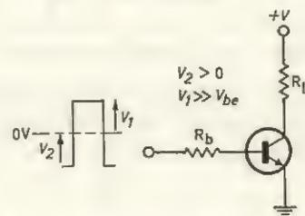
FIG. 3.5 Drive for saturation (circuit of Fig. 3.1)
