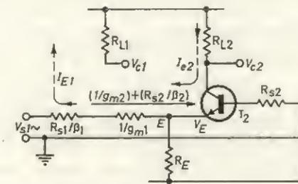
FIG. 4.10 Equivalent circuit for  $v_{S2} = 0$
