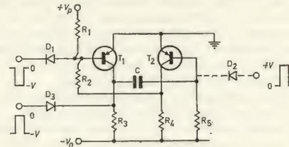
FIG. 3.16 Alternative trigger
