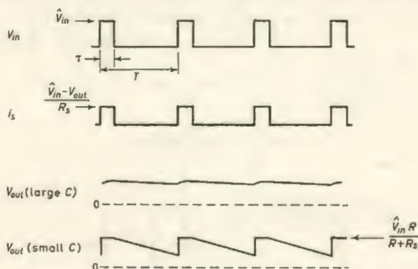
FIG. 1.6 Waveforms for rectifier circuit (Fig. 1.4)
