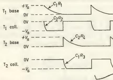
FIG. 3.12 Waveforms for free-running multivibrator (Fig. 3.11)
