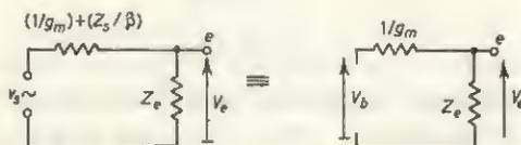
FIG. 4.6 Alternative forms of Fig. 4.5 give identical results
