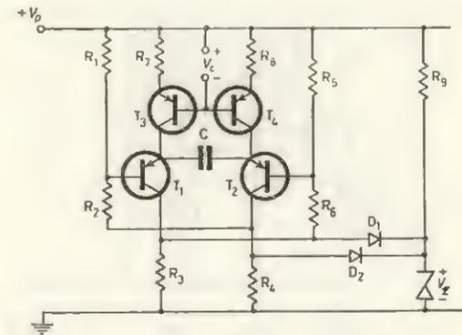
FIG. 11.4 Voltage-controlled oscillator
