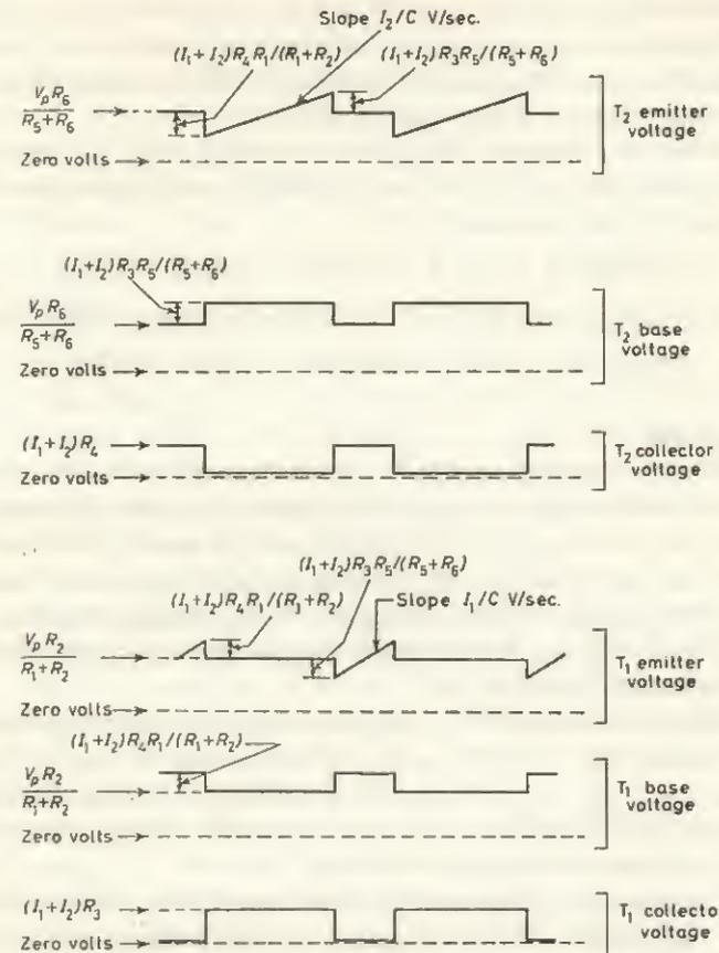
FIG. 11.2 Waveforms for circuit of emitter-coupled multivibrator (Fig. 11.1). Magnitudes are approximate and assume  $R_3 \ll (R_5 + R_6)$ ,  $R_4 \ll (R_1 + R_2)$
