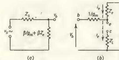
FIG. 4.7 (a) Input, and (b) output equivalent circuits
