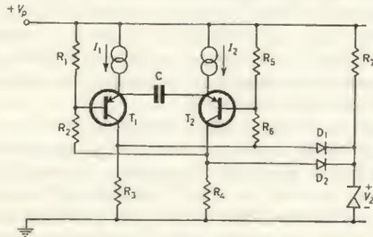
FIG. 11.3 Clipping circuit
