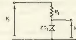
FIG. 1.13 Simple Zener diode stabilizer
