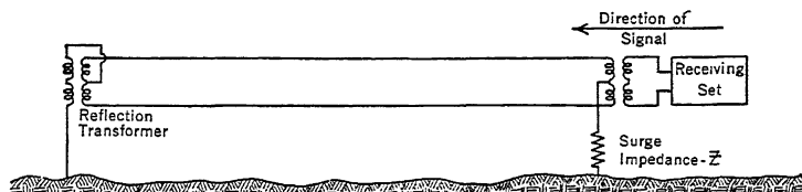
FIG. 24. Schematic of Wave Antenna. (The length may be as much as a mile, the height about 25 feet.)
