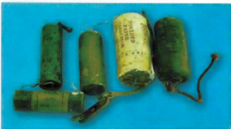
These old paper capacitors have obviously seen better days and have been replaced. If you want to maintain authenticity, you can often use the "shell" of an old capacitor to hide a modern replacement.
