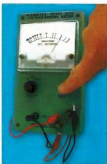
A high-voltage insulation tester is useful for checking capacitors out of circuit.
