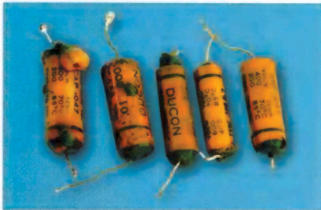
Capacitors that are deformed should be replaced. However, if a capacitor appears OK, it may still be used in many circuit locations even if it is leaky.
