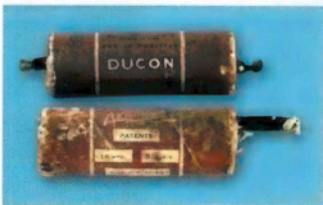
This photo shows a couple of old Ducon paper capacitors. They were notoriously unreliable.
