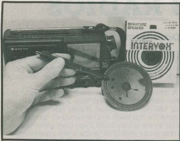
Figure 2. Check the speaker for holes, tears, or a frozen or rubbing voice coil. To check for frozen or rubbing coil, gently move the coil with a thumb or finger on each side of the middle.
