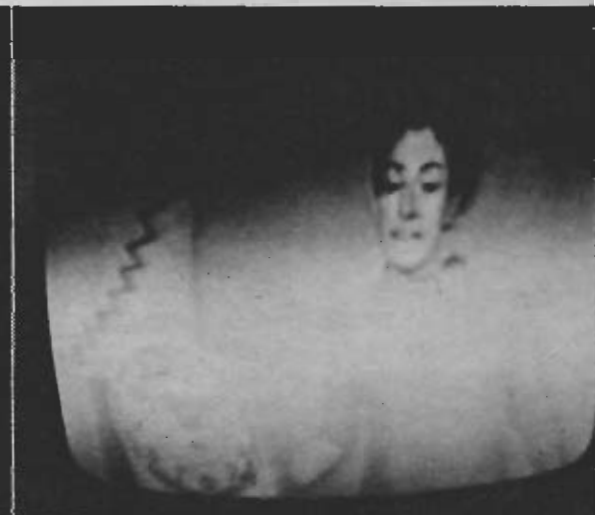
Fig. 6—Banding is across screen for filter short in vertical output (up and down if in horizontal).
