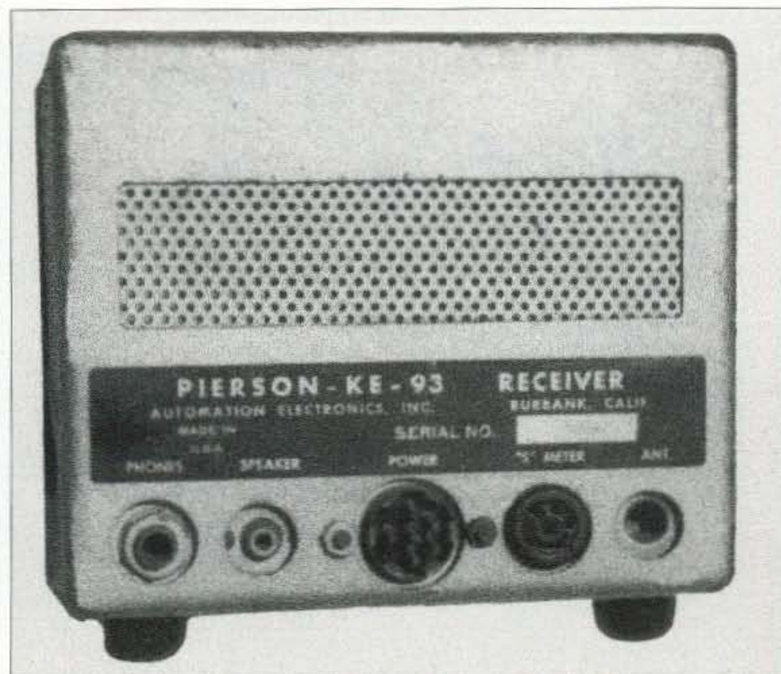
Photo B. Rear cabinet view of the receiver showing the connectors.
