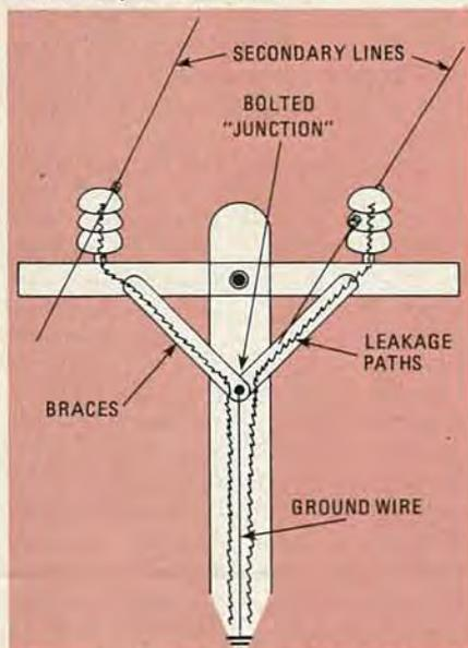
FIG. 2—LEAKAGE PATHS develop on line-pole hardware and generate RFI.
