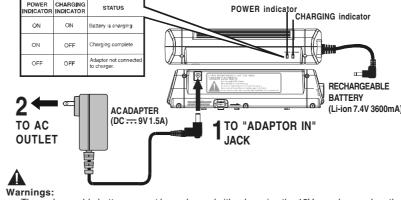
. The rechargeable battery cannot be recharged either by using the 12V car-plug or when the Caution:
