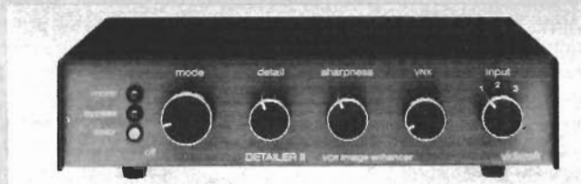
FIG. 5—SIGNAL ENHANCERS, such as the Detailer II from Vidcraft improve the apparent sharpness and resolution of either off-the-air recordings or tape copies.
