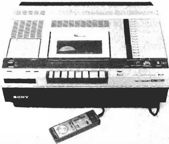
FIG. 12—SONY's SL-5800 uses a double-azimuth head to provide noise-free slow and freeze motion.
