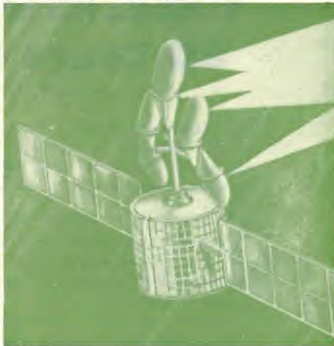
An advanced antenna system for direct broadcast of TV programs from an orbiting satellite to home receivers is being designed today for NASA by Sylvania. By concentrating programming to small areas of the earth and transmitting about 100 times the power of present satellites, the antenna system will provide signals strong enough for reception by modified home equipment. A two-foot diameter antenna and small converter, like the early u.h.f. TV converters, will be required.
