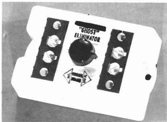
FIG. 4—GHOST ELIMINATOR is inserted in antenna lead-in and adjusted for best picture.
