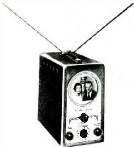
The Tele-Tone has rotatable V antenna.
