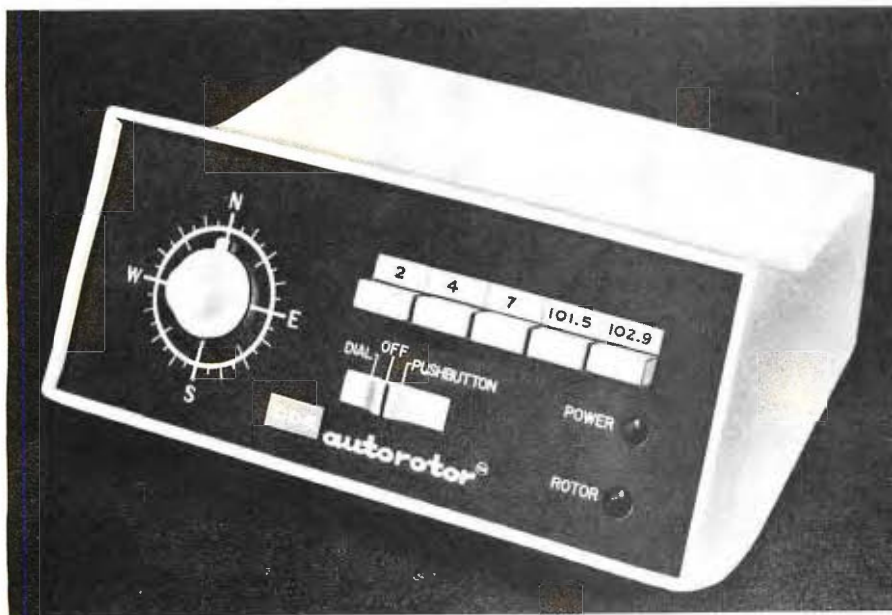
Cornell-Dubilier's AR-33 permits preprogramming for special channels. Unit is all electronic.
