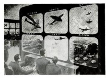
The radio-television controlled plane (shown at right) sends the television impulses down to Earth, where observers before six screens, pictured above, can look into six directions at once. As the plane has no crew it is wholly directed by radio. Wherever it may be, the distant ground radio observers and operators can follow the plane visually at all times. It can be destroyed in flight so it will not fall into the hands of the enemy, should such a decision become necessary.
