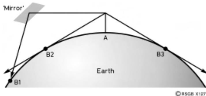
**Figure 2** Reception of A's signals at B1 using the *sky wave*
