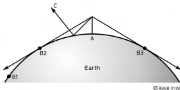
**Figure 1** Stations between B2 and B3 receive the *ground wave*
