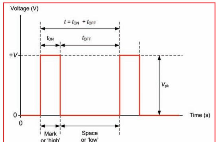
Fig.1.6. A pulse waveform showing 'on' and 'off' times
