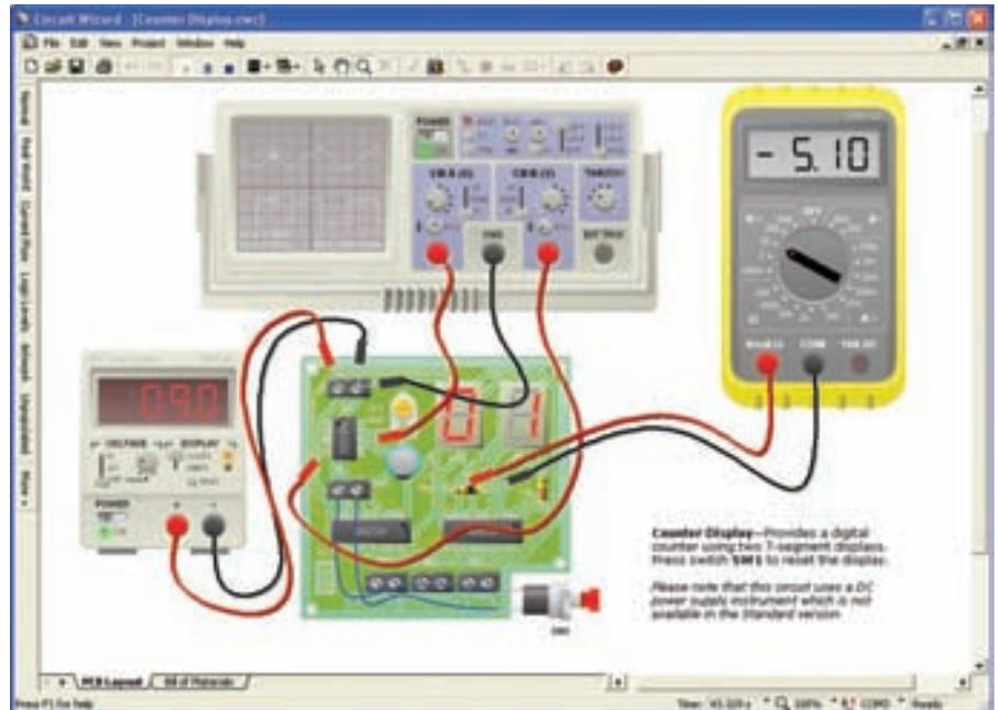
Fig.1.14. Circuit Wizard screenshot showing the use of 'virtual instruments'
