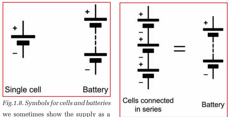
Fig.1.8. Symbols for cells and batteries
