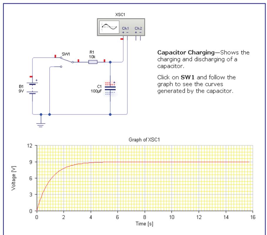
Fig.1.15. A capacitor charging circuit showing charge building up on the plates, voltage levels and a graphical plot of voltage against time
