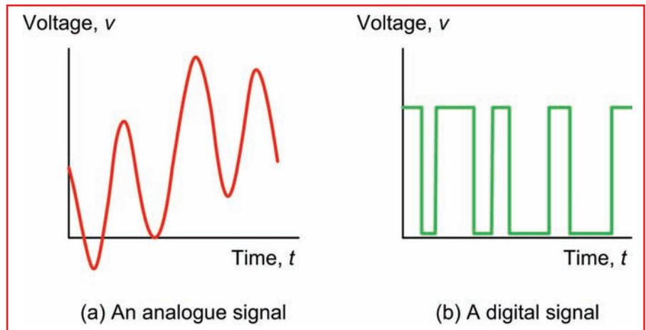
Fig.1.1. Typical analogue and digital signals
