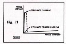
It is possible for a thyristor to be falsely triggered by a voltage well below the maximum rated voltage, if the voltage is applied rapidly enough, perhaps as a spike on the supply. There is a maximum dv/dt rating (rate of change of voltage) that a thyristor can withstand without falsely triggering, possibly in a damaging fashion. Too rapid a rise of voltage on the anode will trigger the device because self capacitance will cause a trigger current to flow.
