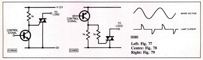
cause enough gate current to flow to destroy the gate structure of the triac and the transistor. On the other hand, a triggering circuit such as that shown in Fig. 78 will not be damaged by occasional spurious triggering.
