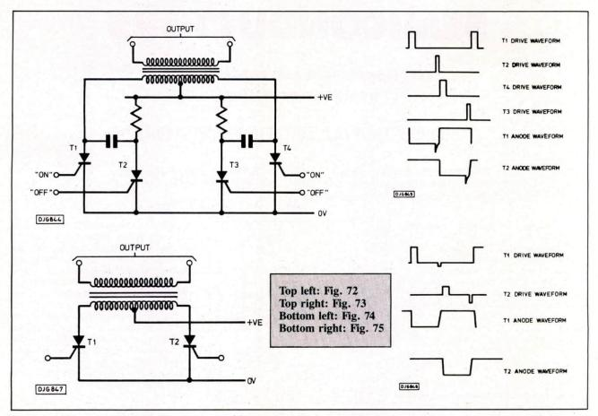
tion thyristor. The drive waveforms are illustrated in Fig. 73.
