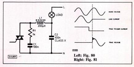
Choose the capacitor value so that the resonant frequency of the snubber capacitor with the load inductance is in the range 1000 to 10,000 Hz. Then calculate a resistor value to bring the Q of the resonant circuit of the snubber capacitor and the load inductance to 1, and then choose nearest preferred value.
