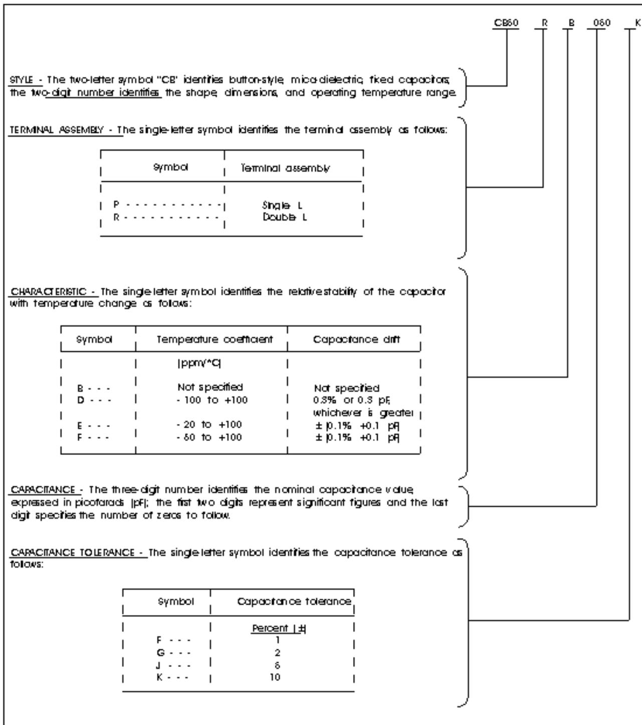
Table 1-2 shows how the part number on the CMR style of capacitor is broken down
