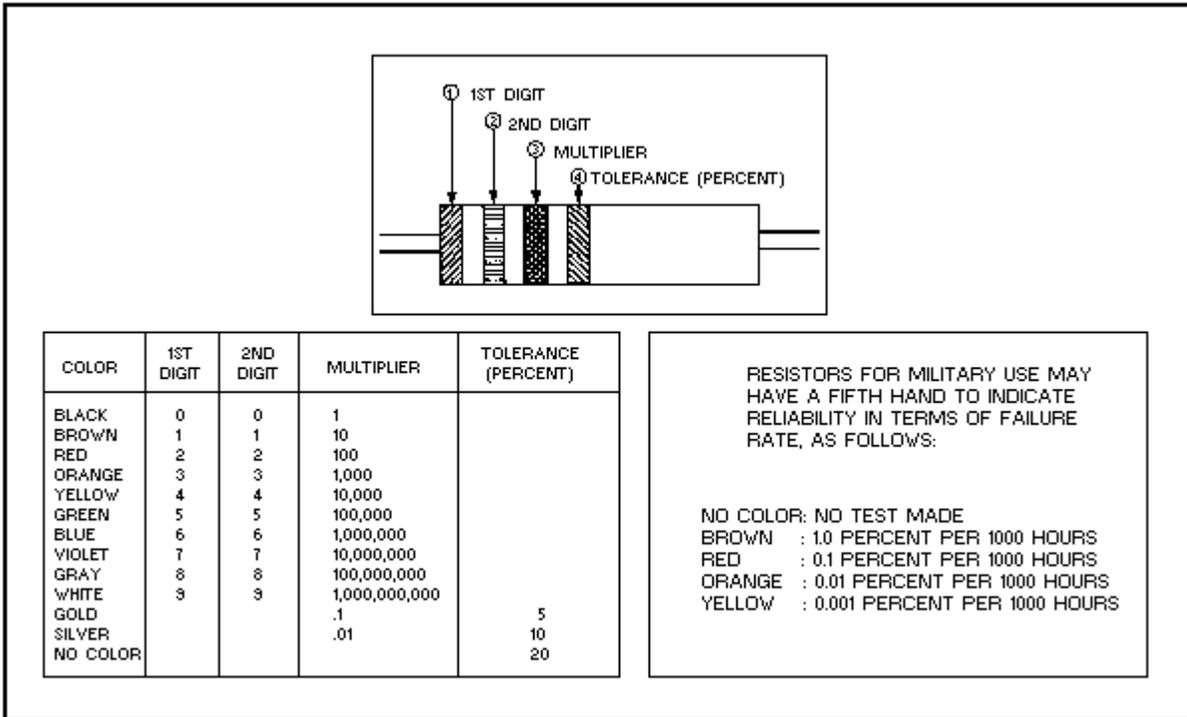
Figure 1-18.—Resistor color code.
