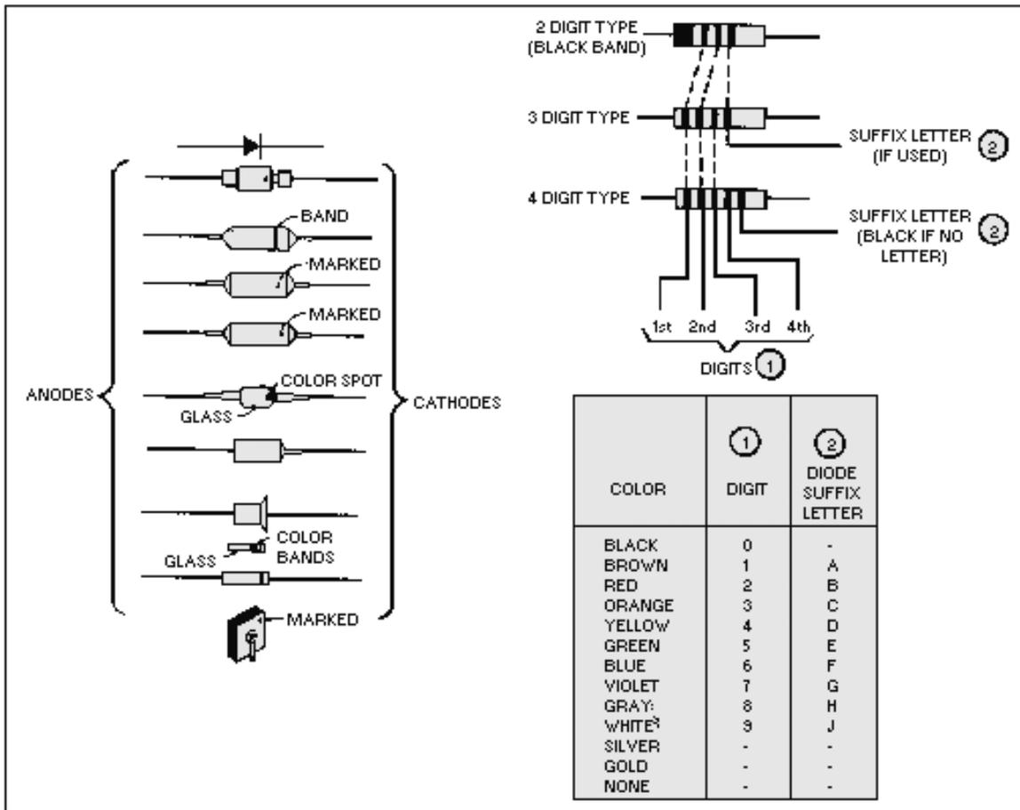
Figure 1-20.—Semiconductor diode markings and color code system.
