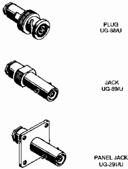
Figure 1-25.—Typical BNC connectors.
