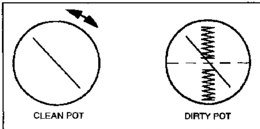
Figure 1-45.—Potentiometer noise check.
