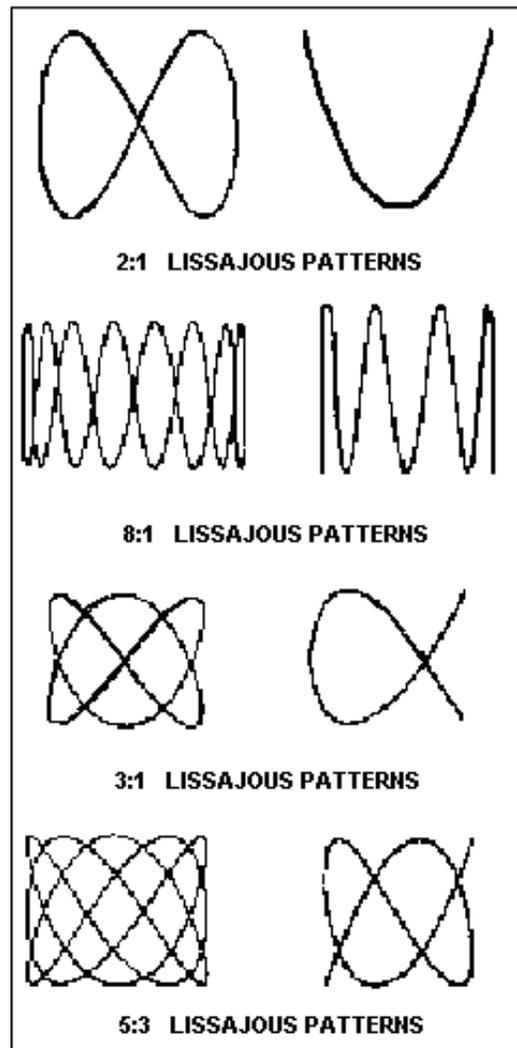
Figure 1-39.—Lissajous patterns of different frequency ratios.
