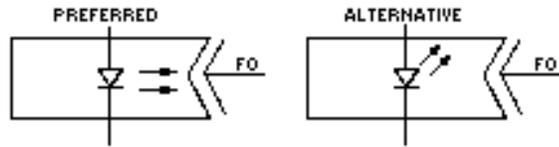
PLUG-WITH OPTICAL SOURCE. FOR OPTICAL DETECTORS REVERSE DIRECTION OF ARROWS.
