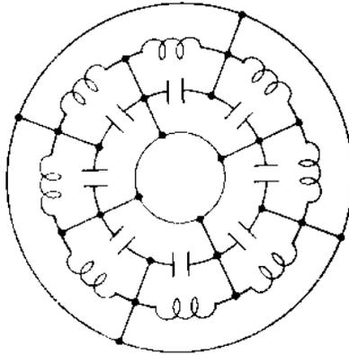
Figure 2-31.—Cavities in parallel because of strapping.
