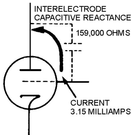
Figure 2-1A.—Interelectrode capacitance in a vacuum tube. 1 MEGAHERTZ.
