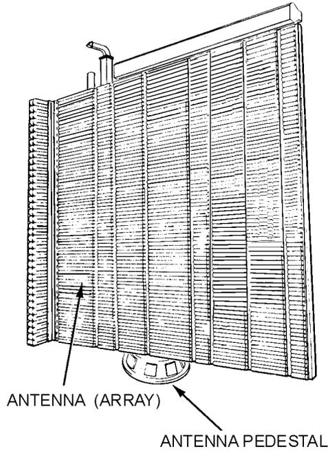
Figure 3-16.—Frequency-sensitive antenna.
