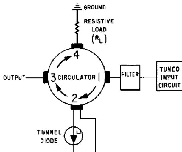
Figure 2-41.—Tunnel-diode amplifier.
