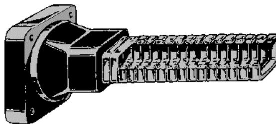
Figure 1-50.—Flexible waveguide.
