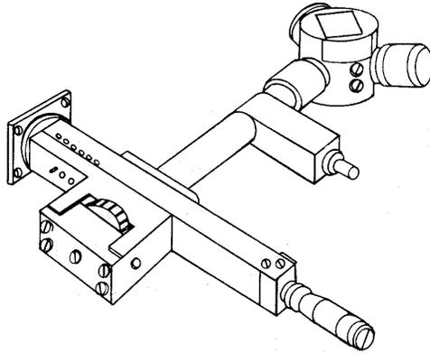
Figure 2-46.—Parametric amplifier.
