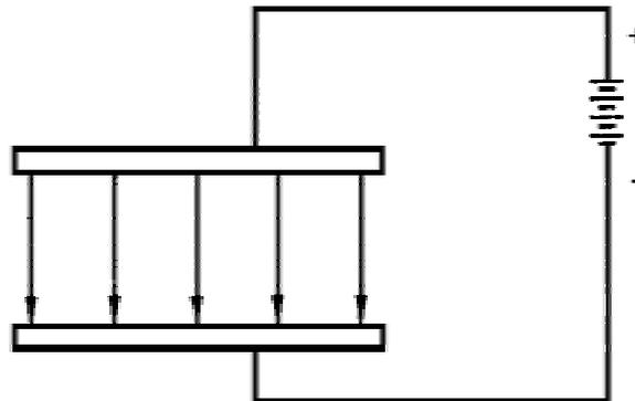
Figure 1-11A.—Simple electric fields. CAPACITOR.
