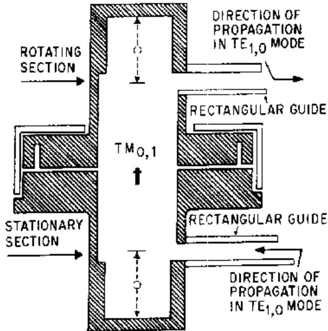
Figure 1-52.—Rotating joint.
