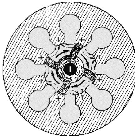
Figure 2-33.—Rotating space-charge wheel in an eight-cavity magnetron.
