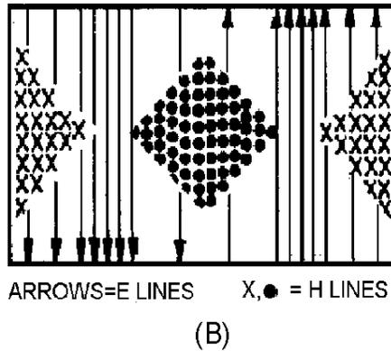
Figure 1-34B.—Waveguide operation in other than dominant mode.
