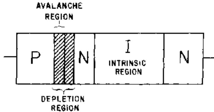
Figure 2-50.—Avalanche transit time for a pnin diode.
