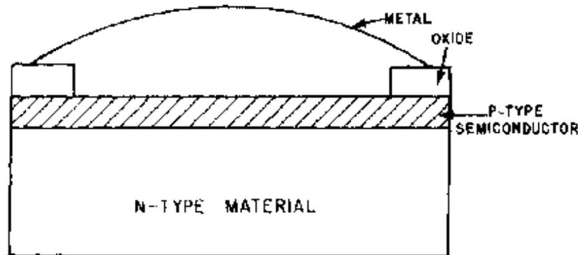
Figure 2-52.—Schottky-barrier diode.
