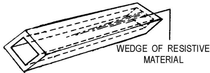
Figure 1-45C.—Terminating waveguides.
