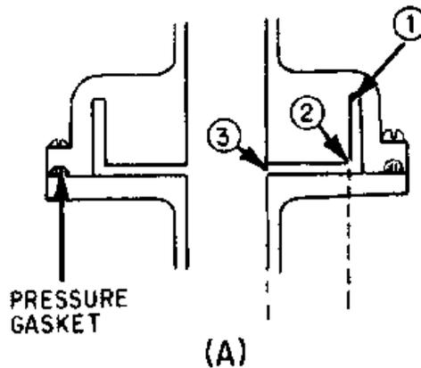
Figure 1-51A.—Choke joint.
