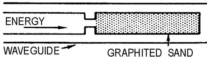
Figure 1-45A.—Terminating waveguides.
