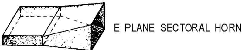
Figure 1-44A.—Waveguide horns. E PLANE SECTORAL HORN.
