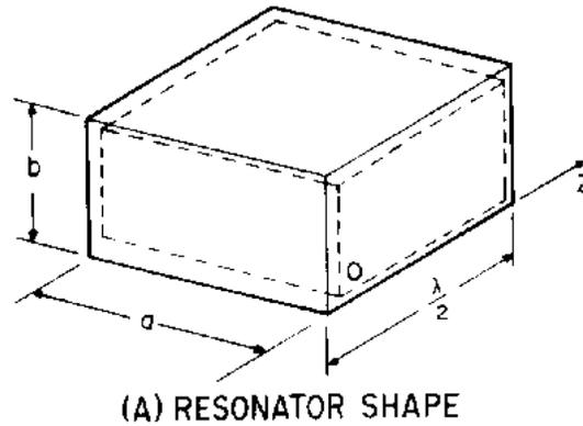
Figure 1-58A.—Rectangular waveguide cavity resonator. RESONATOR SHAPE.
