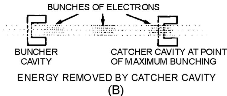
Figure 2-6B.—Removing energy from a velocity-modulated beam.
