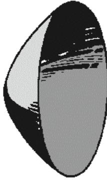
**LENS ANTENNAS** use a **COLLIMATING LENS** to force the spherical components of a wavefront into parallel (focused) paths by delaying or accelerating portions of the wavefronts, as shown in the illustration.
