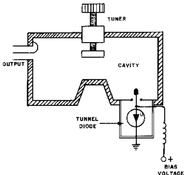
Figure 2-40.—Tunnel-diode oscillator.
