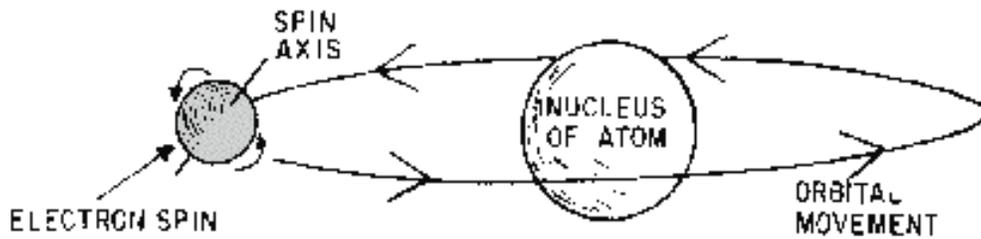
Figure 1-73.—Two types of electron movement.
