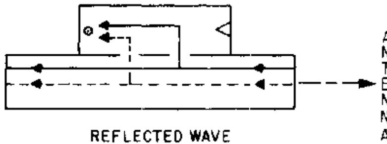
Figure 1-56.—Directional coupler designed to sample reflected energy.
