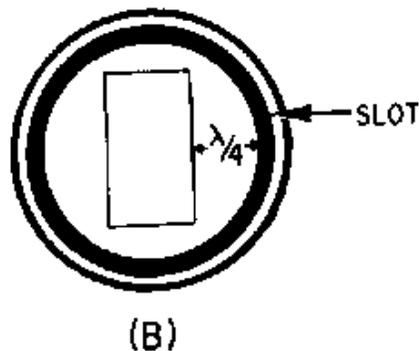
Figure 1-51B.—Choke joint.
