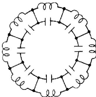
Figure 2-30.—Cavities connected in series.
