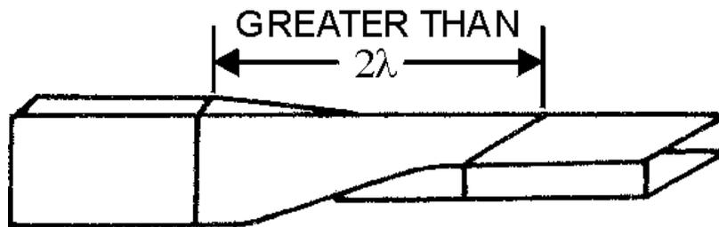
Figure 1-49.—Waveguide twist.
