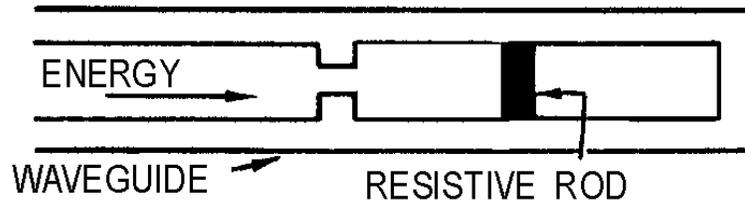
Figure 1-45B.—Terminating waveguides.
