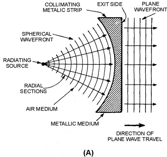
Figure 3-10A.—Waveguide lens.
