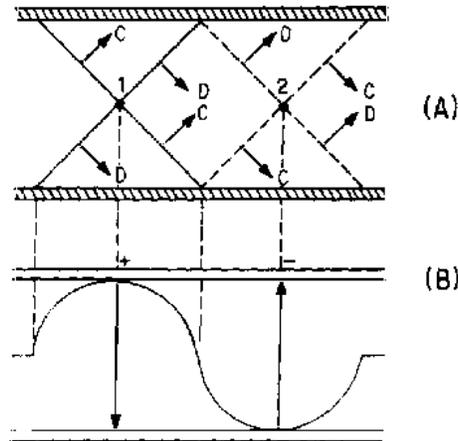
Figure 1-33.—Crisscrossing wavefronts and the resultant E field.
