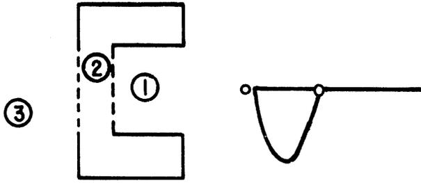
Figure 2-5C.—Buncher cavity action. ELECTRON #2 VELOCITY UNCHANGED.
