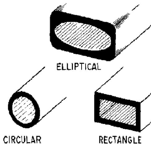
Figure 1-3.—Waveguide shapes.
