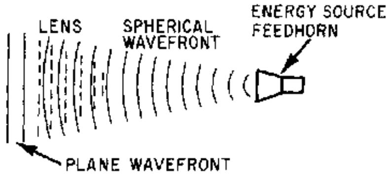
Figure 3-11.—Delay-type lens.
