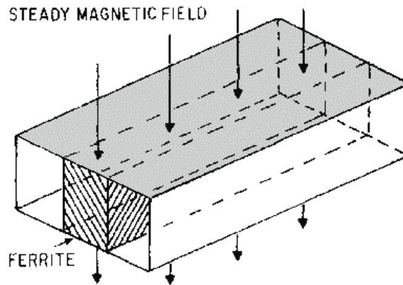
Figure 1-72.—Ferrite attenuator.
