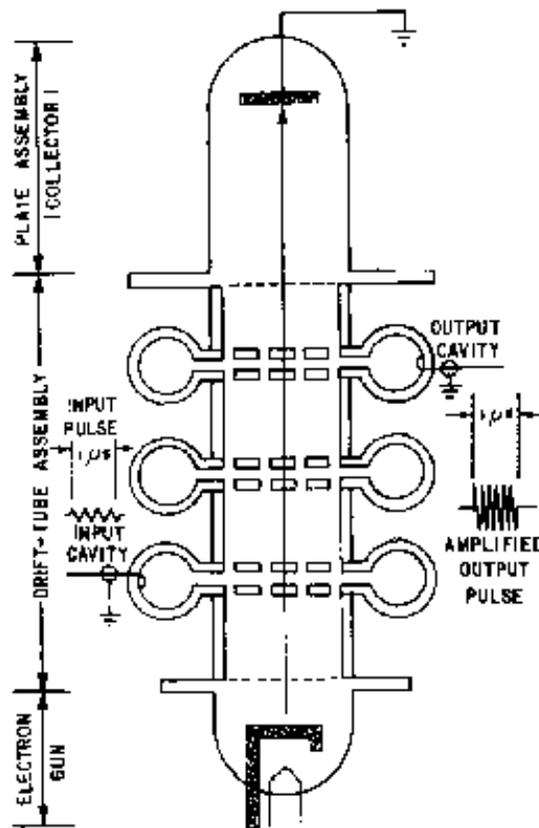
Figure 2-8.—Three-cavity klystron.
