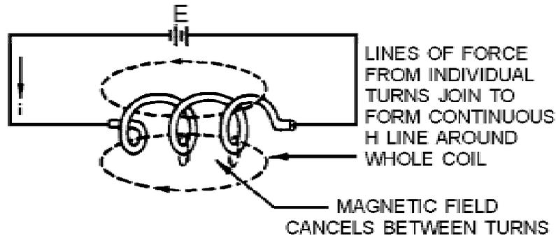
Figure 1-15.—Magnetic field on a coil.
