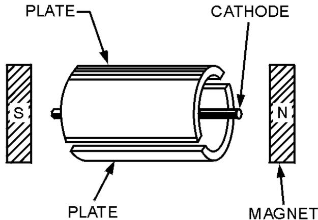
Figure 2-23A.—Split-anode magnetron.
