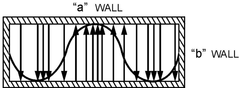
Figure 1-31.—One and one-half sine E field distribution.
