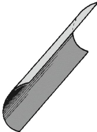
Figure 3-7.—Cylindrical paraboloid.
