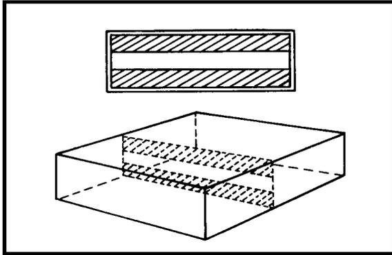
Figure 1B.—Waveguide iris.
