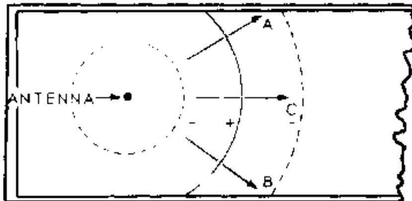
Figure 1-24.—Radiation from probe placed in a waveguide.
