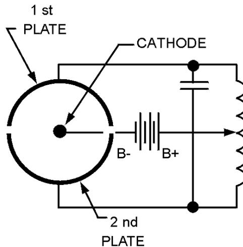
Figure 2-23B.—Split-anode magnetron.
