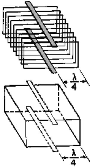
Figure 1-8.—Forming a waveguide by adding quarter-wave sections.
