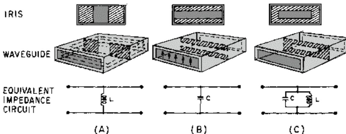
Figure 1-42.—Waveguide irises.
