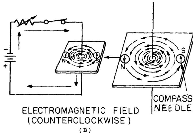
Arrows are generally used in electrical diagrams to indicate the direction of current in a wire. A cross (+) on the end of a cross-sectional view of a wire indicates that current is flowing away from you, while a dot (·) indicates that current is flowing toward you.
