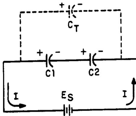
If an electrical circuit contains only two series connected capacitors,  $C_T$  may be computed using the following formula:
