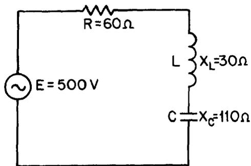
Figure 4-10.—Example circuit for determining power.
