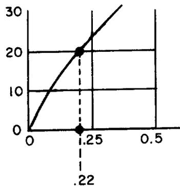
The value selected from the graph means that a capacitor (including the one you are solving for) will reach twenty percent of full charge in twenty-two one hundredths (.22) of one RC time constant. Remember that it takes  $100 \mu s$  for the capacitor to reach 20% of full charge. Since  $100 \mu s$  is equal to .22 RC (twenty-two one-hundredths), then the time required to reach one RC time constant must be equal to:
