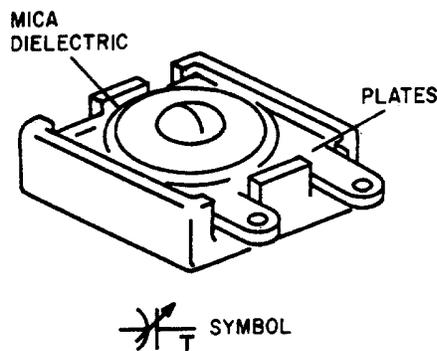
Figure 3-20.—Trimmer capacitor.
