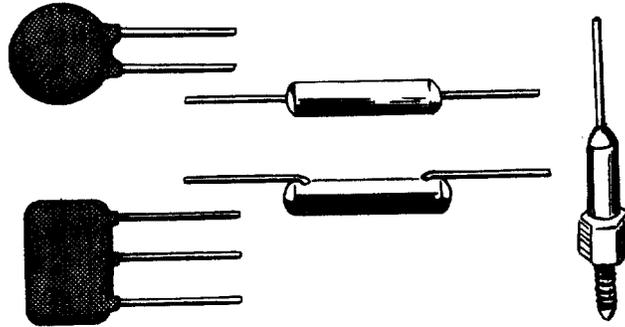
Figure 3-17.—Ceramic capacitors.
