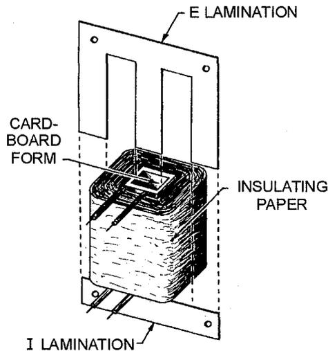
**EXCITING CURRENT**—When voltage is applied to the primary of a transformer, exciting current flows in the primary. The current causes a magnetic field to be set up around both the primary and the secondary windings. The moving flux causes a voltage to be induced into the secondary winding, countering the effects of the counter emf in the primary.
