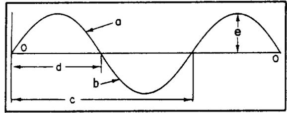
Figure 1C.—Components of a sinewave.
