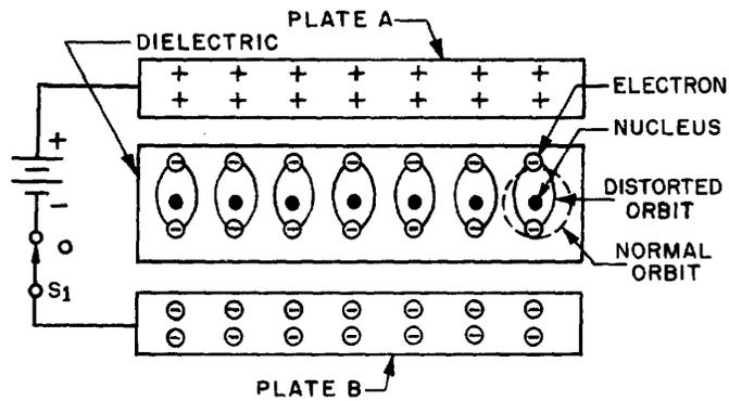
Figure 3-4.—Distortion of electron orbits in a dielectric.
