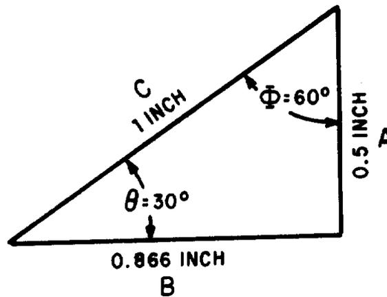
Figure V-2.—A  $30^\circ - 60^\circ - 90^\circ$  triangle.
