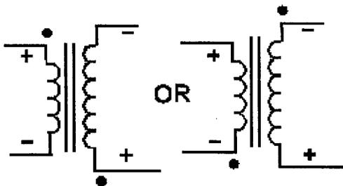
Note: Remember the dots indicate areas of like polarity, NOT a particular polarity.
