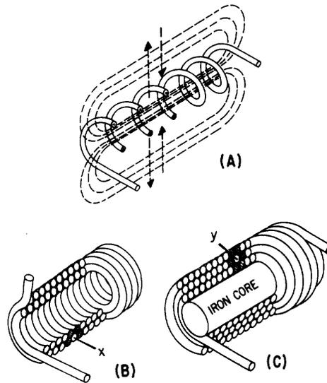
**UNIT OF INDUCTANCE**—Inductance (L) is measured in henrys (H). An inductor has an inductance of one henry (H) if an emf of one volt is induced in the inductor when the current through the inductor is changing at the rate of 1 ampere per second. Common units of inductance are henry (H), millihenry (mH) and the microhenry ( $\mu\text{H}$ ).
