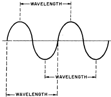
Figure 1-12.—Wavelength measurement.
