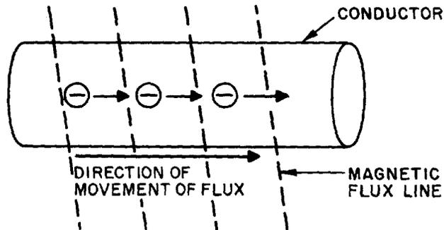
The electrons move from one area of the conductor into another area. The area that the electrons moved from has fewer negative charges (electrons) and becomes positively charged. The area the electrons move into becomes negatively charged. This is shown below:
