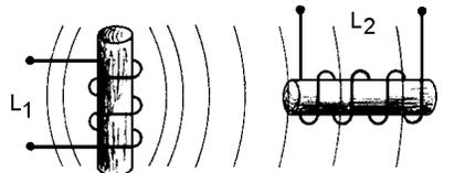
( C ) INDUCTOR AXES PERPENDICULAR – NO  $M$
