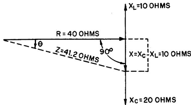
PHASE ANGLE—The number of degrees that current leads or lags voltage in an ac circuit is called the phase angle. The symbol is  $\theta$ .
