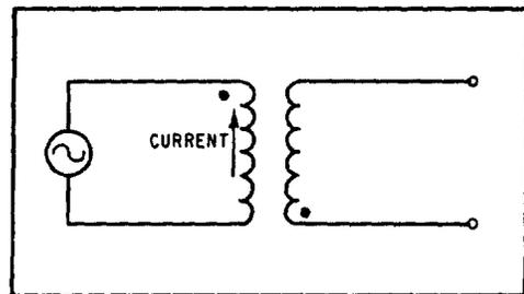
Figure 4B.—Transformer polarity.
