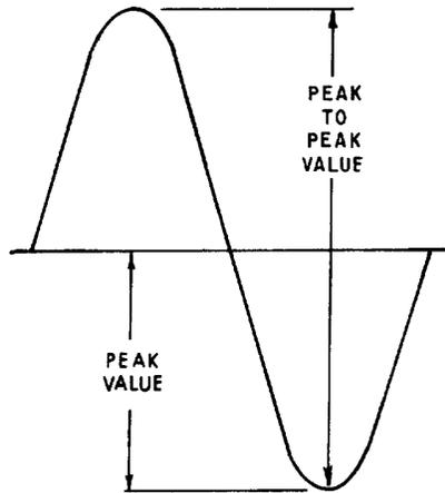
**INSTANTANEOUS VALUE**—The instantaneous value of a sine wave of alternating voltage or current is the value of voltage or current at one particular instant of time. There are an infinite number of instantaneous values between zero and the peak value.
