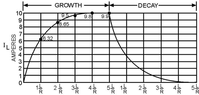
The time constant of an LR circuit may also be defined as the time required for the current in the inductor to grow or decay to its final value if it continued to grow or decay at its initial rate. For all practical purposes, the current in the inductor reaches a maximum value in 5 "Time Constants" and decreases to zero in 5 "Time Constants".
