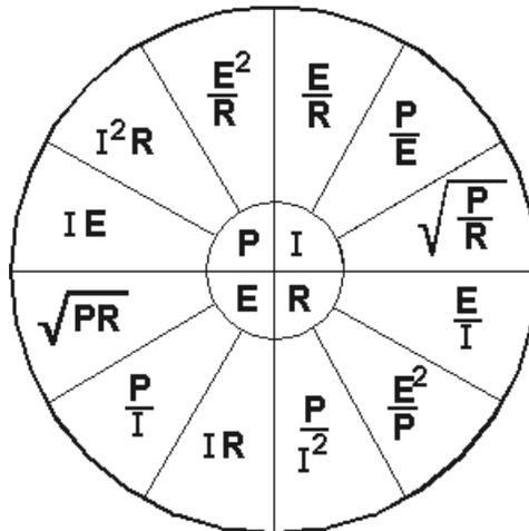
**POWER RATING** in watts indicates the rate at which a device converts electrical energy into another form of energy. The power rating of a resistor indicates the maximum power the resistor can withstand without being destroyed.
