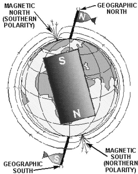
**THE NORTH POLE**, or north seeking pole, of a magnet freely suspended on a string always points toward the north geographical pole.
