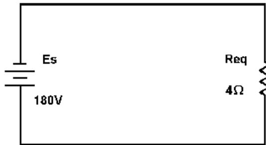
Figure 3-53.—Parallel circuit redrawn to final equivalent circuit.
