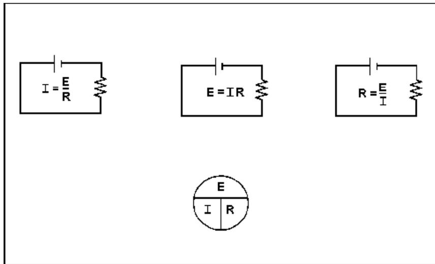
Figure 3-5.—Ohm's law in diagram form.
