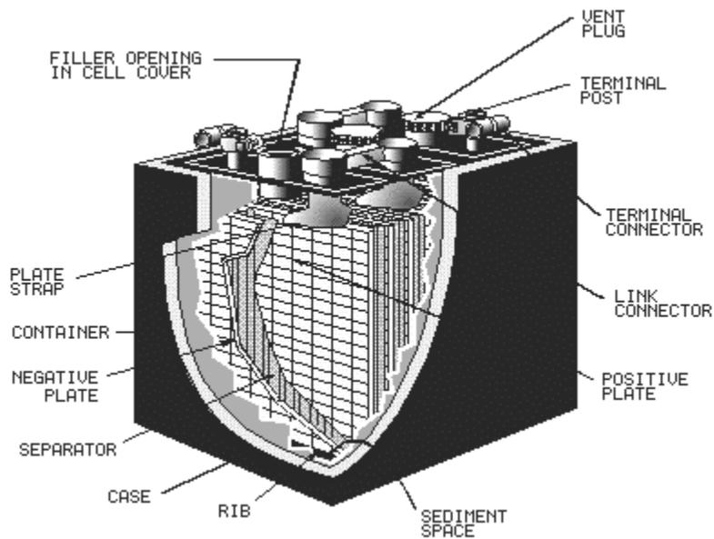
**SERIES CONNECTED CELLS** provide a higher voltage than a single cell, with no increase in current.
