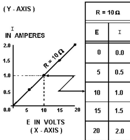
**POWER** is the rate of doing work per unit of time. The time required to perform a given amount of work will determine the power expended. As a formula,  $P = E \times I$ , where P = power in watts, E = voltage in volts, and I = current in amperes.
