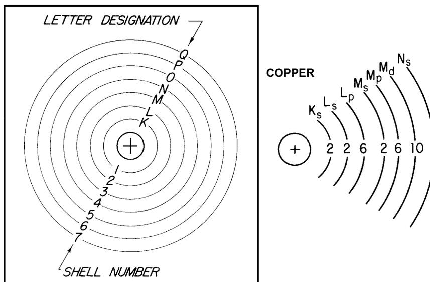
**VALENCE OF AN ATOM** is determined by the number of electrons in the outermost shell. The shell is referred to as the valence shell, and the electrons within it are valence electrons. An atom with few valence electrons requires little energy to free the valence electrons.
