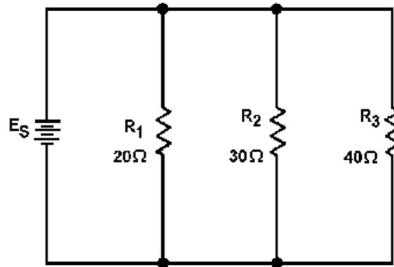
Figure 3-46.—Example parallel circuit with unequal branch resistors.
