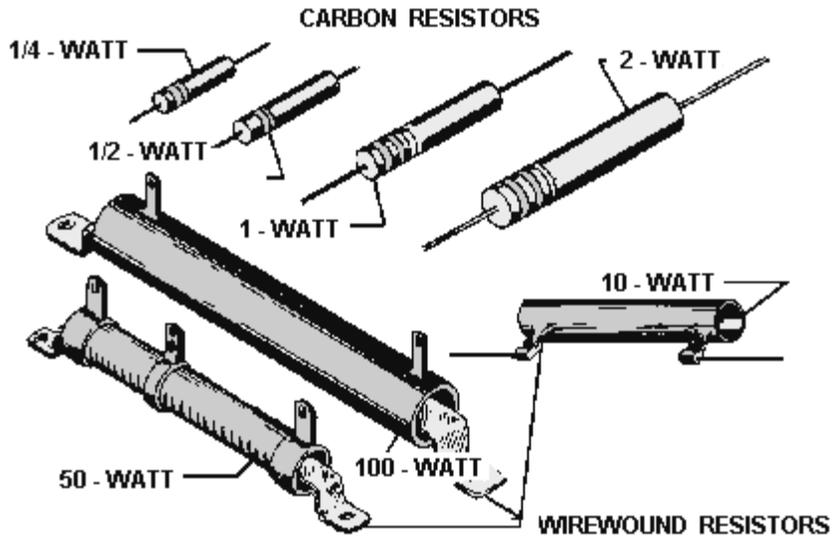
**THE RESISTANCE OF A WIREWOUND RESISTOR** is determined by the metal content of the wire and the wire's length. Wirewound resistors may be tapped so two or more different voltage values may be taken off the same resistor.
