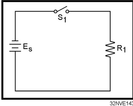
Figure 3A.—Basic circuit.
