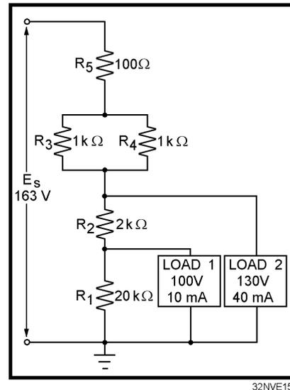
Figure 3I.—Voltage divider.
