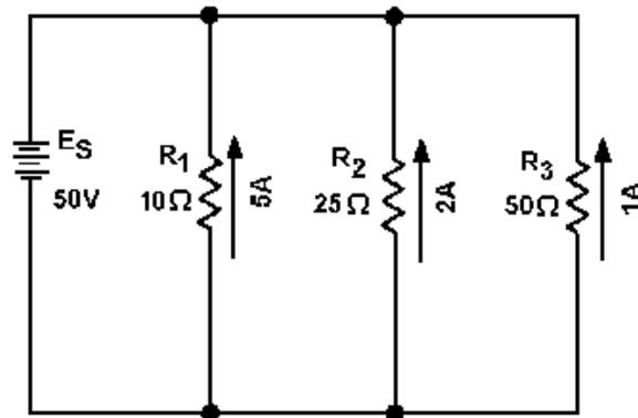
Figure 3-48.—Example parallel circuit.
