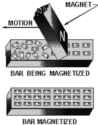
**THE DOMAIN THEORY OF MAGNETISM** states that if the electrons of the atoms in a material spin more in one direction than in the other, the material will become magnetized.
