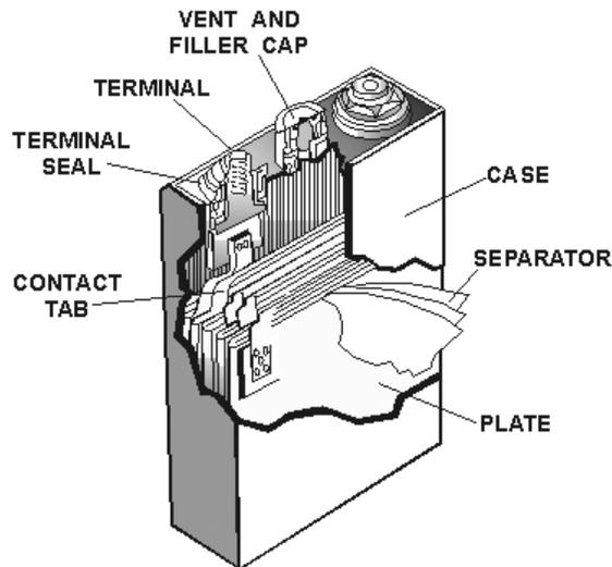
Figure 2-11.—Nickel-cadmium cell.
