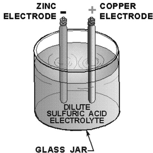
Figure 1-23.—Voltaic cell.
