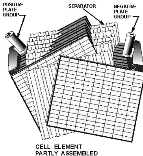
**THE NICKEL-CADMIUM CELL**, commonly called the NICAD, has the following advantages over the lead-acid cell; charges in a shorter period of time, delivers a larger amount of power, stays idle longer, and can be charged and discharged many times. The anode is nickel hydroxide, the cathode is cadmium hydroxide, and the electrolyte is potassium hydroxide and water.
