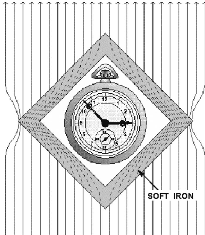
Figure 1-18.—Magnetic shield.
