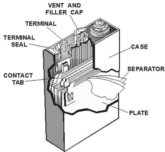
**THE SILVER-ZINC CELL** is used mostly for emergency equipment. It is light, small, and has a large power capacity for its size. The anode is silver oxide, the cathode is zinc, and the electrolyte is potassium hydroxide and water.
