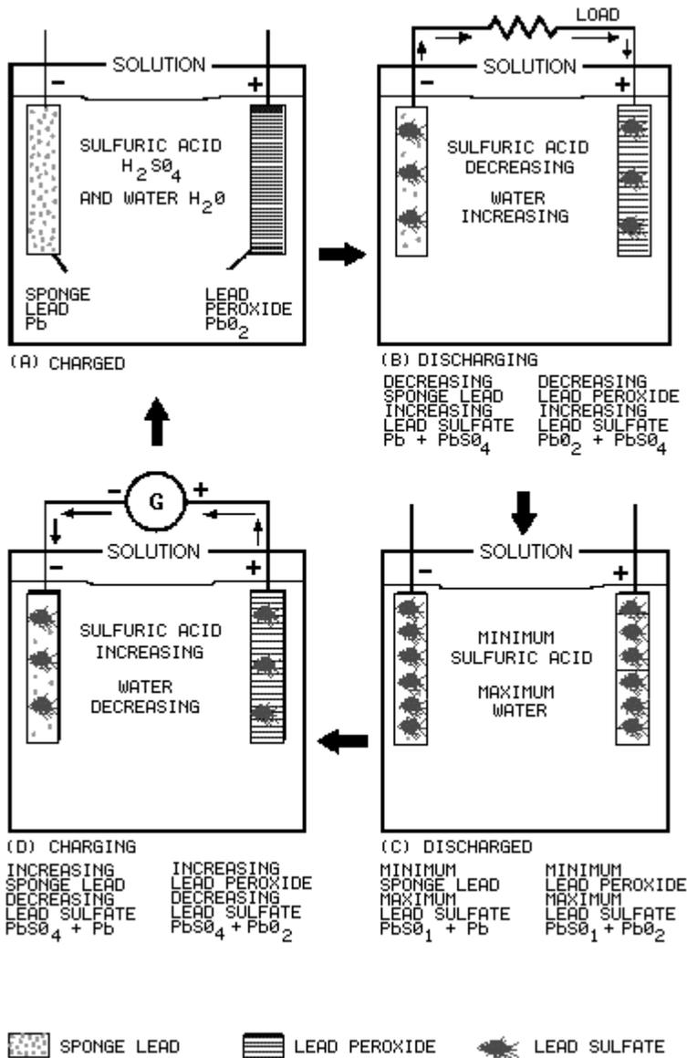
**ELECTROCHEMICAL ACTION** is the process of converting chemical energy into electrical energy.
