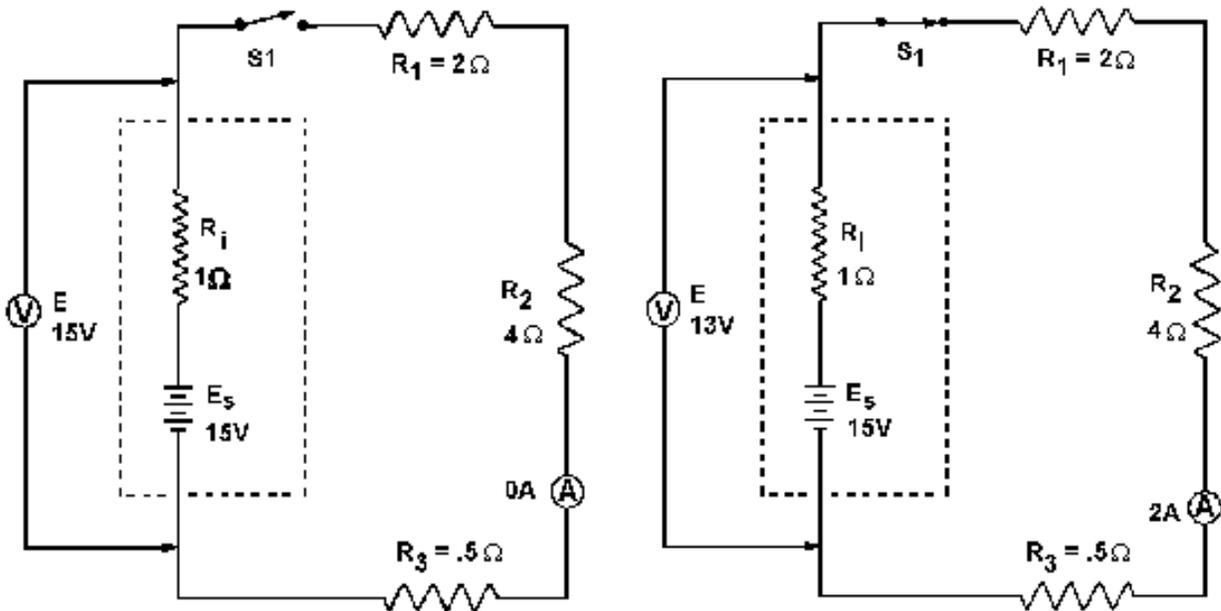
**HIGH EFFICIENCY** in a circuit is achieved when the resistance of the load is high with respect to the resistance of the source.
