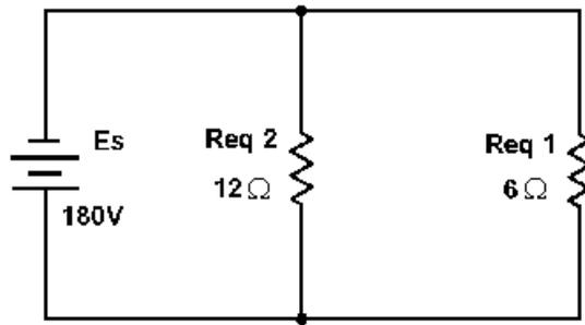
Figure 3-52.—Second equivalent parallel circuit.
