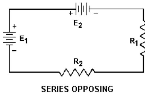
**SERIES OPPOSING VOLTAGES** tend to force current to flow in opposite directions; thus the equivalent voltage is the difference between the opposing voltages.
