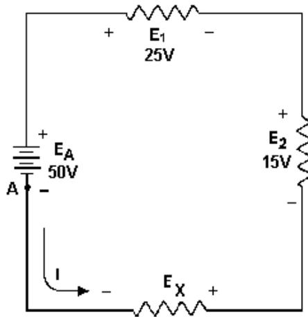
Figure 3-23.—Determining unknown voltage in a series circuit.
