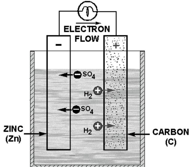
**THE ELECTRODES** are the current conductors of the cell.
