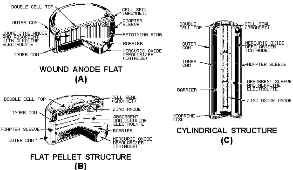
Figure 2-5.—Mercury cells.
