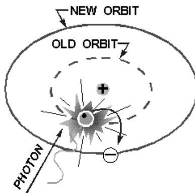
**SHELLS AND SUBSHELLS** of electrons are the orbits of the electrons in the atom. Each shell contains a maximum of 2 times its number squared electrons. Shells are lettered K through Q, starting with K, which is the closest to the nucleus. The shell can be split into 4 subshells labeled s, p, d, and f, which can contain 2, 6, 10, and 14 electrons, respectively.
