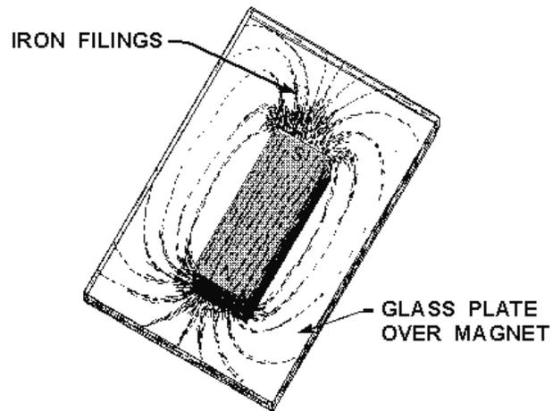
**MAGNETIC LINES OF FORCE** are imaginary lines used to describe the patterns of the magnetic field about a magnet. These lines are assumed to flow externally from the north pole and into the south pole.
