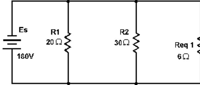
Figure 3-51.—First equivalent parallel circuit.
