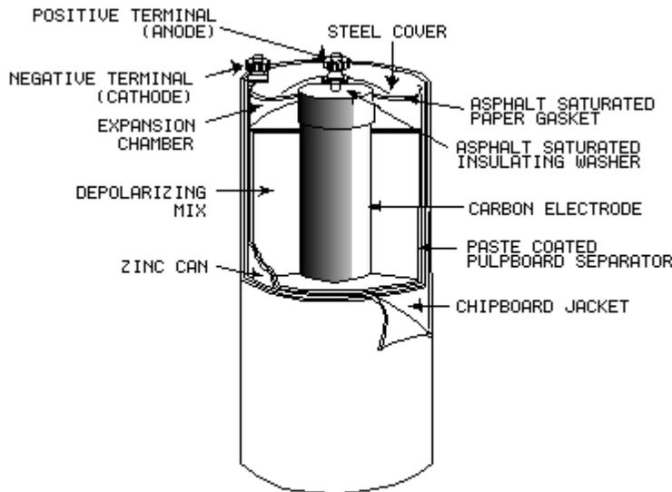
Figure 2-4.—Cutaway view of the general-purpose dry cell.
