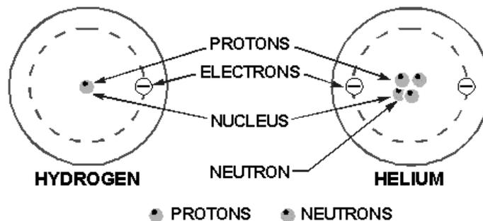
Figure 1-1.—Structures of simple atoms.
