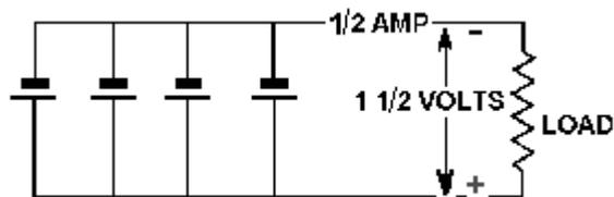
**SERIES-PARALLEL CONNECTED CELLS** provide a higher voltage and a higher current than a single cell.
