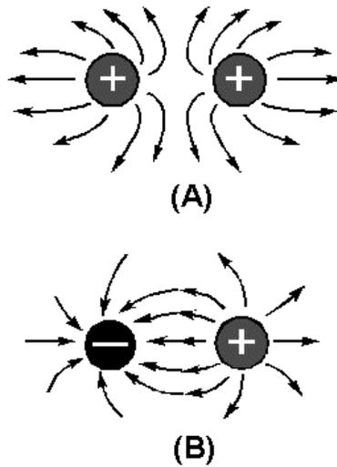
**ELECTROSTATIC LINES** of force are a graphic representation of the field around a charged body. These lines are imaginary. Lines from a positively charged body are indicated as flowing out from the body, while lines from a negatively charged body are indicated as flowing into the body.
