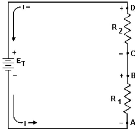
**VOLTAGE POLARITIES** must be used when applying Kirchhoff's voltage law. The point at which current enters a load (resistor) is considered negative with respect to the point at which current leaves the load.
