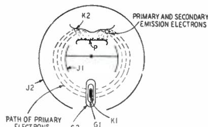
Fig. 3—Operation of the "orbital-beam" tube.
