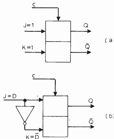
Fig. 7. Illustration of the JK used as a T type flip-flop (a) and as a D type (b)
