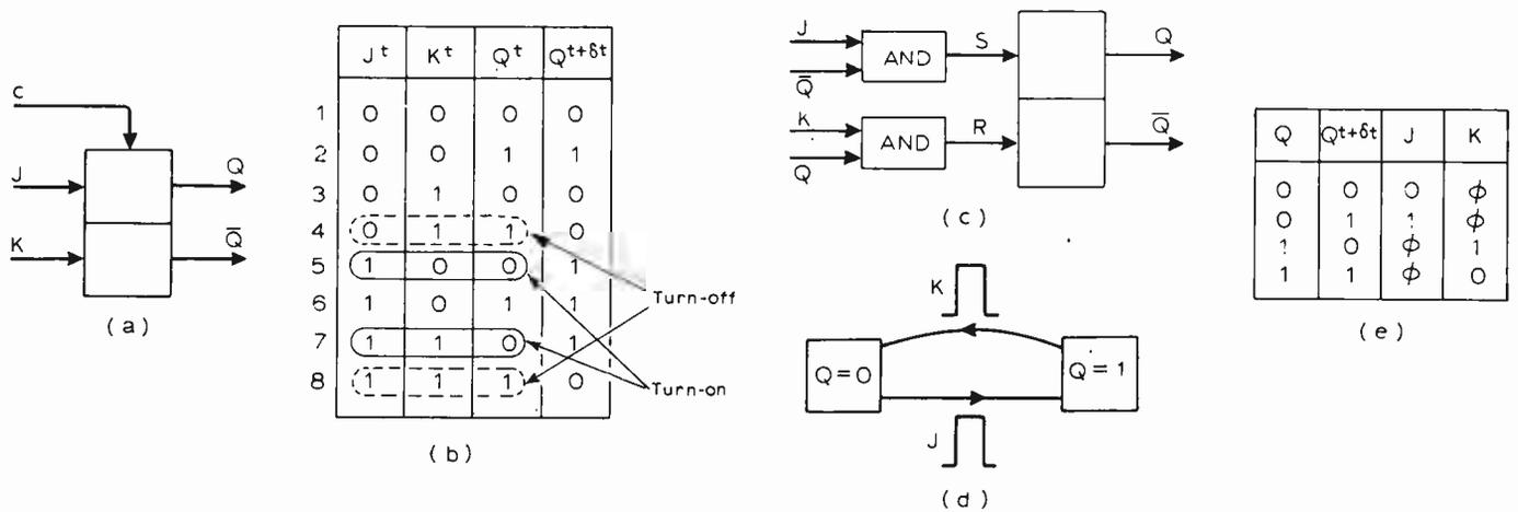
Fig. 3. The JK flip-flop is shown symbolically at (a), with its truth table at (b). That a JK is simply an SR with two NANDs at the inputs is shown by (c). State diagram for a clocked JK is shown at (d) and the steering table at (e). Clocked JK realised in NAND form is at (f), in which the single-input gates are redundant and can be replaced by a wire.
