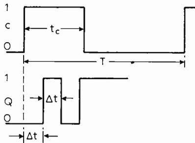
Fig. 4. Illustration of a "race-around", where the output oscillates during the duration of the trigger pulse,  $t_c$
