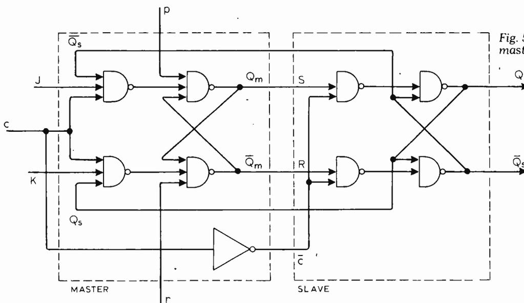
Fig. 5. NAND embodiment of a master/slave flip-flop.
