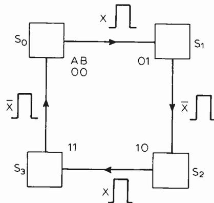
Fig. 8. State diagram for a clock-driven circuit.
