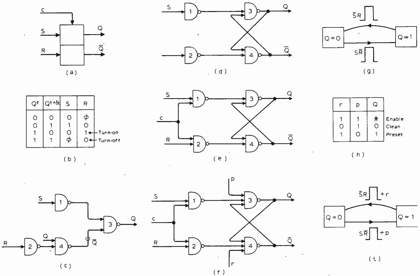
Fig. 2. (a) Symbol for the SR flip-flop, whose steering table is at (b), where Φ indicates either 0 or 1. The SR can be realized, in unclocked form, by NAND gates, as in (c) shown rearranged in a more familiar form at (d). A clocked type of SR is seen at (e) and, with preset and clear, at (f). State diagram for the clocked SR is at (g) and the truth table for P and C can be seen at (h). At (i) is the state diagram for a clocked SR with P and C controls.
