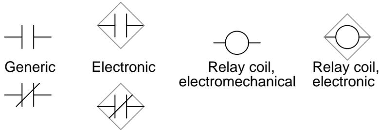
*Relays, electronic schematic notation style*
