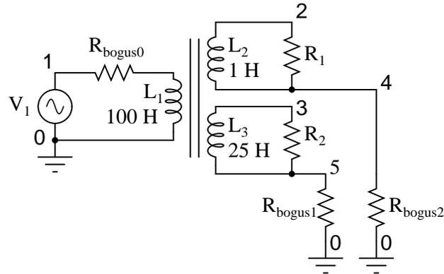
SPICE understands transformers as a set of mutually coupled inductors. Thus, to simulate a transformer in SPICE, you must specify the primary and secondary windings as separate inductors, then instruct SPICE to link them together with a "k" card specifying the coupling constant. For ideal transformer simulation, the coupling constant would be unity (1). However, SPICE can't handle this value, so we use something like 0.999 as the coupling factor.
