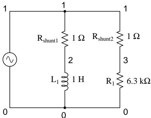
The currents through each leg are indicated by the voltage drops across each respective shunt resistor (1 amp = 1 volt through 1  $\Omega$ ), output by the `v(1,2)` and `v(1,3)` terms of the `.print` card. The phase of the currents through each leg are indicated by the phase of the voltage drops across each respective shunt resistor, output by the `vp(1,2)` and `vp(1,3)` terms in the `.print` card.
