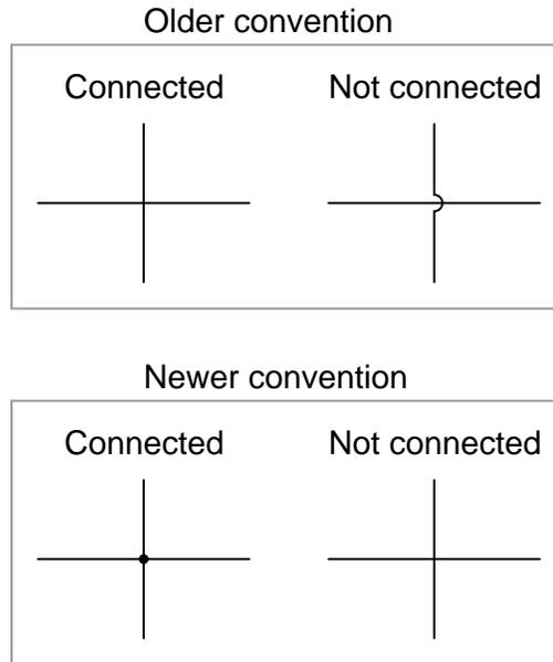
Older electrical schematics showed connecting wires crossing, while non-connecting wires “jumped” over each other with little half-circle marks. Newer electrical schematics show connecting wires joining with a dot, while non-connecting wires cross with no dot. However, some people still use the older convention of connecting wires crossing with no dot, which may create confusion.
