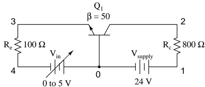
This analysis sweeps the input voltage ( $V_{in}$ ) from 0 to 5 volts in 0.1 volt increments, then prints out the voltage between the collector and emitter leads of the transistor  $v(2,3)$ . The transistor ( $Q_1$ ) is an NPN with a forward Beta of 50.
