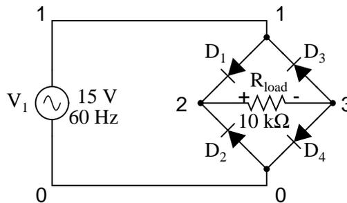
Diodes, like all semiconductor components in SPICE, must be modeled so that SPICE knows all the nitty-gritty details of how they're supposed to work. Fortunately, SPICE comes with a few generic models, and the diode is the most basic. Notice the `.model` card which simply specifies "d" as the generic diode model for `mod1`. Again, since we're plotting the waveforms here, we need to specify all parameters of the AC source in a single card and print/plot all values using the `.tran` option.
