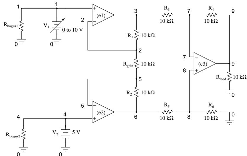
Note the very high-resistance  $R_{bogus1}$  and  $R_{bogus2}$  resistors in the netlist (not shown in schematic for brevity) across each input voltage source, to keep SPICE from thinking  $V_1$  and  $V_2$  were open-circuited, just like the other op-amp circuit examples.
