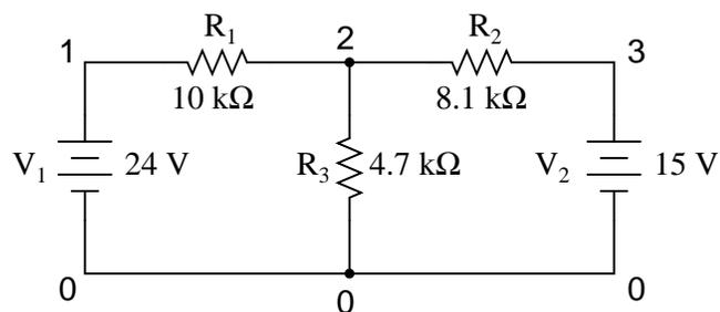
By adding a `.dc` analysis card and specifying source  $V_1$  from 24 volts to 24 volts in 1 step (in other words, 24 volts steady), we can use the `.print` card analysis to print out voltages between any two points we desire. Oddly enough, when the `.dc` analysis option is invoked, the default voltage printouts for each node (to ground) disappears, so we end up having to explicitly specify them in the `.print` card to see them at all.
