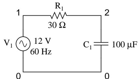
The `.ac` card specifies the points of ac analysis from 60Hz to 60Hz, at a single point. This card, of course, is a bit more useful for multi-frequency analysis, where a range of frequencies can be analyzed in steps. The `.print` card outputs the AC voltage between nodes 1 and 2, and the AC voltage between node 2 and ground.
