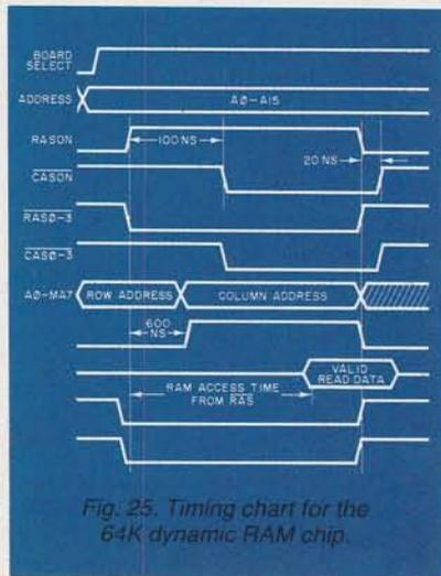
Fig. 25. Timing chart for the 64K dynamic RAM chip.
