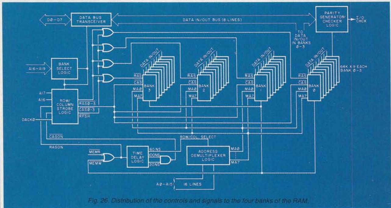
Fig. 26. Distribution of the controls and signals to the four banks of the RAM.
