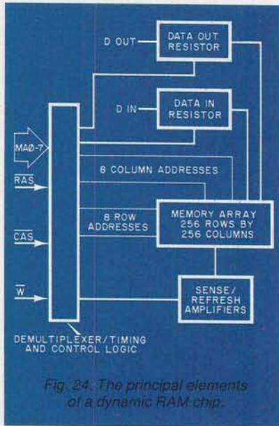
Fig. 24. The principal elements of a dynamic RAM chip.
