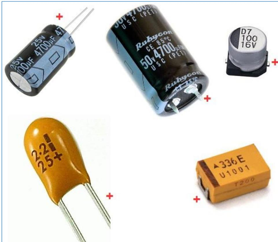
Figure 169 - Polarity in aluminum and tantalum electrolytic capacitors.
