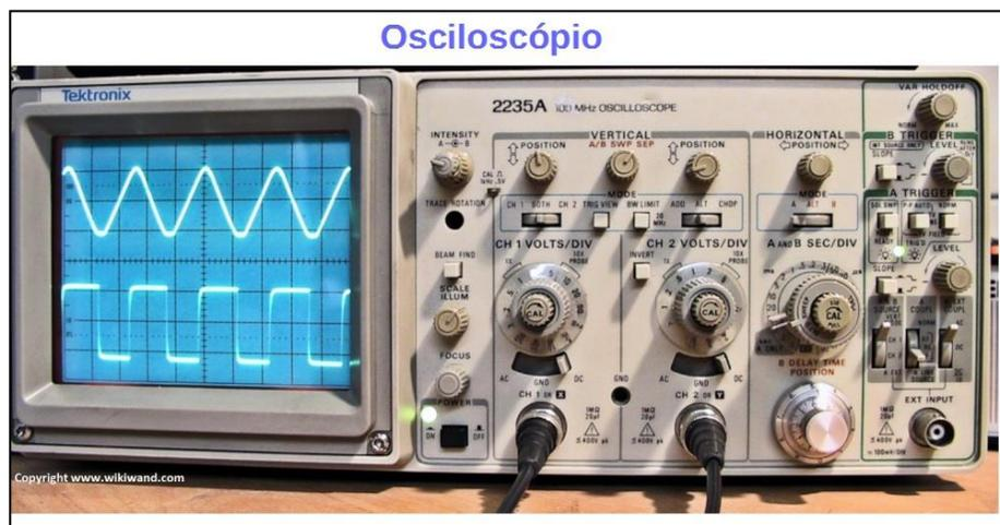
Figure 96 - Oscilloscope showing two waveforms on your screen.
