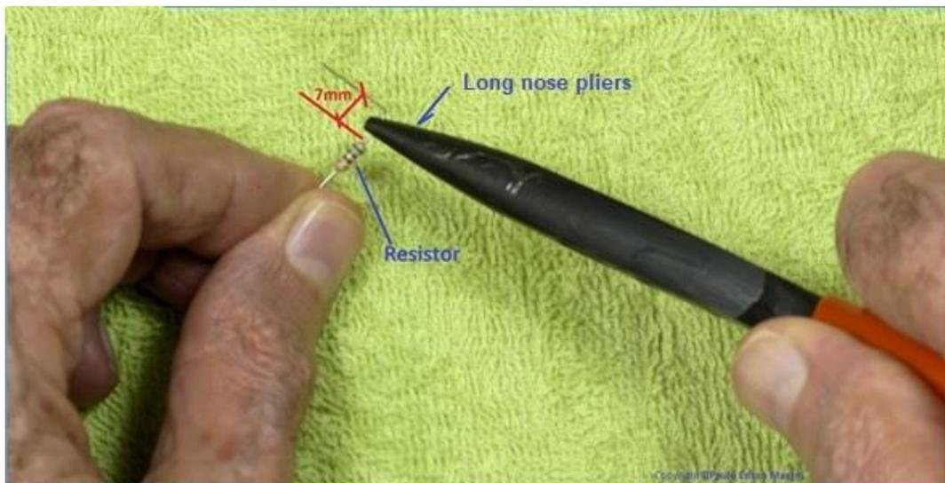
Figure 76 – Bending the terminal of the 560-ohm resistor.
