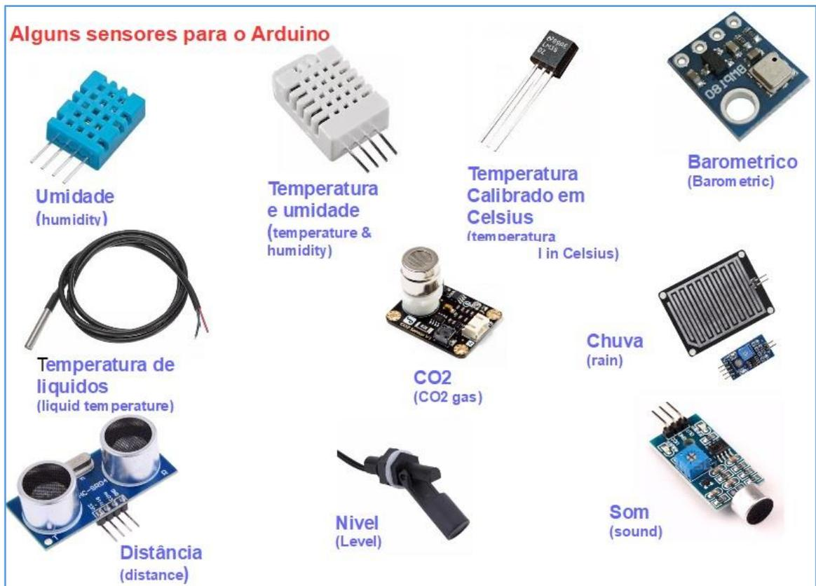
Figure 293 Some types of sensor for Arduino and similar.
