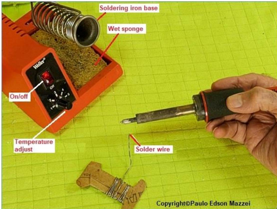
Figure 214 - How to hold the soldering iron.
