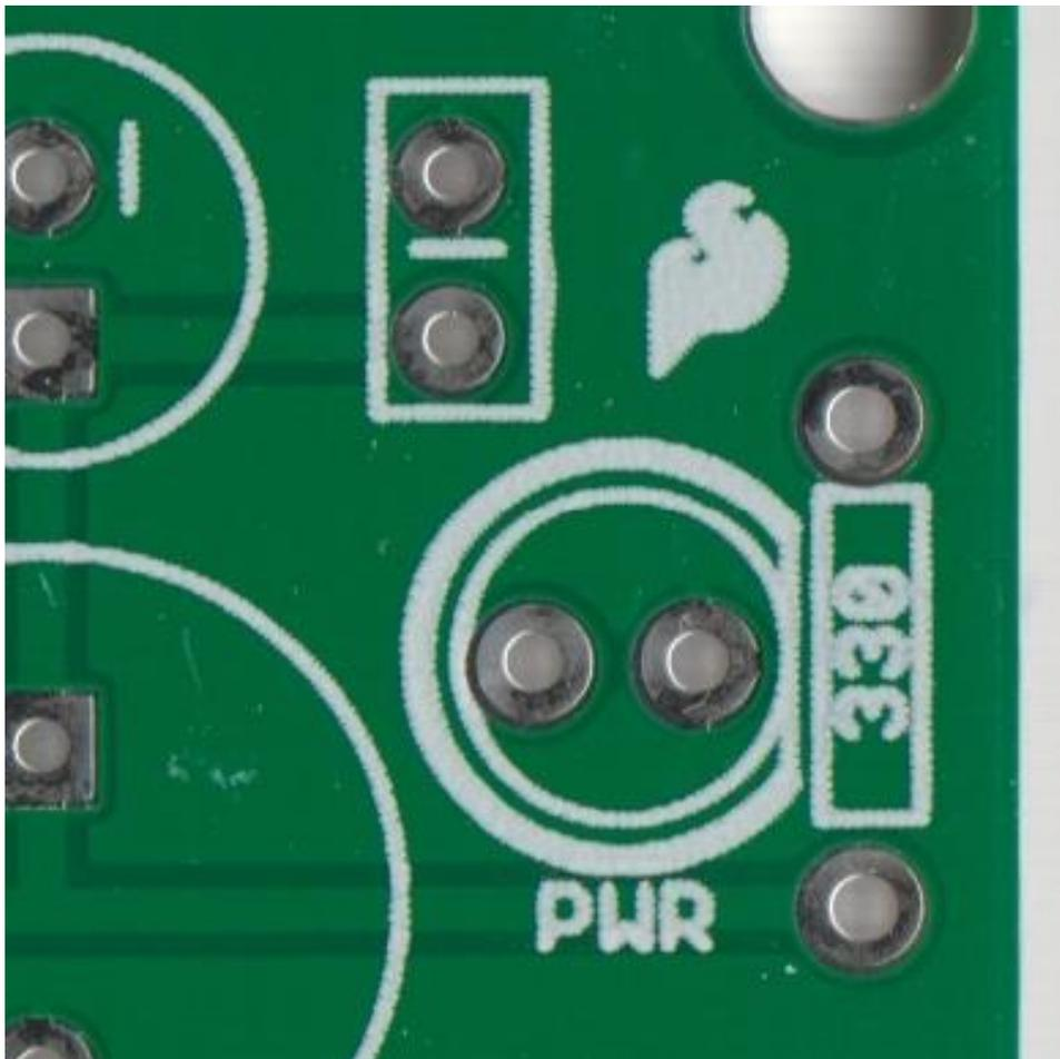
*Figure 290 - Silkscreen process in a PCB.*
