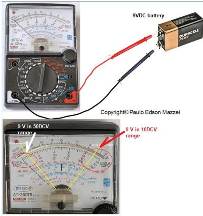
Figure 33 Measuring the DC volts of a 9 V battery.
