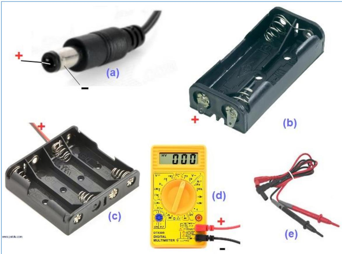
*Figure 171 - Polarity in components.*
