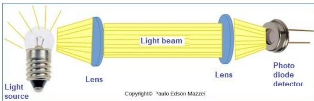
Figure 268 - Use of a light source, lenses and a light receiver.
