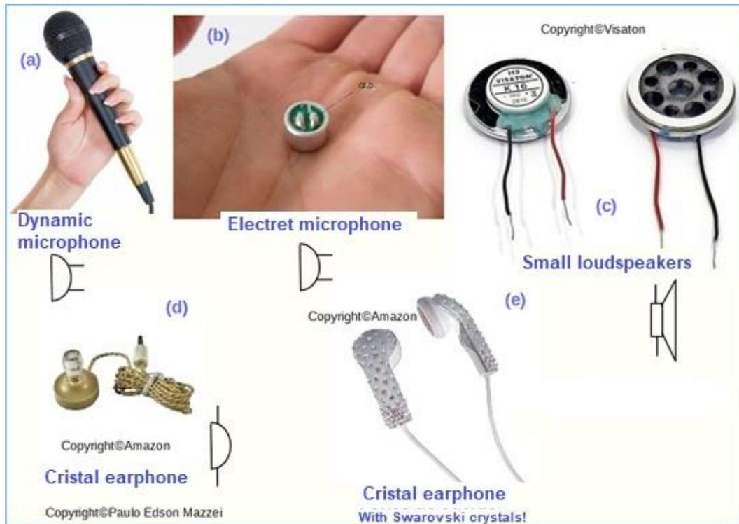
Figure 905- Microphones, loudspeakers and earphones.
