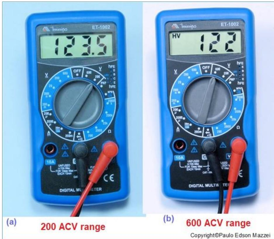
Figure 26 - 127VAC voltage, measured at two different DMM ranges.
