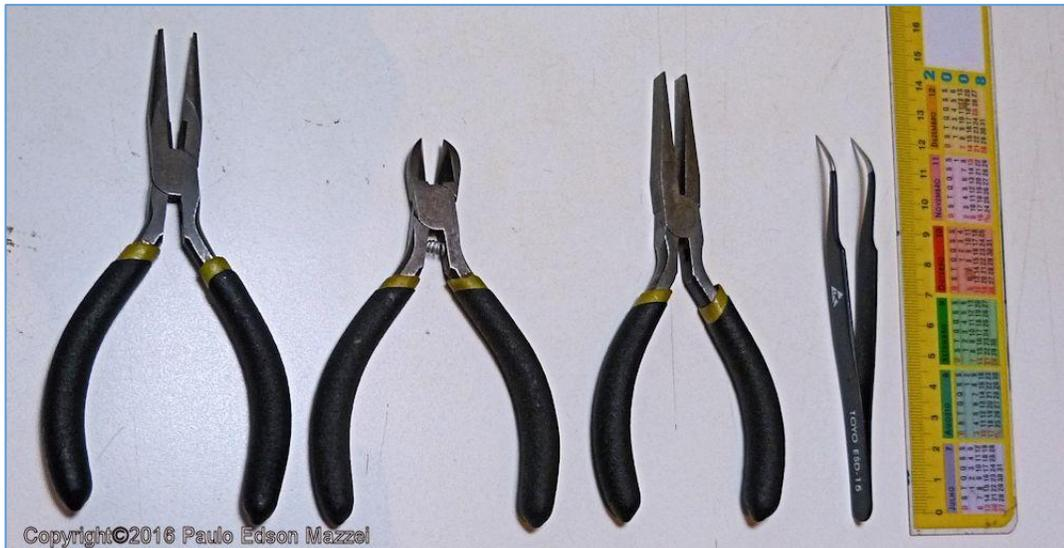
*Figure 1 - Simple tools for use in electronics.*
