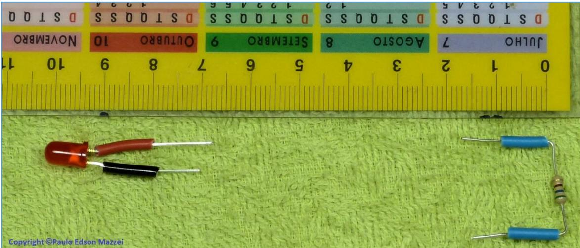
Figure 77 – LED and resistor with small pieces of cover in their terminals.
