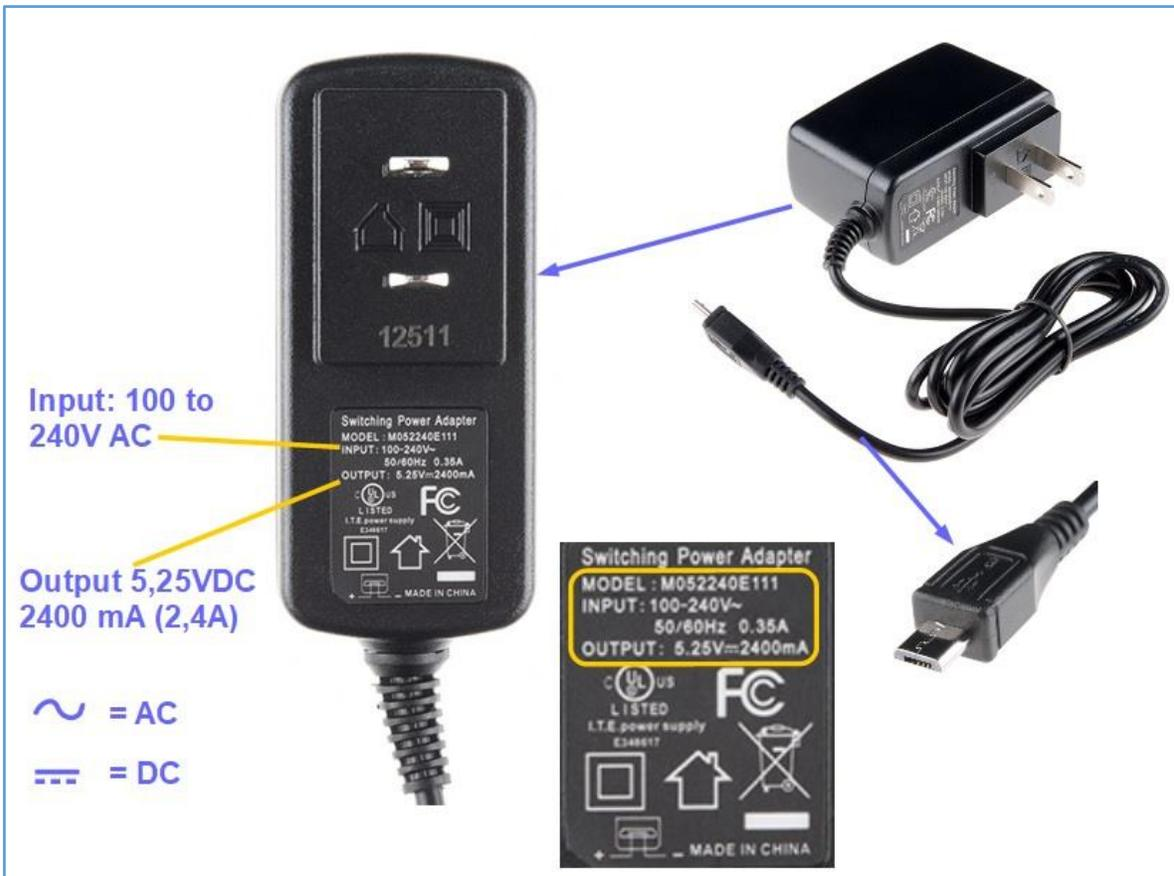
Figure 176 - Alternating Current Adapter. Input from 100 to 240VAC and output of 5.25VDC - 2.4 A.
