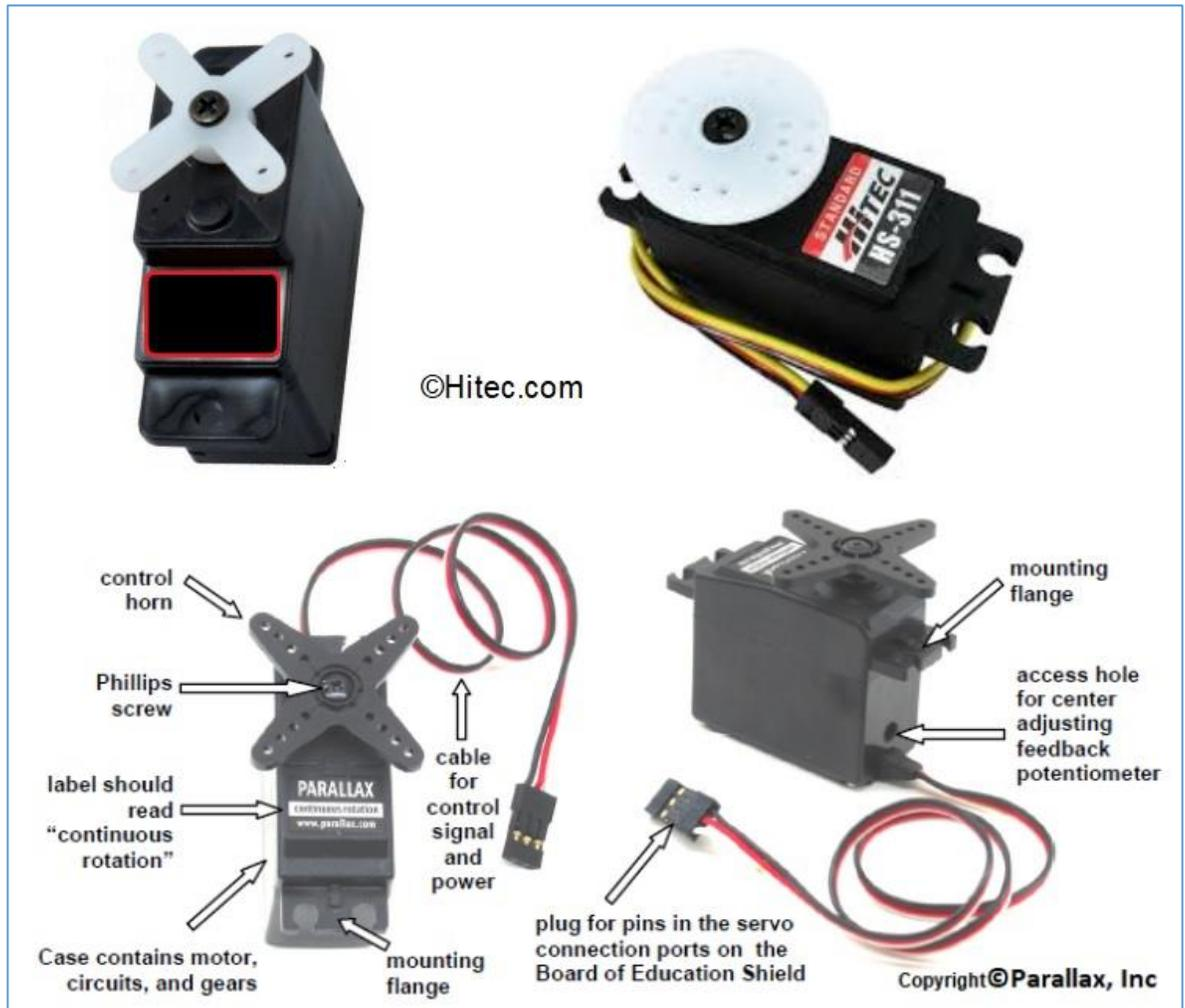
Figure 300 - Examples of servo motors. See the excellent description in the design of Parallax, Inc.
