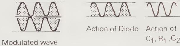
The high radio frequency is shorted to ground by  $C_1$ , and the low-pass filter  $R_1$ - $C_2$  removes any remaining trace of radio frequency from the output signal. Capacitor  $C_3$  is used to couple the signal to the next stage of amplification.
