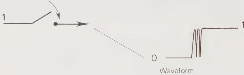
Fig. 9.13 The SWITCH-BOUNCE Waveform.
