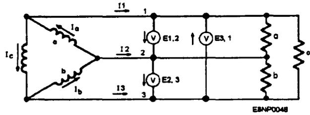
Figure 3-14.—Three-phase, delta-connected system.
