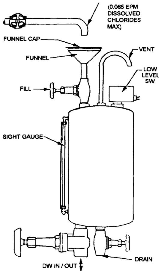
Figure 1-11.—Gravity expansion tank.
