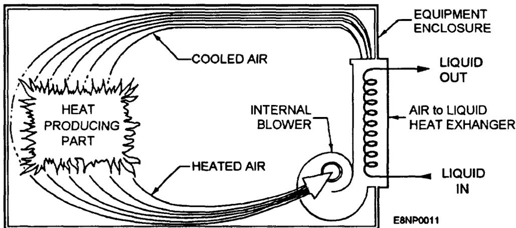
Figure 1-5.—Air-to-liquid cooling.
