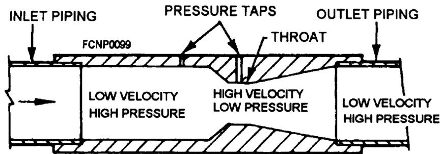
Figure 1-22.-Venturi flowmeter.
