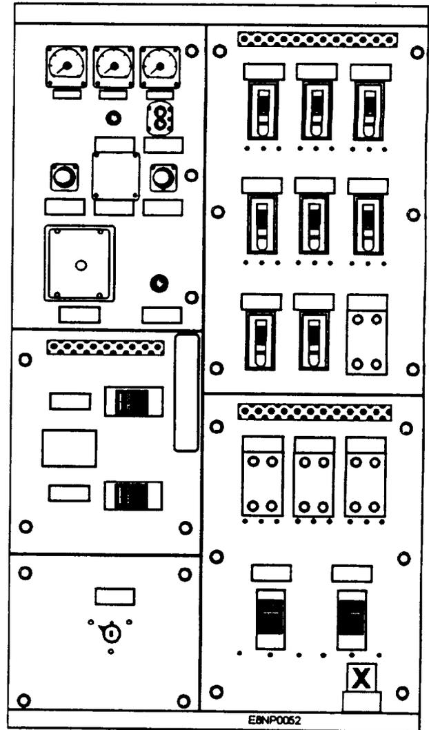
Figure 3-18. 400-Hz switchboard.
