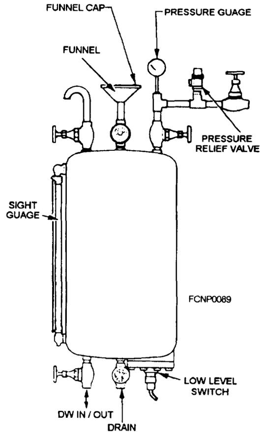
Figure 1-12.—Pre-ssure expansion tank.
