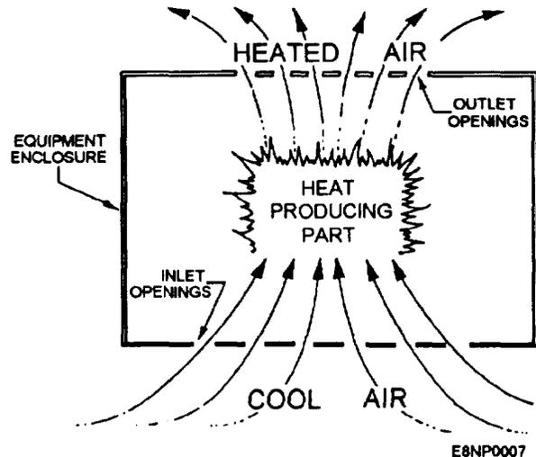
Figure 1-1.-Convection cooling.
