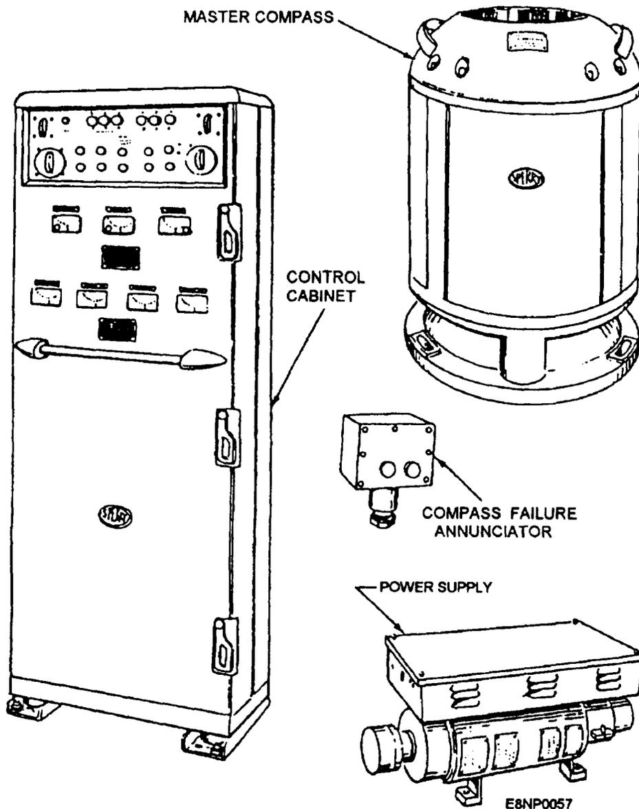
Figure 4-1.—Mk 19 Mod 3A gyrocompass equipment.
