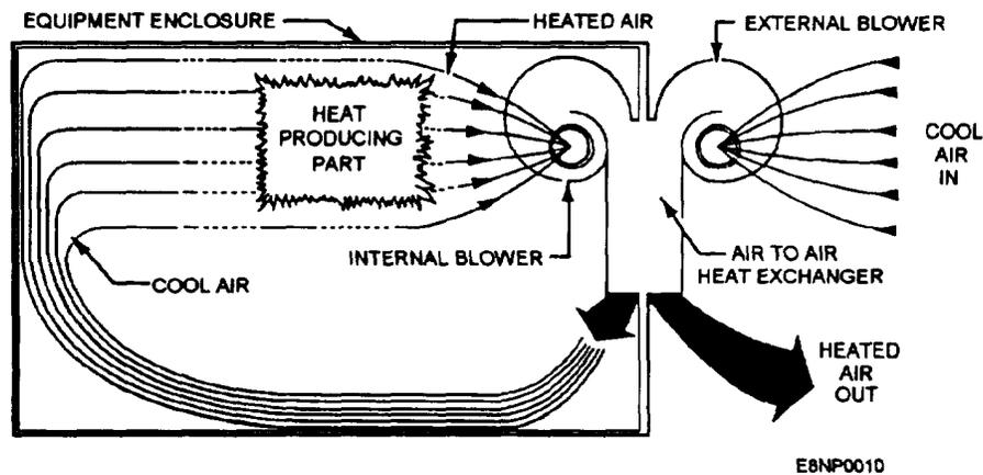
Figure 1-4.—Air-to-air cooling.
