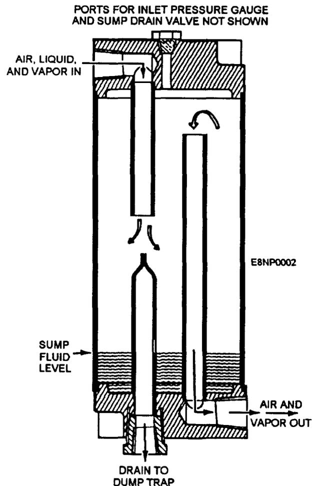
Figure 2-2.—Fluid separator.
