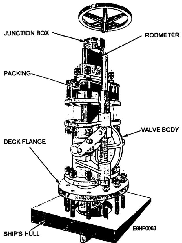
Figure 4-7.—Exploded view of these valve.
