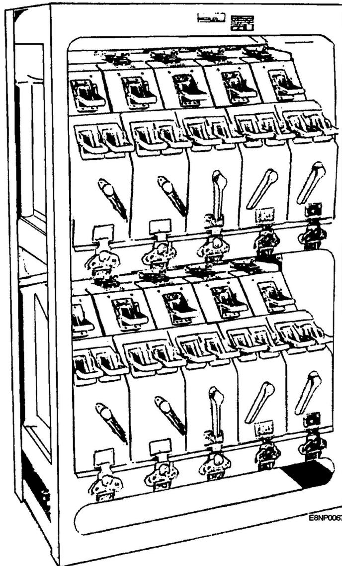
**Figure 5-1.—Manual switchboard.**
