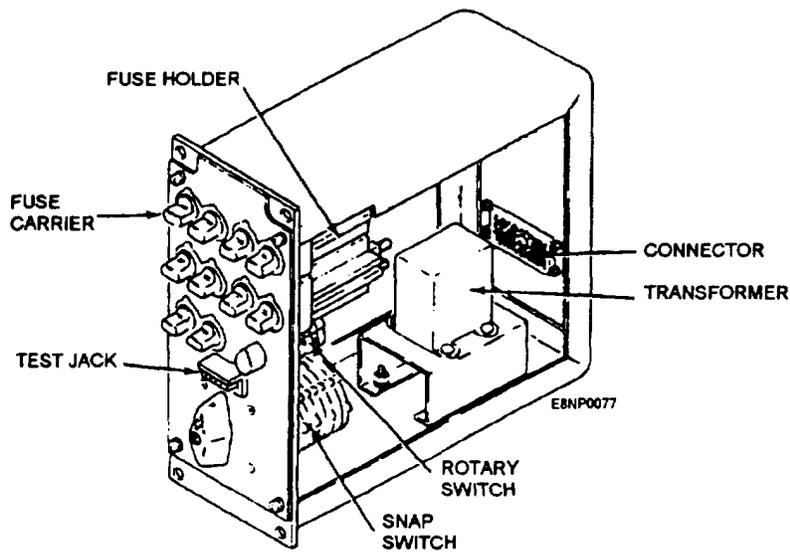
Figure 5-11.—Switch control and potential transformer ACO assembly.
