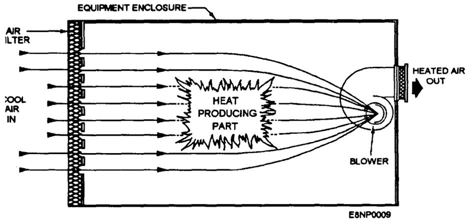
Figure 1-3.—Forced-air cooling.
