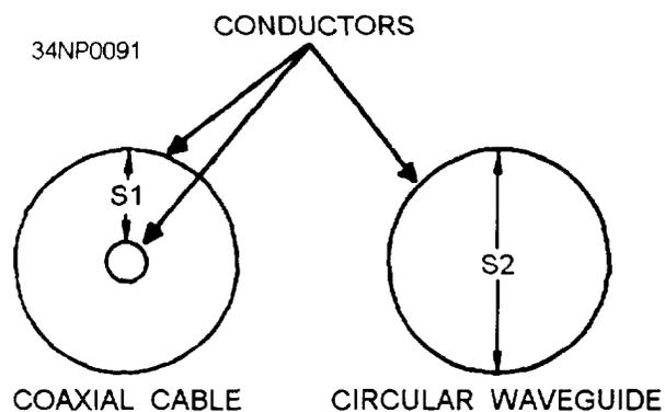
**Figure 3-18.—Comparison of spacing in coaxial cable and a circular waveguide.**
