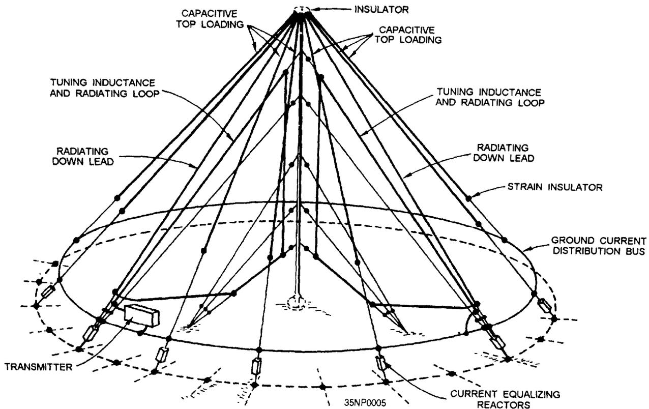
Figure 2-13.—Pan polar antenna.
