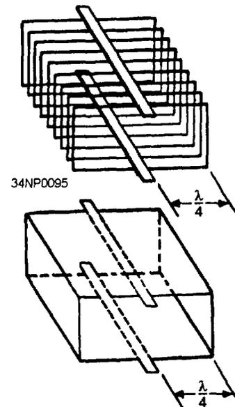
Figure 3-22.—Forming a waveguide by adding quarter-wave sections.
