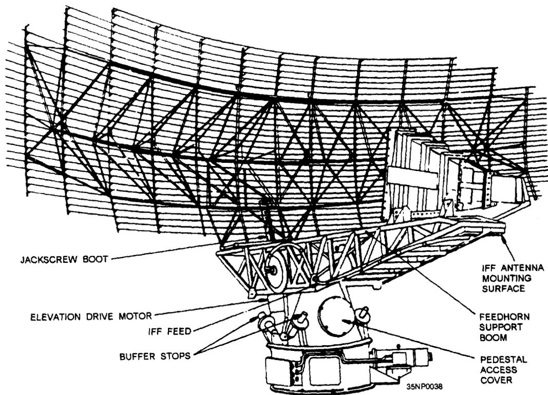
Figure 2-46.—AS-3263/SPS-49(V) antenna.
