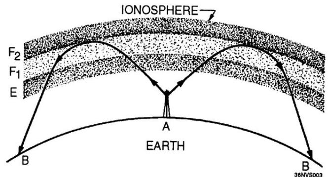
Figure 1-3.—Radio-wave refraction.
