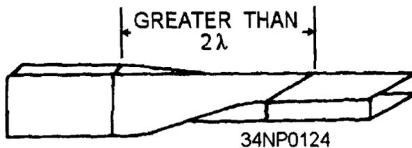
Figure 3-51.—Waveguide twist.
