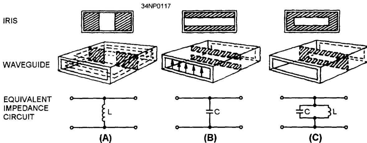
Figure 3-44.—Waveguide irises.
