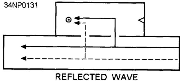
Figure 3-58.—Directional coupler designed to sample reflected energy.
