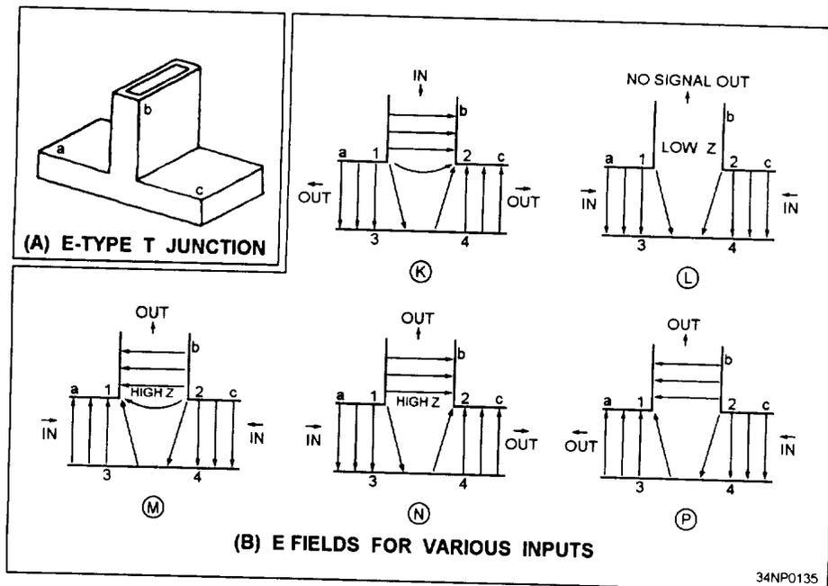
Figure 3-62.—E fields in an E-type T junction.
