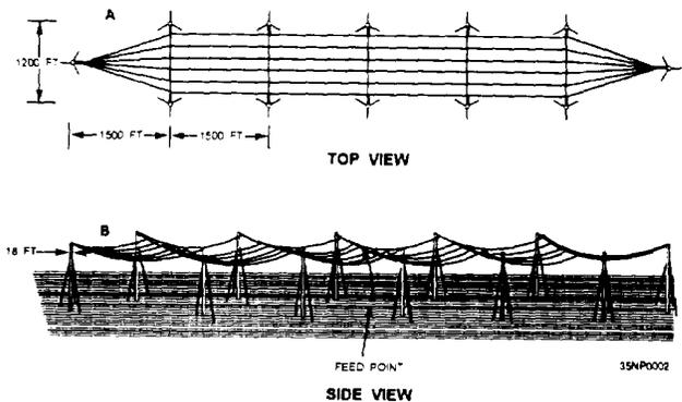
Figure 2-10.—Triatic-type antenna.
