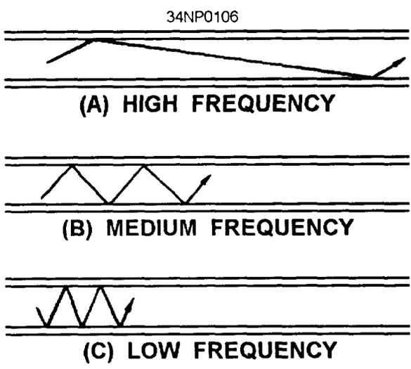
Figure 3-33.—Reflection angle at various frequencies.
