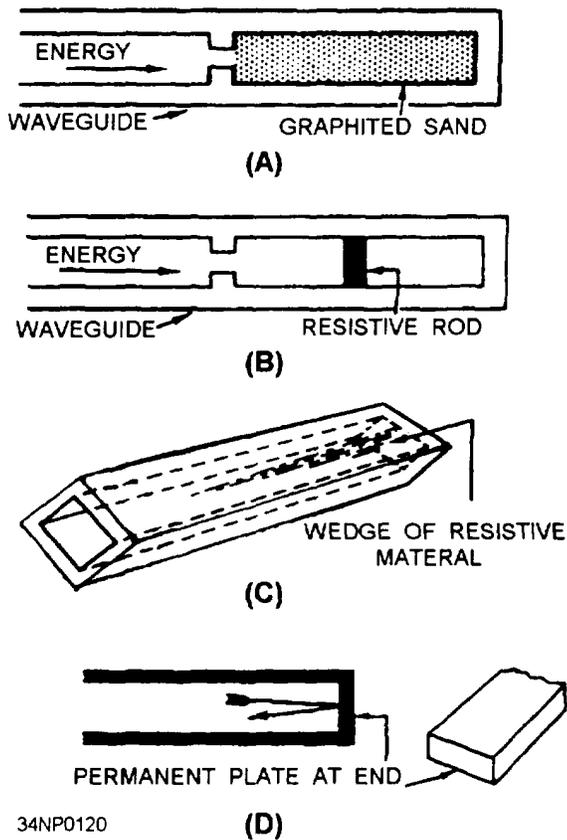
Figure 3-47.—Terminating waveguides.
