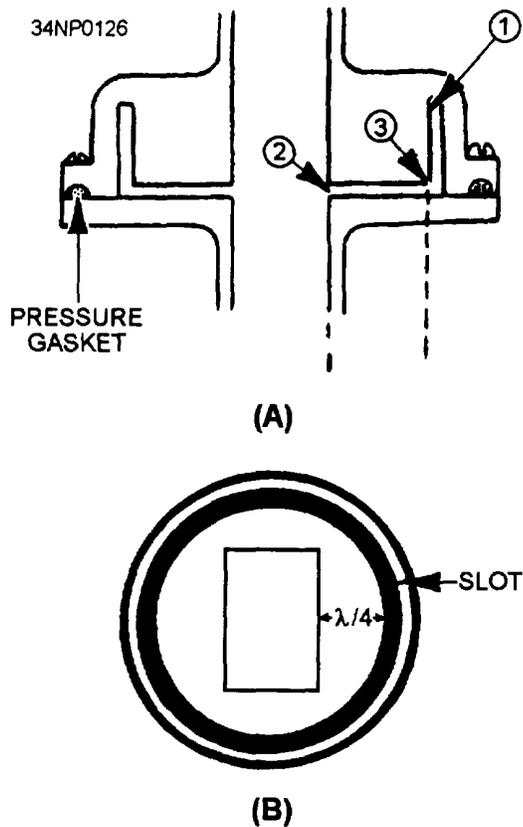
Figure 3-53.—Choke joint.
