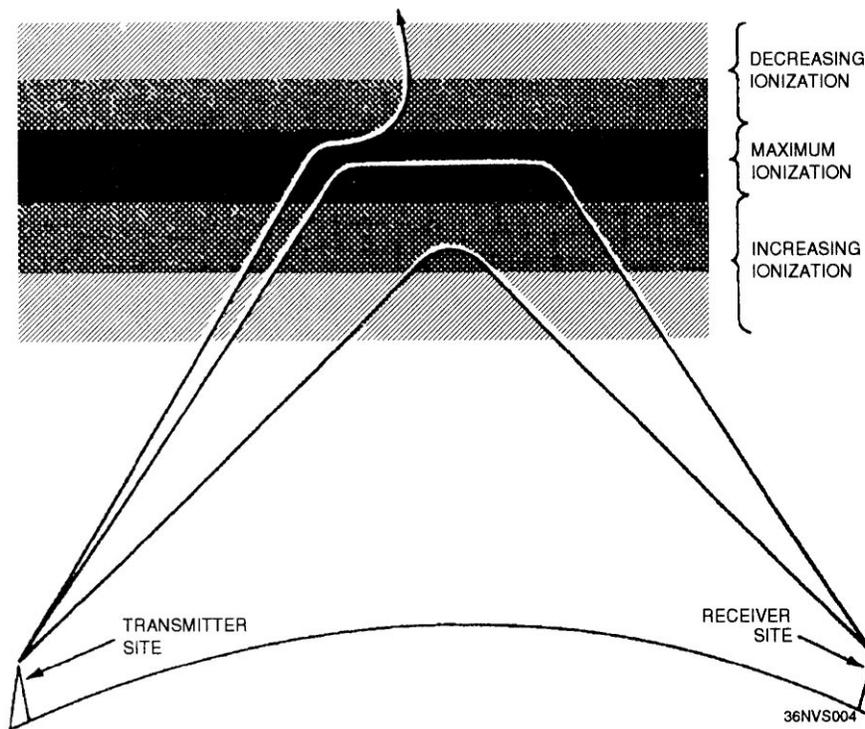
**Figure 1-4.—Effects of ionospheric density on radio waves.**
