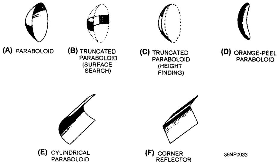
**Figure 2-41.—Reflector shapes.**
