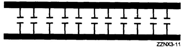
Figure 3-3.—Distributed capacitance.
