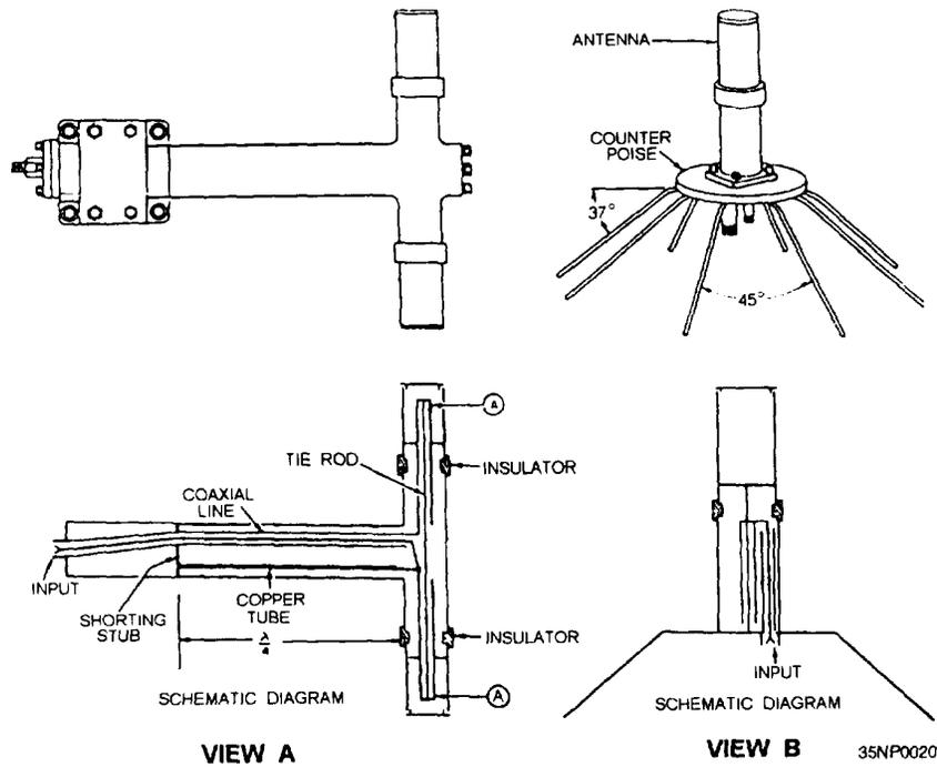
Figure 2-28.—Coaxial dipole.
