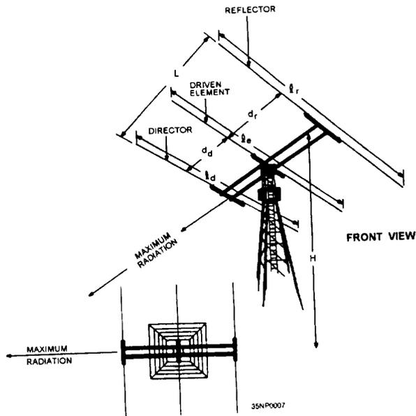
Figure 2-15.—Yagi antenna.
