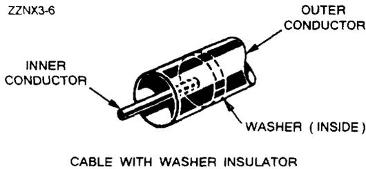
**Figure 3-13.—Air coaxial line.**
