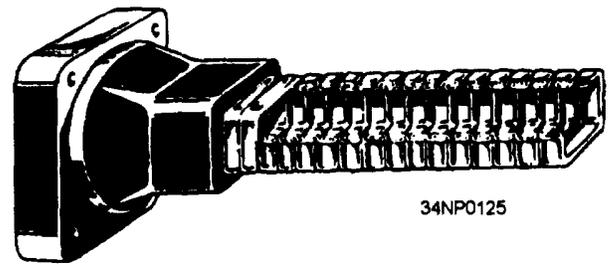
Figure 3-52.—Flexible waveguide.
