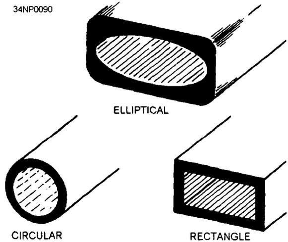
Figure 3-17.—Waveguide shapes.
