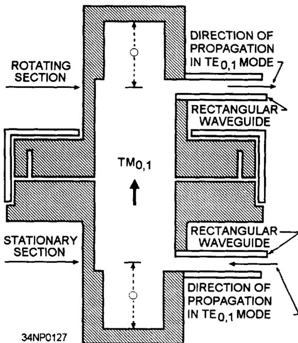
Figure 3-54.—Rotating joint.
