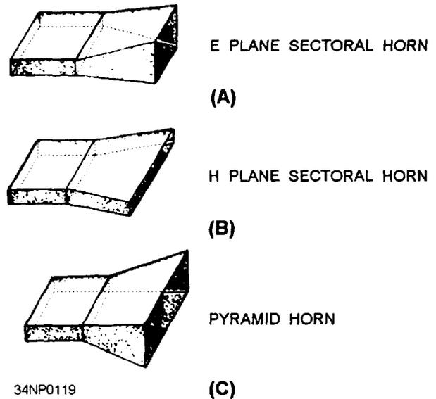
Figure 3-46.—Waveguide horns.
