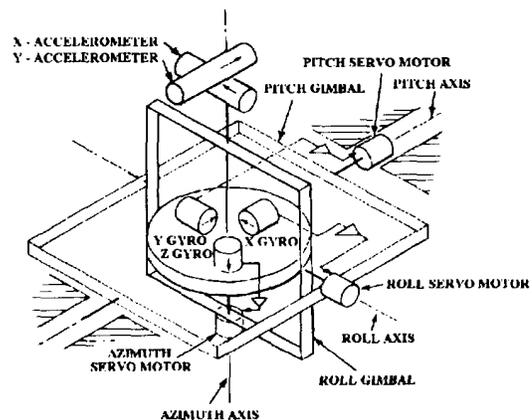
Figure 1-1.—Stable platform with inertial components.
