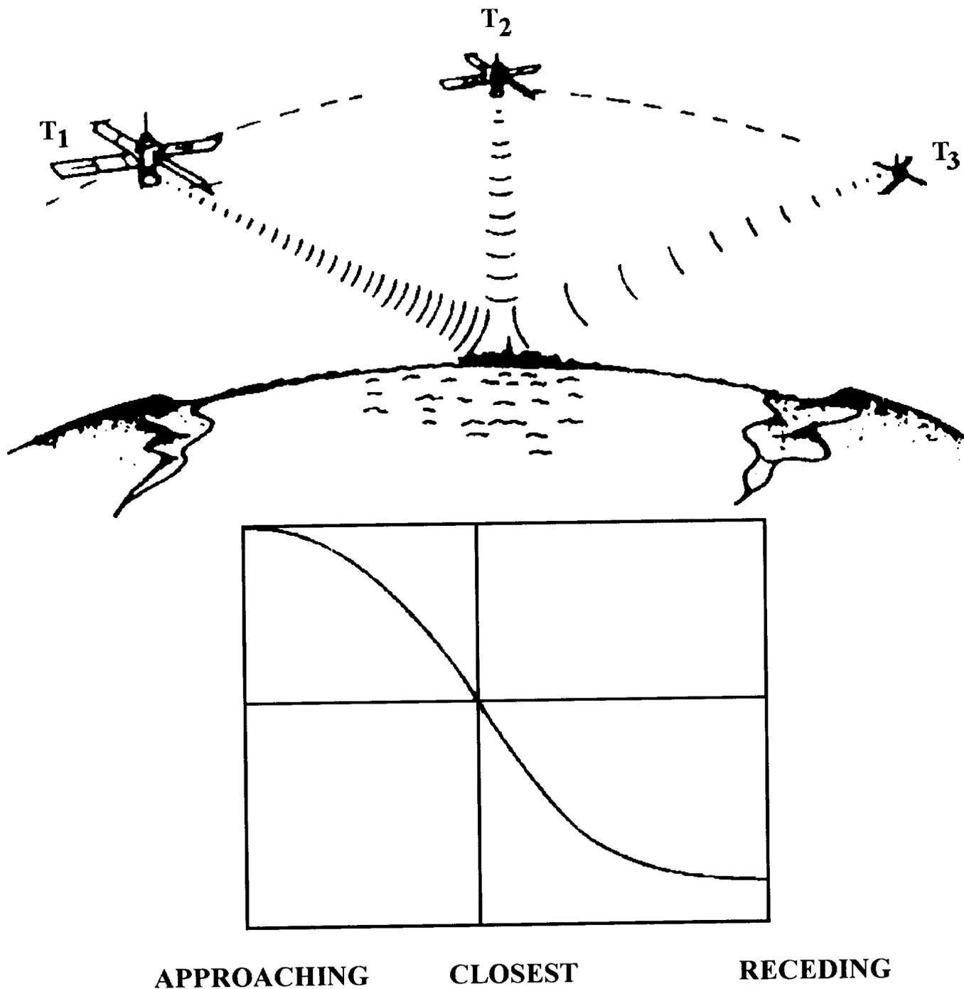
Figure 1-7.—Doppler shift relative to satellite transmitted frequency.
