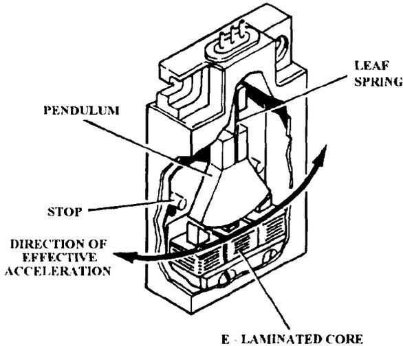
Figure 1-2.—E-transformer accelerometer.
