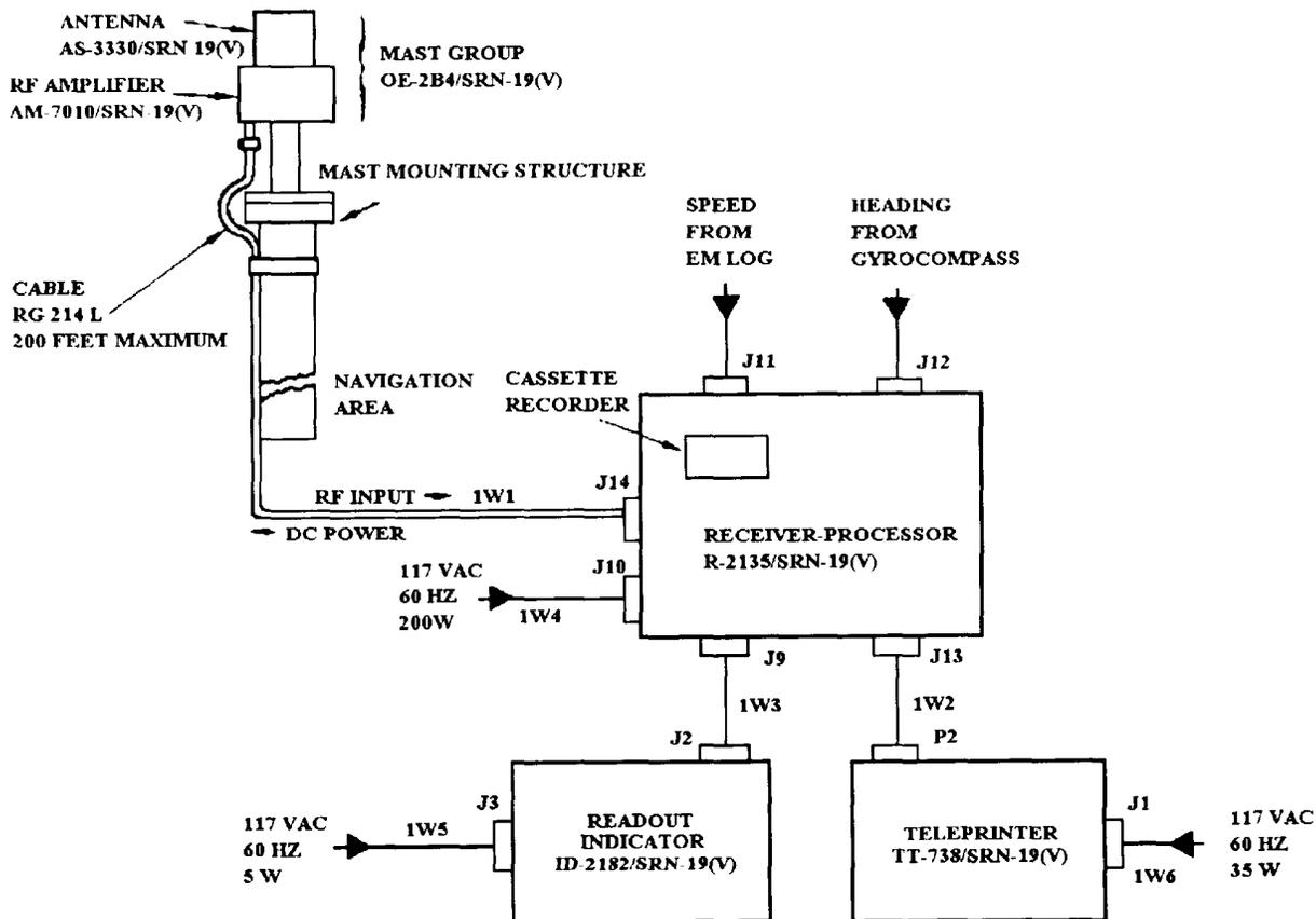
Figure 1-10.—AN/SRN-19(V)2 simplified block diagram.
