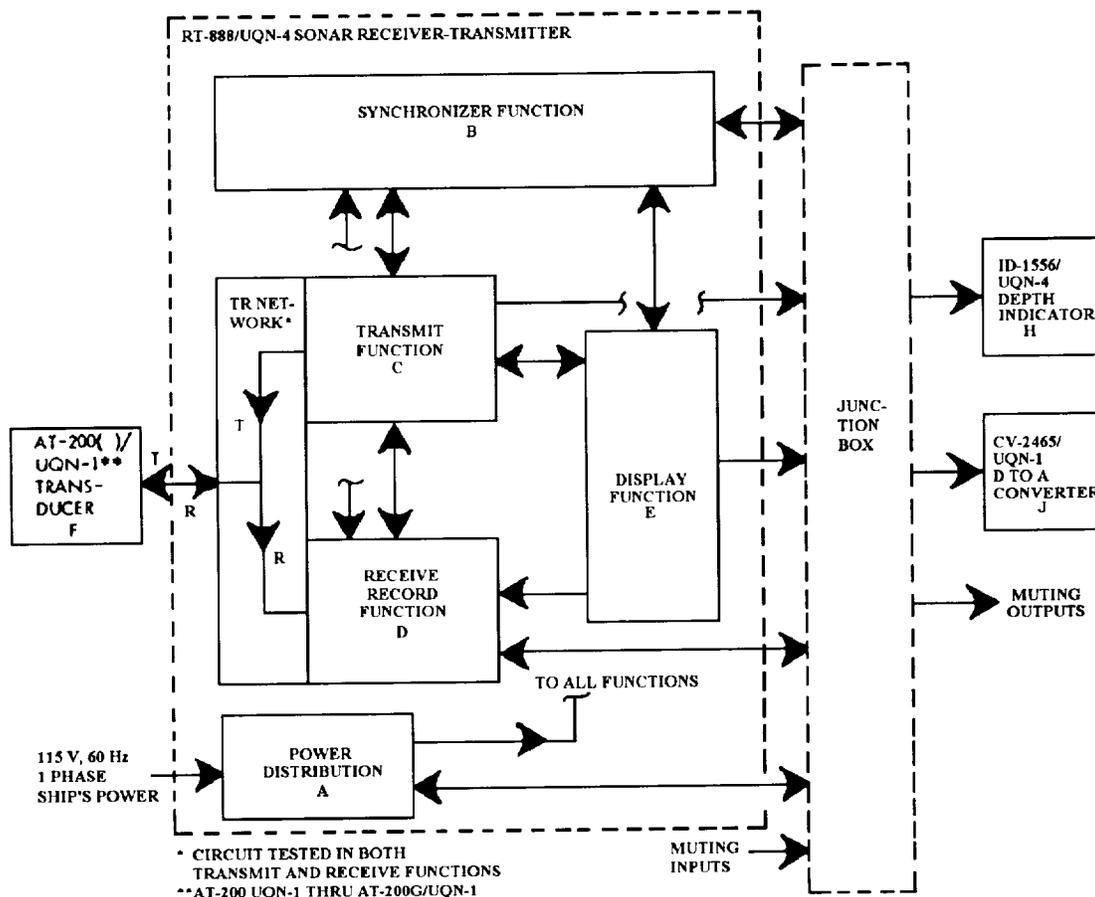
Figure 1-15.—AN/UQN-4A functional diagram.
