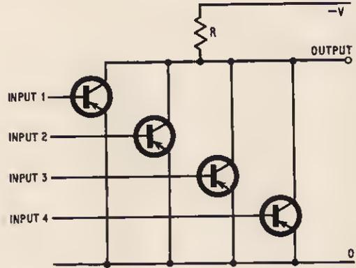
Fig. 11.4a. Basic circuit of a transistor NOR gate
