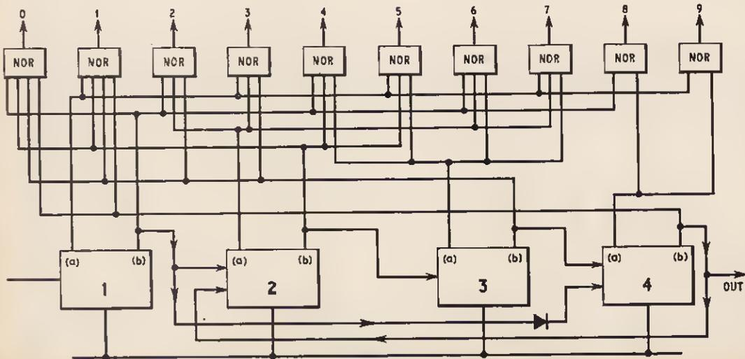
Fig. 11.4b. Complete decimal unit and NOR gate decoder
