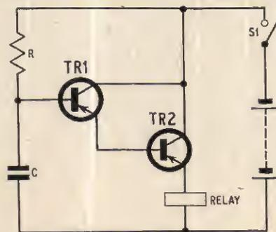
Fig. 7.1a. Darlington pair used to operate a relay
