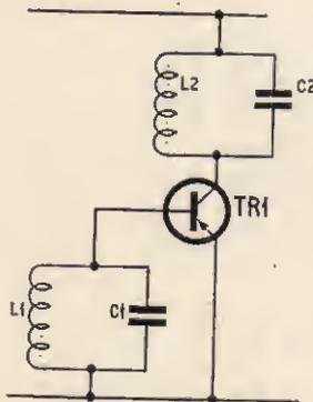
Fig. 7.8a. Basic tuned collector, tuned base oscillator
