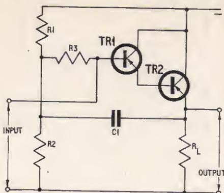
Fig. 7.2b. "Bootstrap" circuit using a Darlington pair
