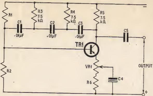
Fig. 7.5. Phase shift oscillator tuned to 1,000 c/s
