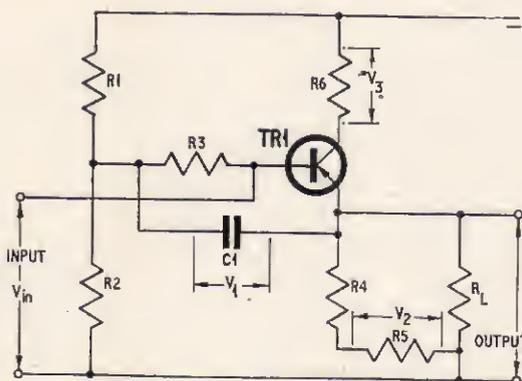
Fig. 7.3 (right). Basic "bootstrap" circuit
