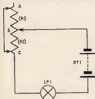
Fig. 2.1. The shunting wire is connected across the resistance element and sections R1 and R2 are thus in parallel
