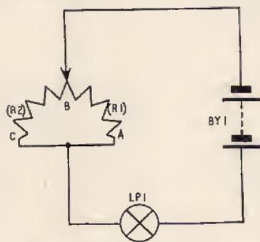
Fig. 2.2. This is the same set-up as Fig. 2.1 but the diagram has been redrawn to show more clearly the fact that R1 and R2 are in parallel
