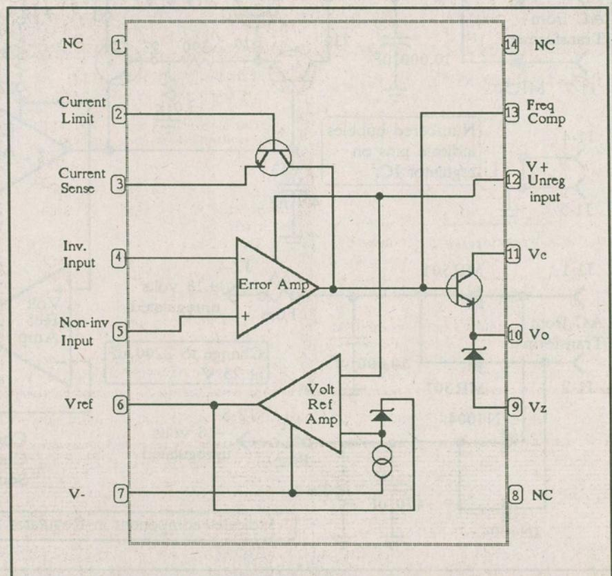
Figure 3. The 723 Voltage Regulator
