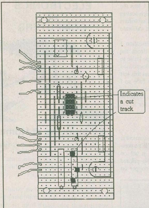
Figure 8. Rear View of Board Indicating Cut Tracks
