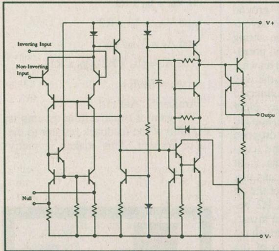
Fig. 2A. Internal Schematic of a 741 Op Amp
