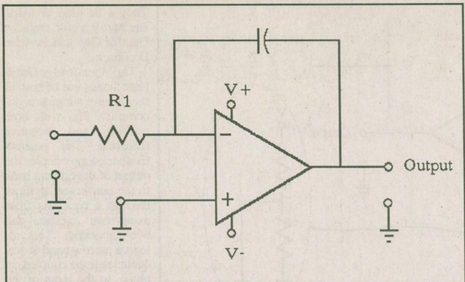
*Fig. 8. An Integrator Configuration*
