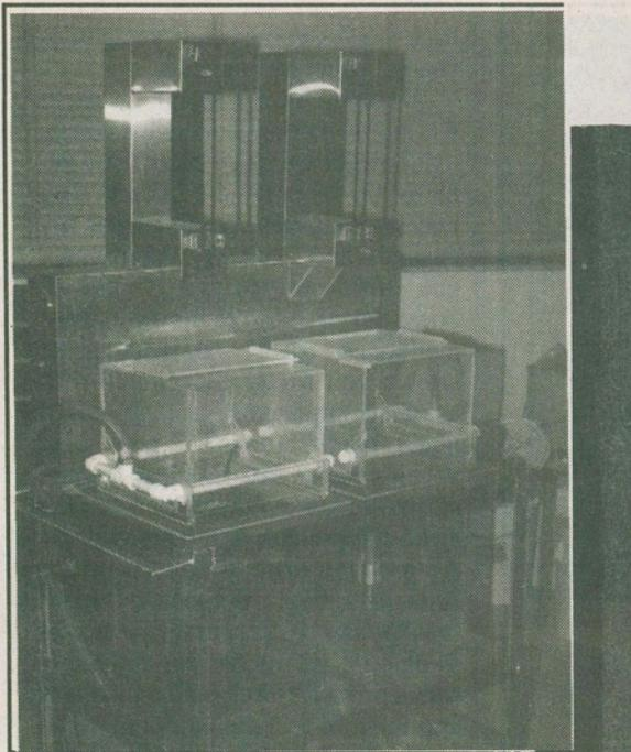
Figure 10. An Etching Tank Using Ammonium Persulfate.
