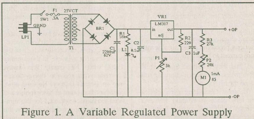
Figure 1. A Variable Regulated Power Supply
