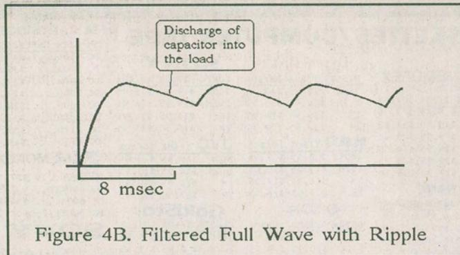
Figure 4B. Filtered Full Wave with Ripple
