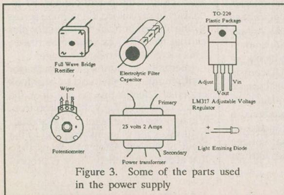
Figure 3. Some of the parts used in the power supply
