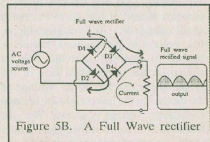
to use the circuit shown in Figure 5B. This is called a full wave or bridge rectifier. Using four diodes in this configuration 'steers' the voltage, whether it is positive or negative from the source, so that it always flows the same
