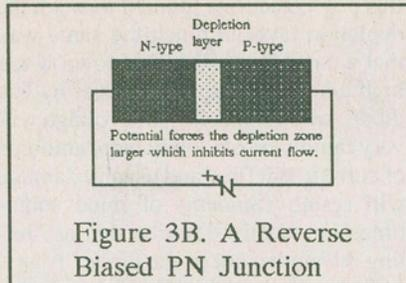
the depletion layer to widen. Positive voltage on the N-type material draws electrons to it widening the depletion layer which is neutral. This stops electrons from flowing through the depletion layer which creates, in effect, a high resistance to current flow. So, when the PN junction is reverse biased it acts like a high resistance and effectively blocks current flow.
