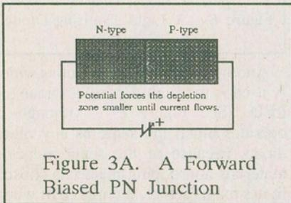
connected to the N-type material. The negative potential on the N-type material causes the extra electrons in the material to be pushed toward the junction while the holes are being pushed toward the junction by the positive side of the voltage source. As the voltage is increased, eventually the electrons will gain enough energy to break through the depletion layer and recombine with holes in the P-type material. When that happens conduction will occur.
