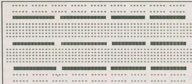
Figure 2. A solderless breadboard
