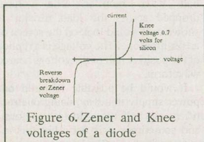
Figure 6. Zener and Knee voltages of a diode
