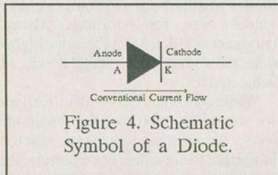
We call this a diode. It conducts in one direction but blocks current flow in the other. Figure 4 shows the standard symbol for a diode with anode (P-type material) and cathode (N-type material) labelled. The anode symbolizes an arrow in the direction of current flow while the cathode symbolizes a blockage of current flow from the other direction.
