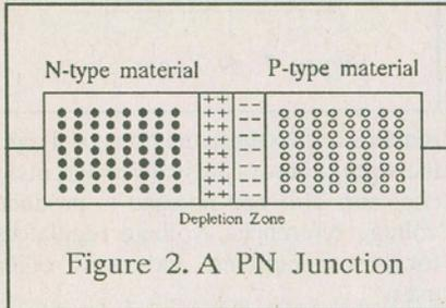
(See Figure 2) Next we apply a voltage. Figure 3A shows a PN junction with a variable voltage source connected across it. When the voltage is connected as in Figure 3A positive voltage is applied to the P-type material while the negative side of the voltage source is
