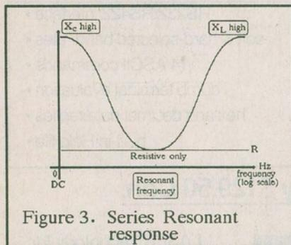
Figure 3. Series Resonant response
