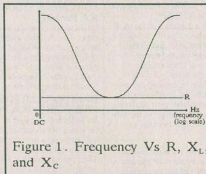
Figure 1. Frequency Vs R,  $X_L$ , and  $X_C$
