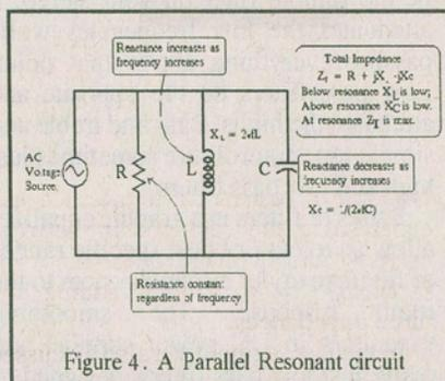
Figure 4. A Parallel Resonant circuit
