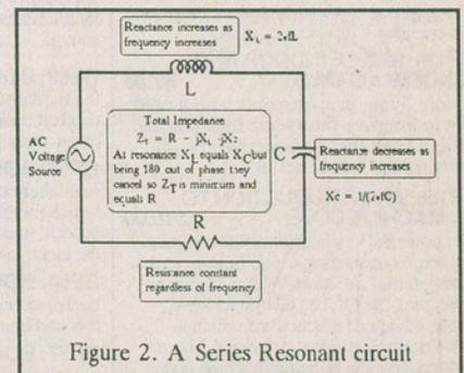
Figure 2. A Series Resonant circuit
