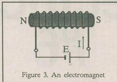
That's what we have done in Figure 3. Not only have we used several turns of current carrying wire (supplied by the battery), but we have added a "core". The core is a ferrous material which concentrates the lines of flux. This increases what we call the "flux density" because there are more lines of flux in a smaller space. Up to a certain point increasing the flux density increases the "field strength" of the electromagnet, in other words making it a stronger magnet.
