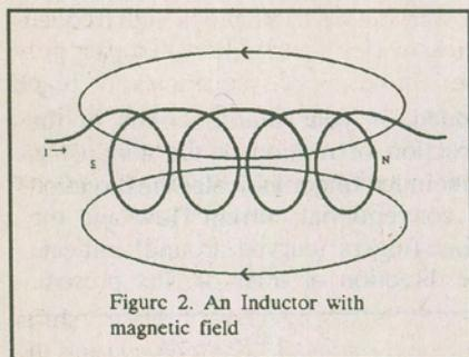
Figure 2. An Inductor with magnetic field
