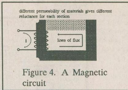
Figure 4. A Magnetic circuit
