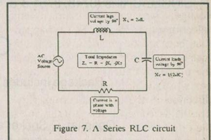
Figure 7. A Series RLC circuit
