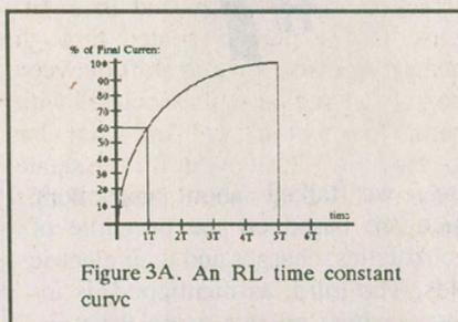
Figure 3A. An RL time constant curve
