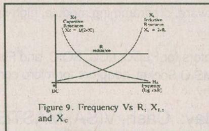
Figure 9. Frequency Vs R, X<sub>L</sub>, and X<sub>C</sub>
