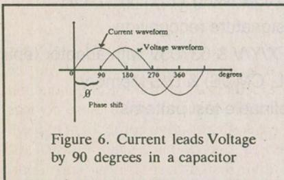
Figure 6. Current leads Voltage by 90 degrees in a capacitor
