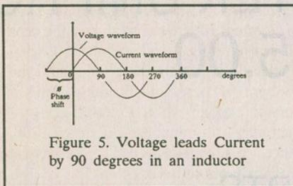
Figure 5. Voltage leads Current by 90 degrees in an inductor
