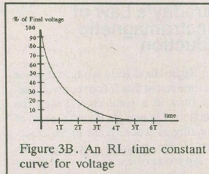
Figure 3B. An RL time constant curve for voltage
