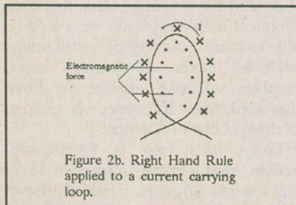
Figure 2b shows a loop of wire with current flowing through it. If we use the Right Hand Rule to determine the direction of the lines of flux and try to visualize it in three dimensions we will find
