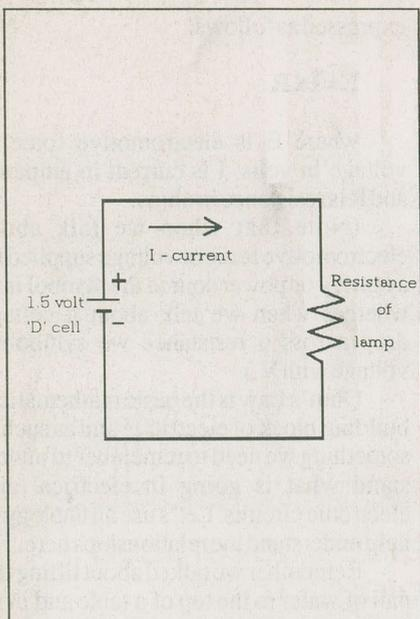
Fig. 5. A simple electrical circuit.
