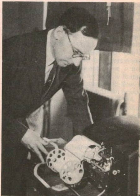
EDSAC, one of the first electronic digital computers, built at Cambridge University in 1949. The shot at right shows Dr. M. V. Wilkes, leader of the team which produced the machine. It used more than 3000 thermionic valves. The name "EDSAC" stood for electronic delay storage automatic calculator.
