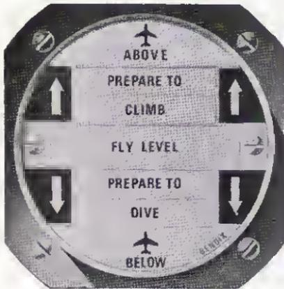
Fig. 1-15. The cockpit indicator of the Bendix collision avoidance system. (Courtesy Bendix Corp., Avionics Division)
