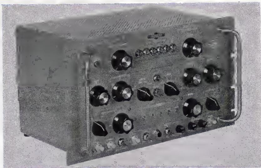
Fig. 9-18. The Collins 578X-1 ATC transponder bench test set.
