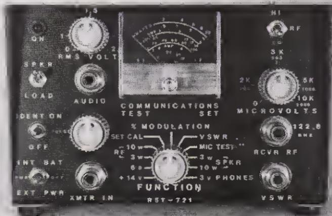
Fig. 15-3. The Radio Systems Technology Model RST-721 Communications Test Set. (Courtesy Radio Systems Technology)
