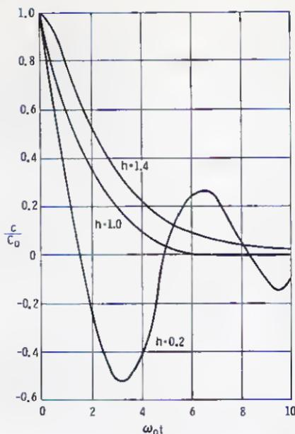
Fig. 11-20. Graph shows oscillation, critical damping, and over-damping.
