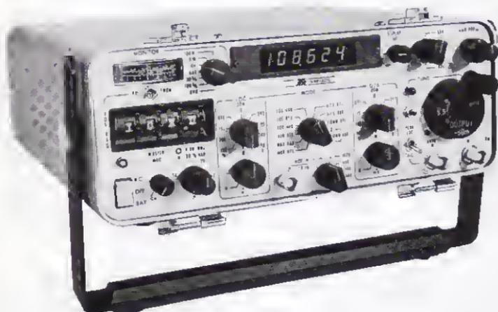
Fig. 6-20. The IFR, Inc., NAV-401L Marker/Nav/Comm Test Set.
