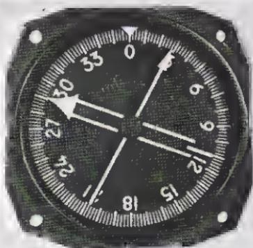
Fig. 7-16. Radio magnetic indicator provides complete heading information on a single instrument (see text). (Courtesy Collins Div., Rockwell International)
