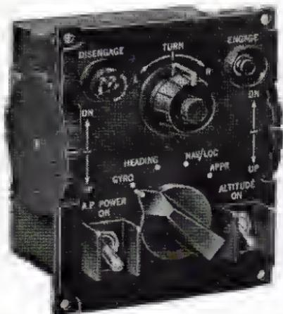
Fig. 13-11. Control head of the Collins AP-103 autopilot. (Courtesy Collins Div., Rockwell International)
