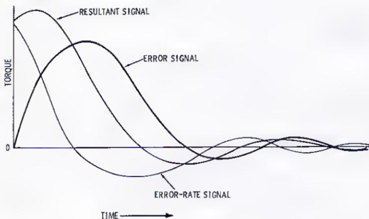
**Fig. 11-19. Error-rate damping.**
