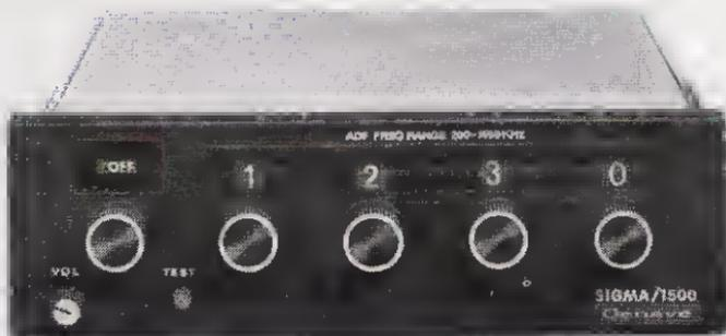
Fig. 7-17. The Genave SIGMA/1500 ADF uses PLL frequency synthesis to cover all 1-kHz increments from 200 kHz to 1699 kHz. (Courtesy General Aviation Electronics, Inc.)
