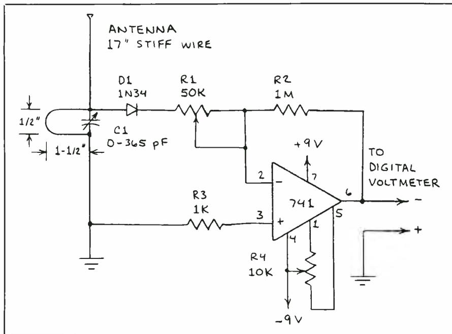
Fig. 5. A radio-frequency field-strength meter.
