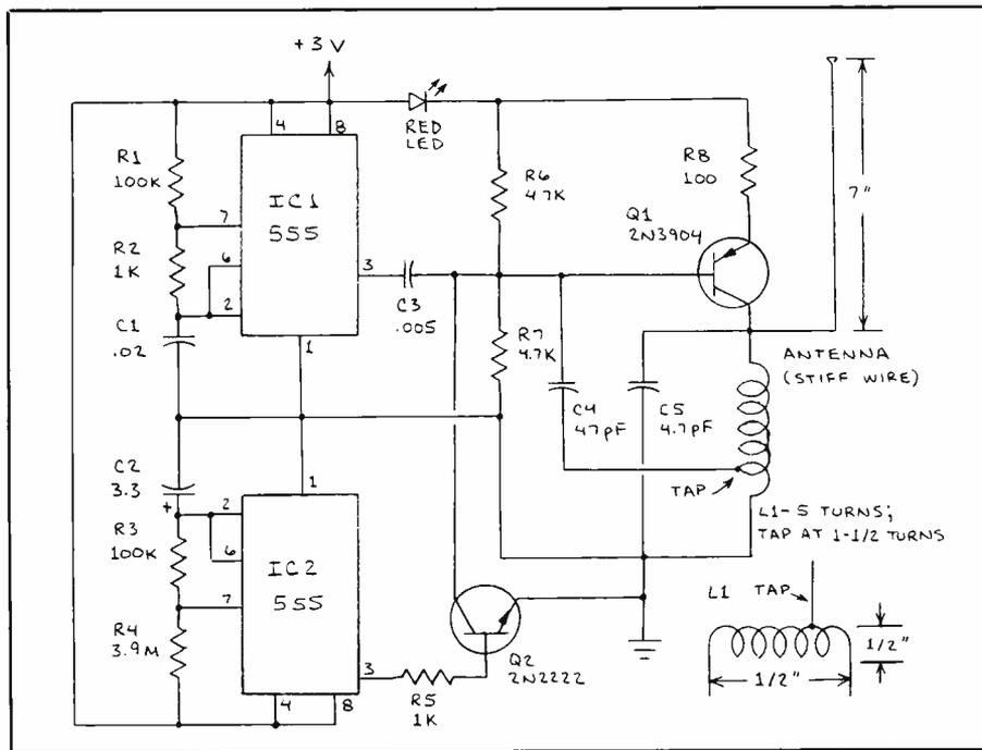
Fig. 3. A low-power vhf pulse transmitter.
