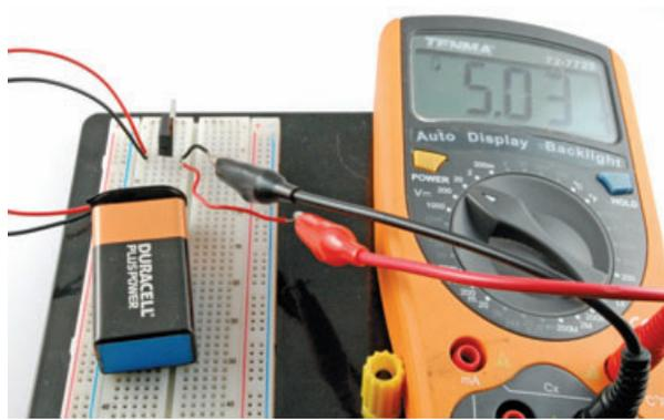
FIGURE 5-7 Experimenting with the 7805
