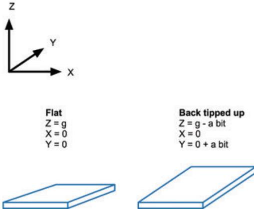
**FIGURE 8-15** The effect of gravity on the accelerometer
