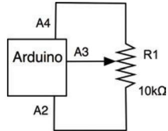
FIGURE 6-17 Schematic diagram—measuring voltage with an Arduino
