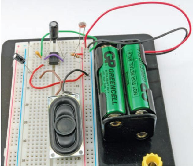
**FIGURE 9-18** Generating tones with a 555 timer IC
