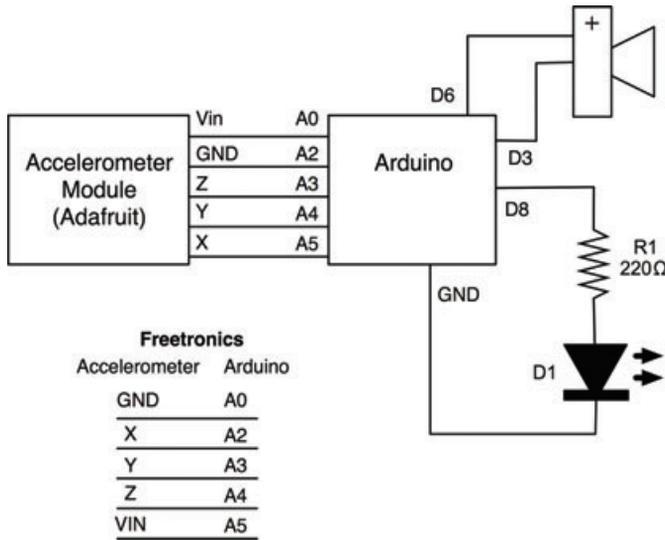
**FIGURE 8-17** The schematic diagram for the Arduino Egg and Spoon
