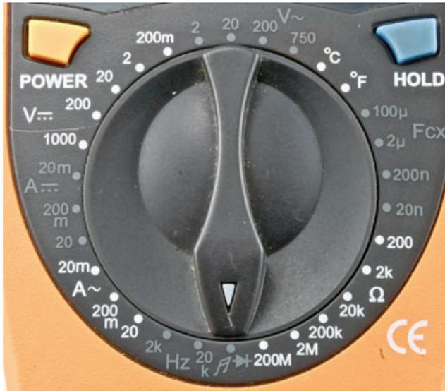
**FIGURE 11-1** Multimeter range selection
