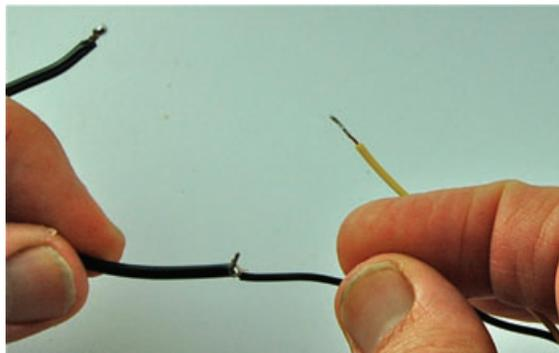
**FIGURE 1-14** Connecting the negative leads together
