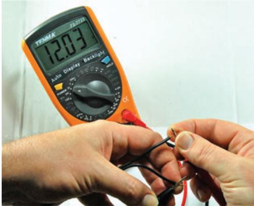
**FIGURE 1-13** Using a multimeter to find the power supply polarity
