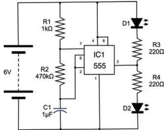
FIGURE 4-18 The LED flasher schematic
