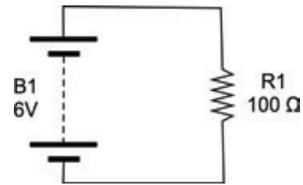
FIGURE 3-1 The schematic for heating a resistor
