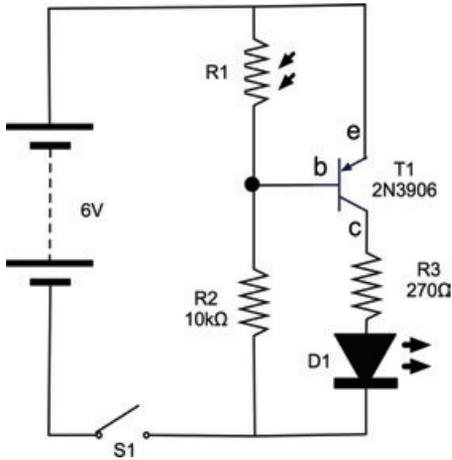
**FIGURE 3-24** Using a PNP bipolar transistor
