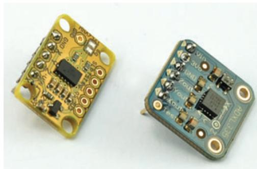
**FIGURE 8-14** Accelerometer modules
