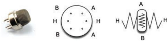
FIGURE 8-1 A methane sensor
