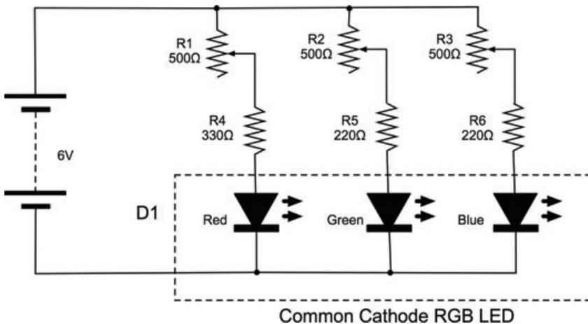
**FIGURE 4-7** An RGB LED test breadboard layout
