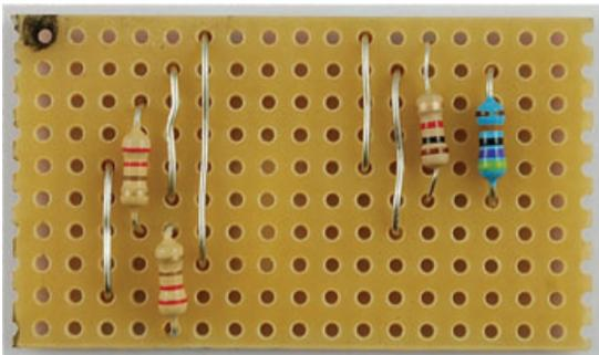
**FIGURE 4-28** The stripboard with resistors in place
