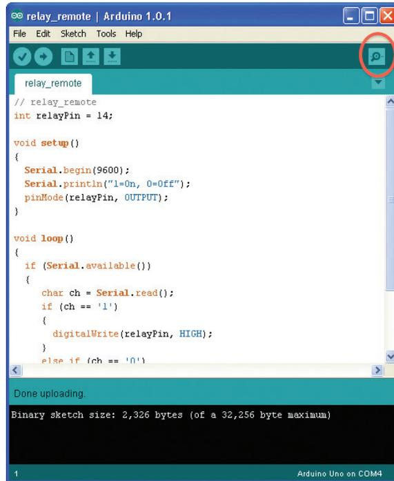
FIGURE 6-14 Opening the Serial Monitor
