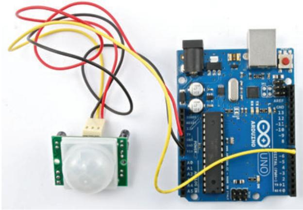
**FIGURE 7-5** The Arduino and the PIR sensor
