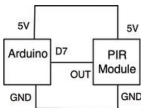
**FIGURE 7-4** Schematic diagram for the Arduino and PIR sensor
