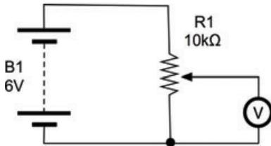
**FIGURE 3-4** A voltage divider schematic diagram
