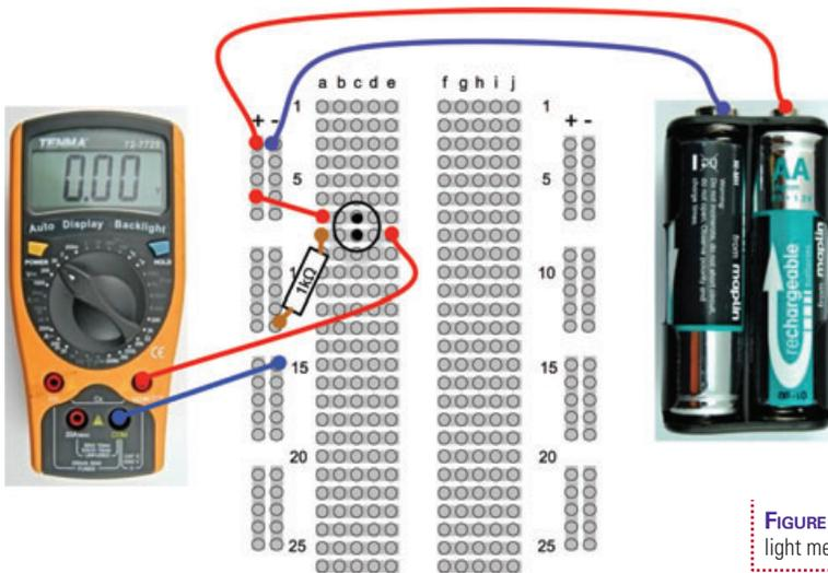
FIGURE 3-10 A breadboard layout for light measurement
