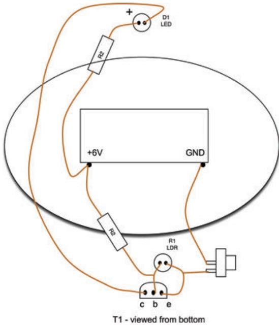
FIGURE 3-22 The push light wiring diagram
