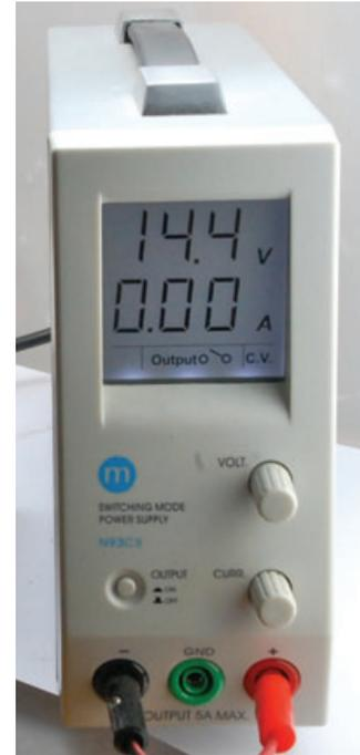
FIGURE 11-7 A lab power supply
