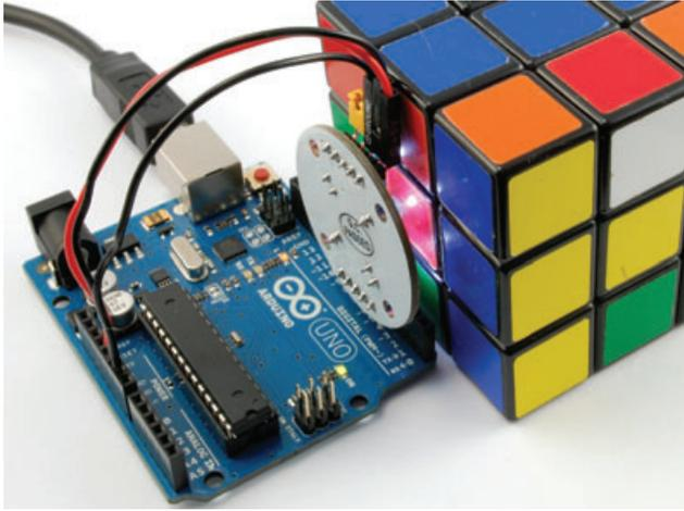
**FIGURE 8-9** Sensing colors on a Rubik's cube
