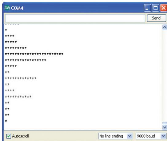
FIGURE 9-23 The Serial Monitor as a VU meter
