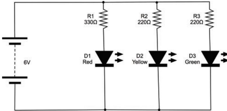
FIGURE 4-4 An LED's schematic
