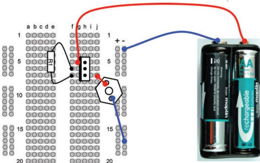
**FIGURE 4-12** The LED constant current driver
