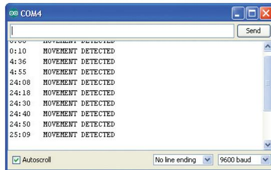
**FIGURE 7-6** The Serial Monitor showing intruder alerts
