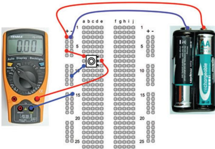
FIGURE 3-5 A voltage divider breadboard layout
