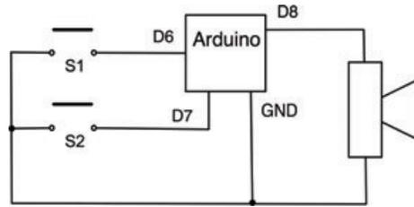
FIGURE 6-23 Schematic diagram for the tone generator
