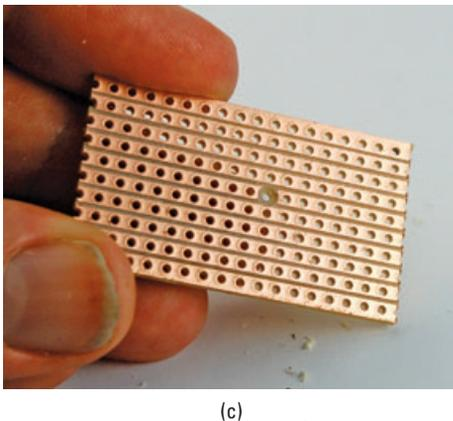
**FIGURE 4-24** Cutting a track on stripboard
