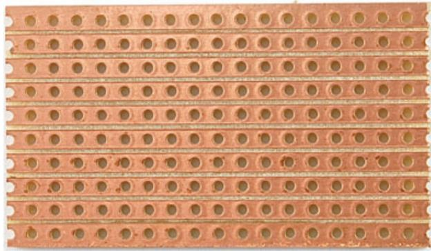
**FIGURE 4-23** A stripboard cut to size
