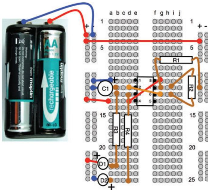
FIGURE 4-19 The LED flasher breadboard layout
