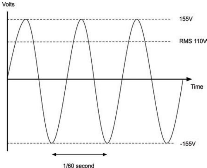
FIGURE 11-4 Alternating current
