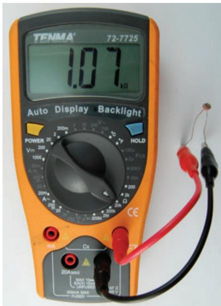
**FIGURE 3-8** Measuring the LDR resistance
