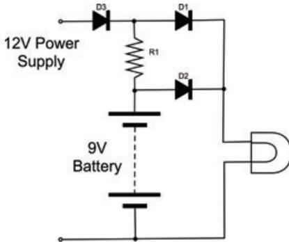
**FIGURE 5-12** Battery backup and charging
