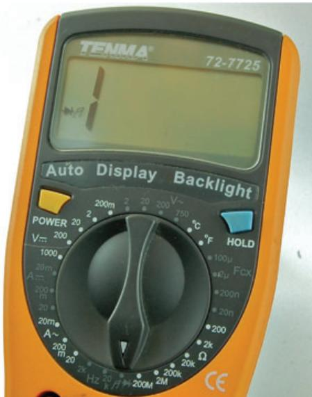
**FIGURE 1-8** A multimeter in Continuity mode
