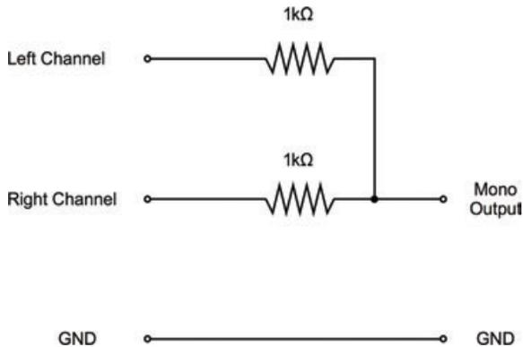
**FIGURE 9-4** Mixing stereo to mono
