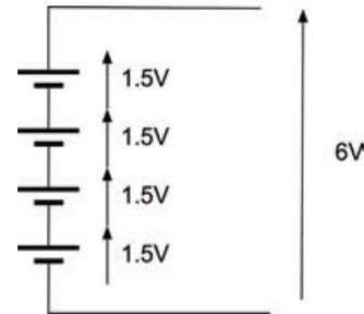
FIGURE 3-2 The schematic diagram for a battery holder
