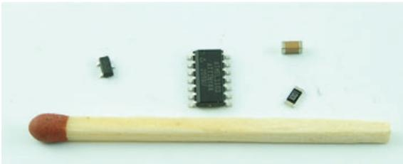
**FIGURE 2-10** Surface mount components
