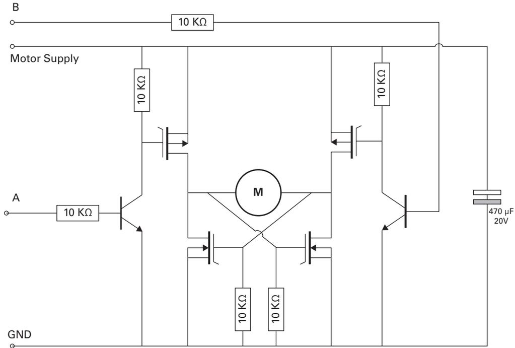
FIGURE 7-21 An example schematic for an H-Bridge
