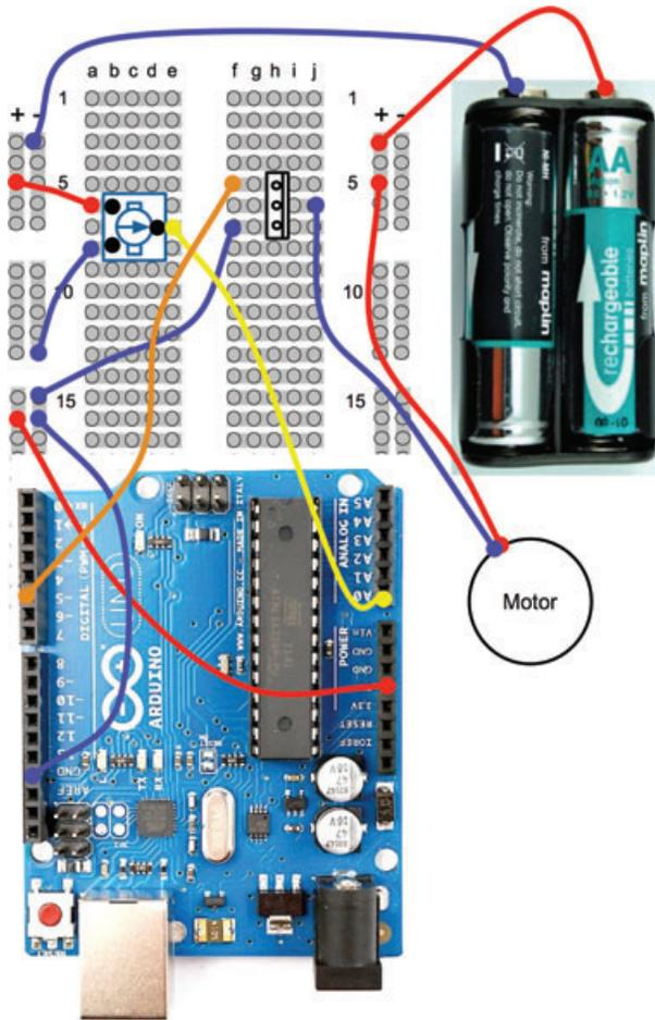
**FIGURE 7-19** Breadboard layout for the MOSFET motor control
