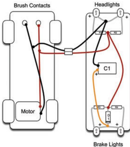
**FIGURE 4-35** The wiring diagram for the modified car
