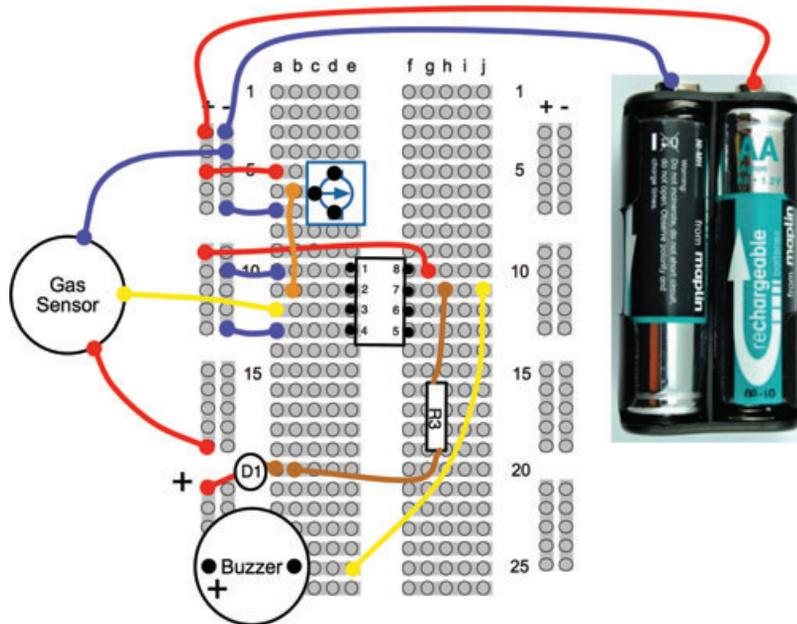
FIGURE 8-4 Breadboard layout for the gas detector
