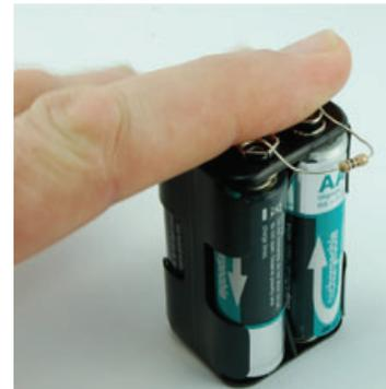
FIGURE 3-3 Making a resistor get hot
