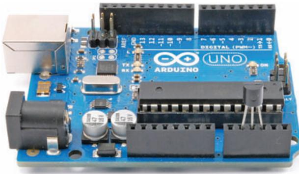
**FIGURE 8-13** The TMP36 attached to an Arduino
