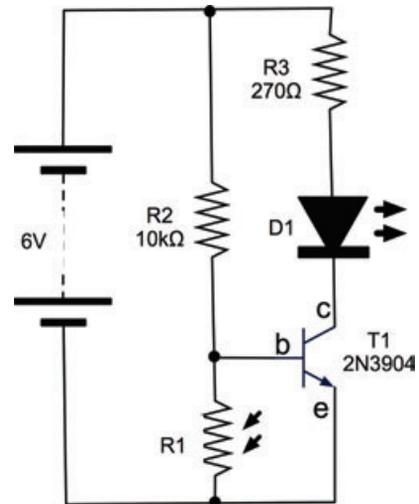
FIGURE 3-14 Using an LDR and transistor to switch an LED
