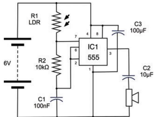
**FIGURE 9-19** Schematic diagram for a 555 tone generator
