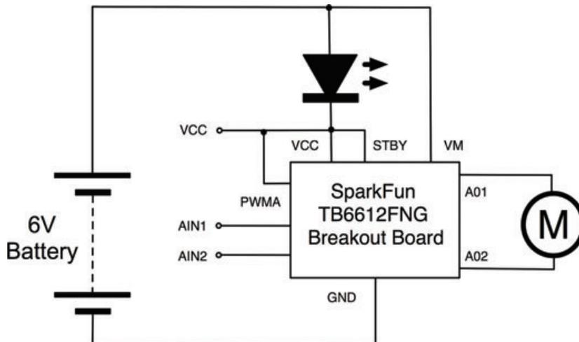
**FIGURE 7-25** Breadboard layout for the H-Bridge experiment
