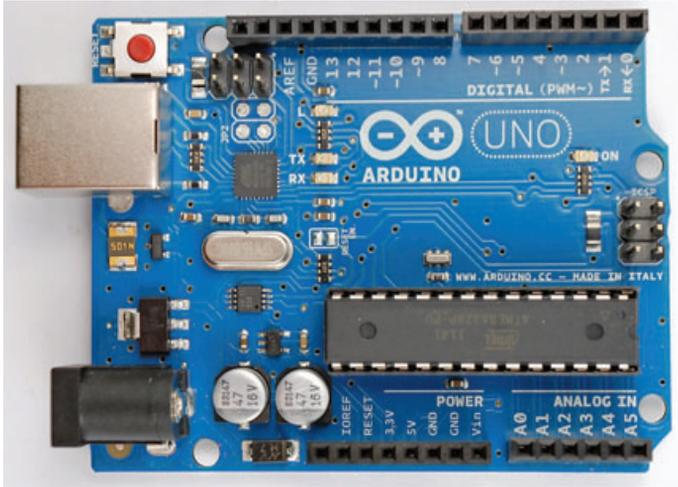
FIGURE 6-1 An Arduino Uno board
