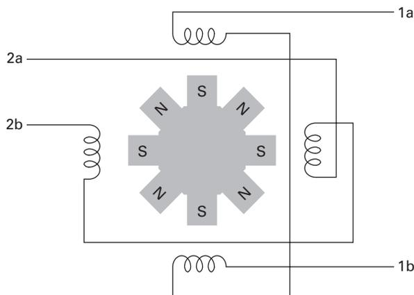
**FIGURE 7-26** How a bipolar stepper motor works
