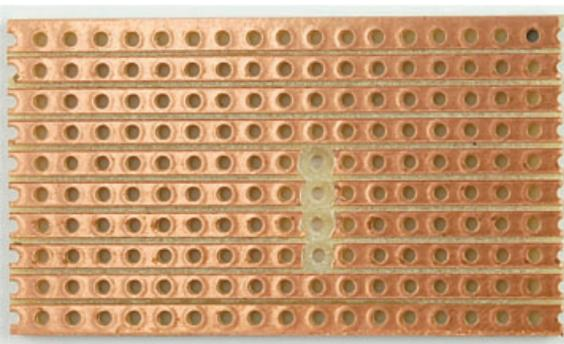
**FIGURE 4-25** The stripboard with breaks cut
