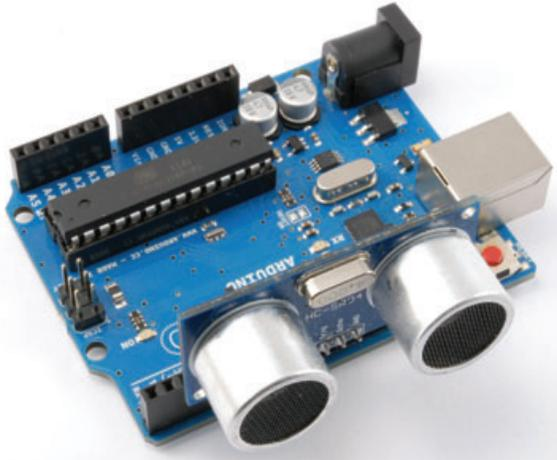
**FIGURE 7-9** An HC-SR04 rangefinder on an Arduino
