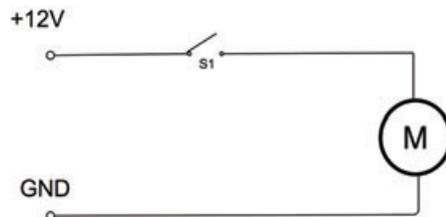
**FIGURE 1-11** The schematic diagram for the fume extractor
