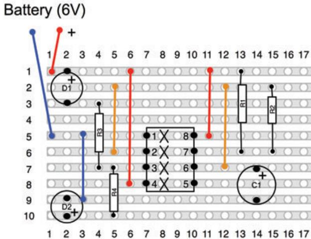
FIGURE 3-22 An LED flasher stripboard layout
