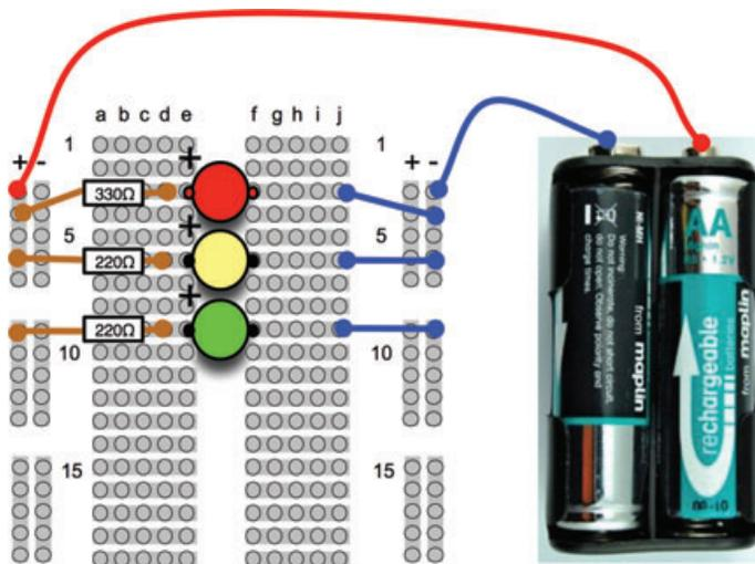
FIGURE 4-5 An LED breadboard layout
