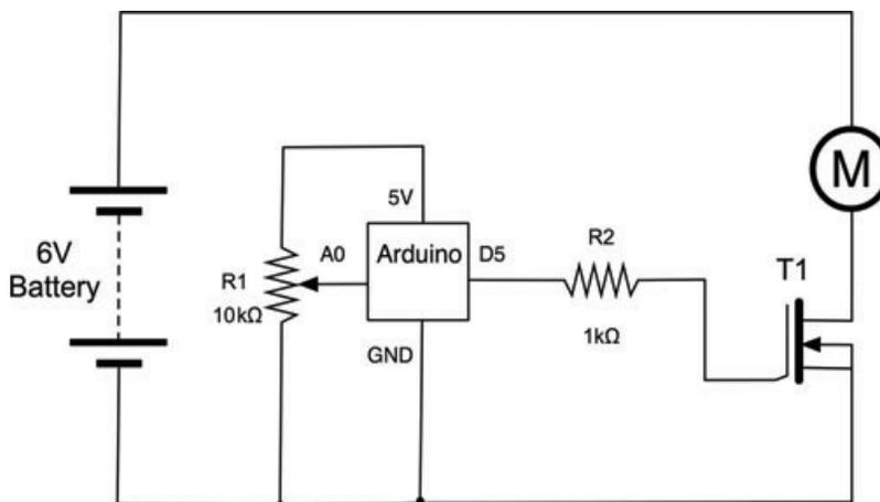
**FIGURE 7-18** The MOSFET motor control
