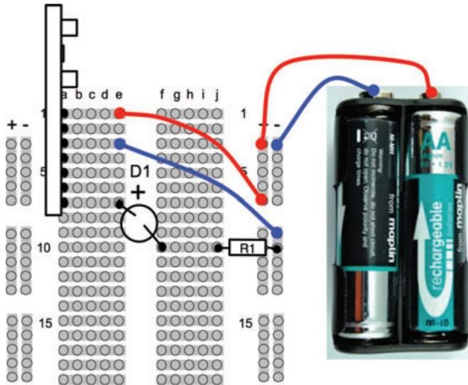
**FIGURE 7-14** Breadboard layout for testing the RF module
