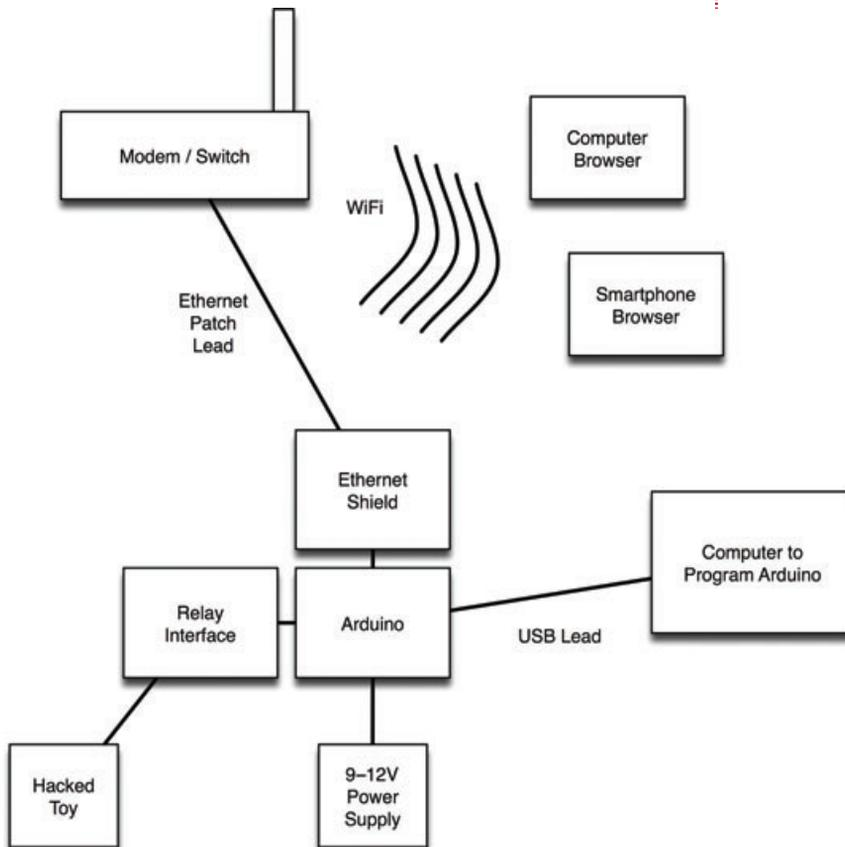
**FIGURE 6-26** Wiring diagram for remote relay control
