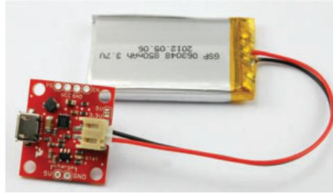
**FIGURE 5-9** Combined LiPo charger and booster
