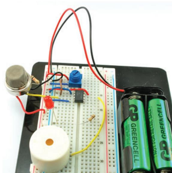
FIGURE 8-5 The gas detector
