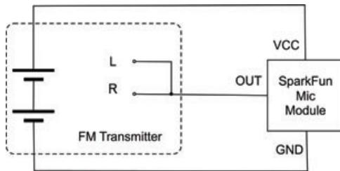
**FIGURE 9-10** Schematic diagram for the radio bug
