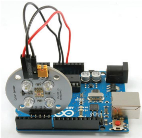
**FIGURE 8-8** A light sensor attached to an Arduino
