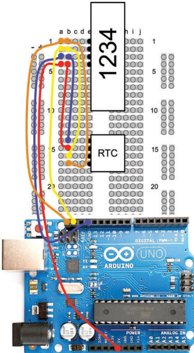
**FIGURE 7-41** Breadboard layout for the clock
