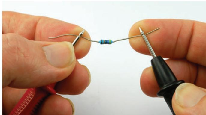
**FIGURE 11-2** How not to measure high-value resistors
