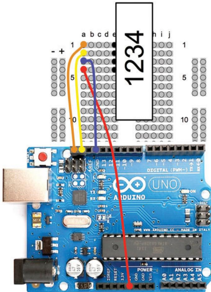
**FIGURE 7-37** Breadboard layout for using the seven-segment display
