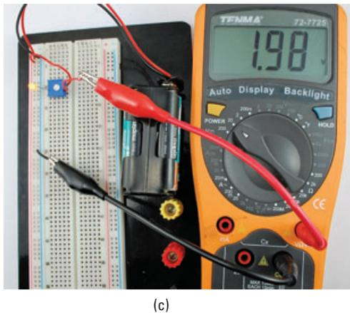
**FIGURE 4-15** Measuring the forward voltage of an LED
