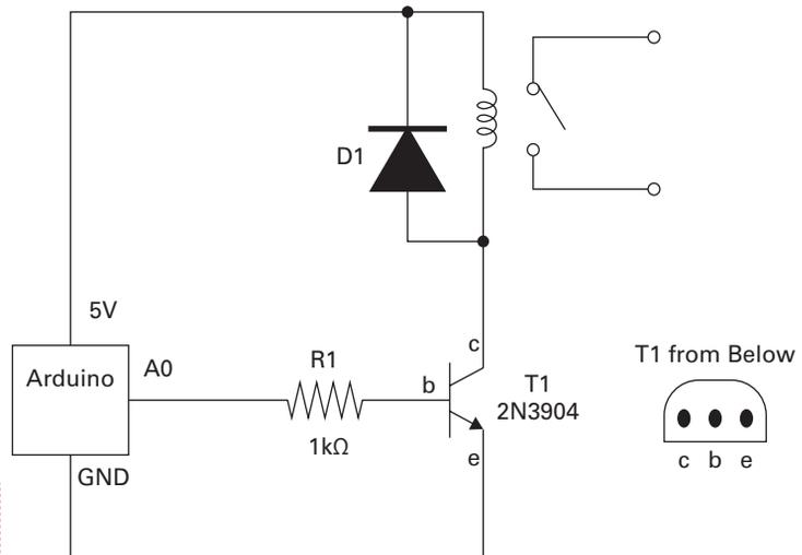
**FIGURE 6-8** Schematic diagram of an Arduino-controlled relay
