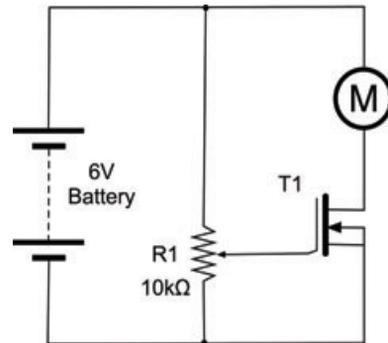
FIGURE 3-26 A schematic for the MOSFET experiment
