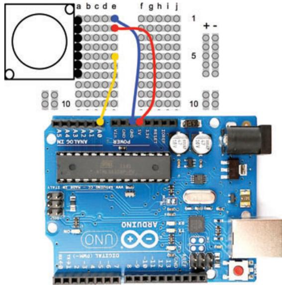
FIGURE 7-12 The MaxBotix rangefinder and Arduino breadboard layout
