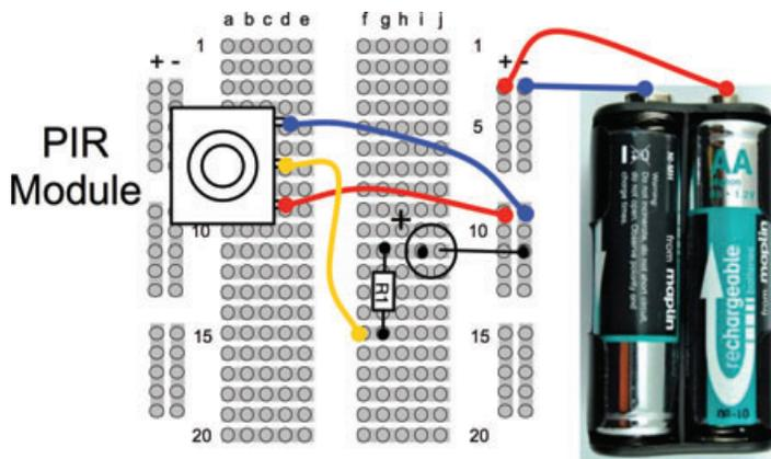
**FIGURE 7-1** Schematic diagram—using a PIR module with an LED
