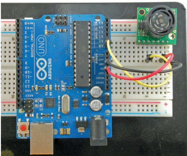
We will use the analog method to test out this device. The figure of  $V_{cc} / 512$  per inch means that the analog output will be the supply voltage divided by 512 per inch. So if the object was 10 inches away, then the analog output voltage would be:
