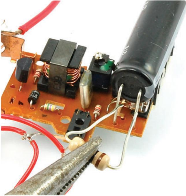
**FIGURE 10-1** Safely discharging a capacitor
