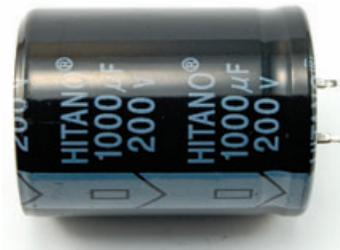
**FIGURE 2-4** An electrolytic capacitor
