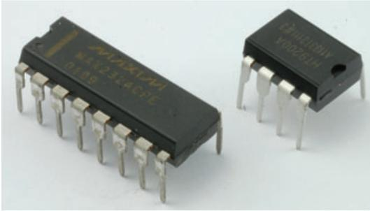
**FIGURE 2-9** Integrated circuits
