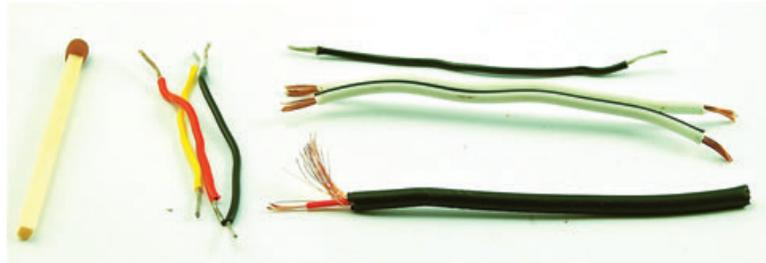
**FIGURE 1-3** Common types of wire
