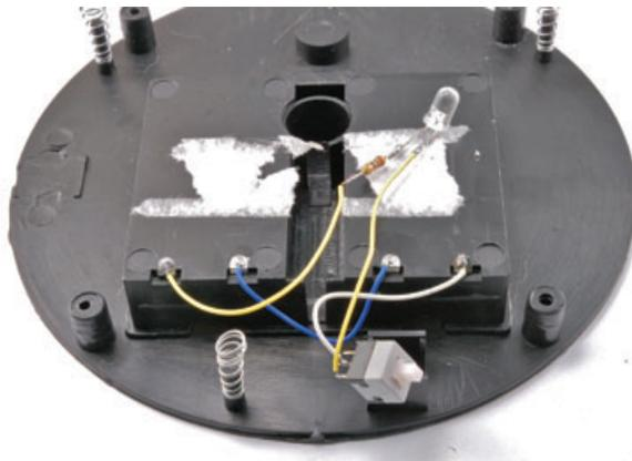
**FIGURE 3-20** Replacing the bulb with an LED and a resistor
