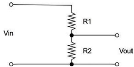
FIGURE 3-7 A voltage divider with fixed resistors
