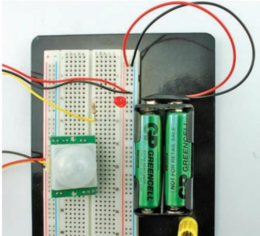
**FIGURE 7-3** Using a PIR module with an LED
