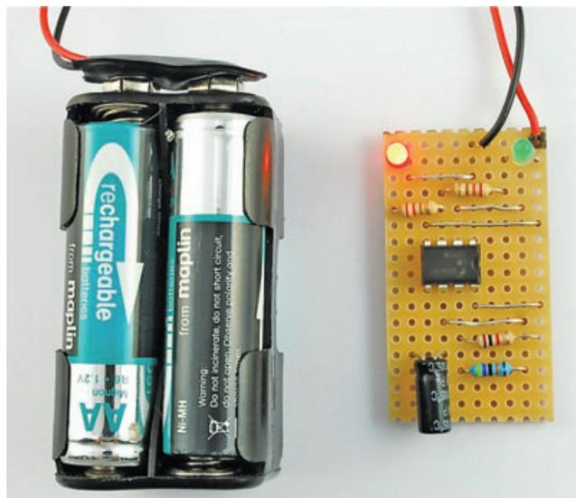
**FIGURE 4-29** The LED flasher on the stripboard
