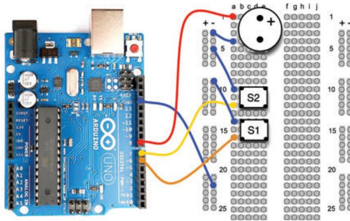
FIGURE 6-24 Breadboard layout for the tone generator
