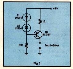
tor load is. In practice, there is a limit to how low you can go, with the load resistance between collector and ground. But this is more to do with the power dissipated by the transistor than the excessive current flow. With the transistor turned fully on, we can assume that there is no voltage drop between the emitter and collector and that we have a maximum voltage of 8.4V at the collector.
