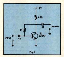
This last factor is often known as 'little r-e' and in our circuit, it is around 25 ohms. multiply that by 100 as a minimum figure for the gain of a BC547 transistor and you get an overall input impedance of around  $2.5k\Omega$ .
