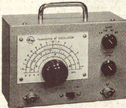
Typical RF signal generators. At top is a commercial unit, while immediately above is one of our more recent designs.
