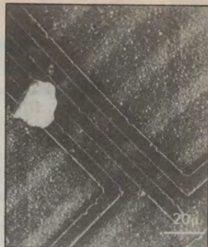
Left: View of part of a circuit on a semiconductor wafer, showing charging effects; "spread" in the darker area is due to charging. Right: A view of the same circuit after charge neutralisation.
