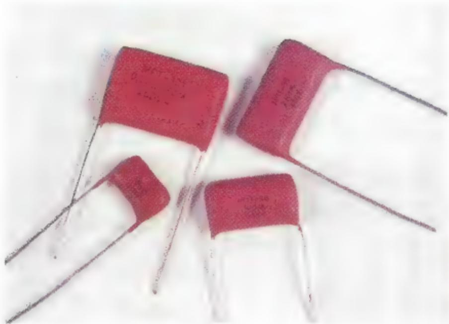
A range of high voltage, metallised polyester film capacitors that are suitable for a wide range of applications including supply decoupling, filter, integrator and audio circuits etc. These low-cost, non-inductive, self-healing capacitors conform to IEC 384-1/384-2.
